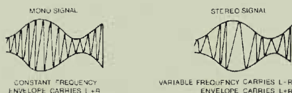
Monophonic and stereophonic modulation of a carrier.
