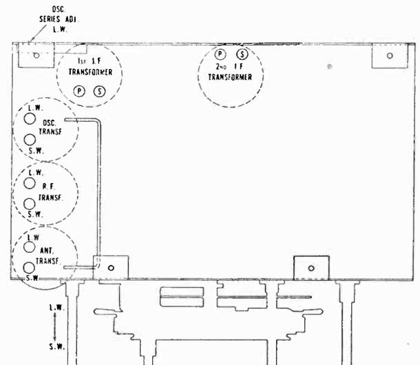
Figure E—Location of Line-Up Capacitors
