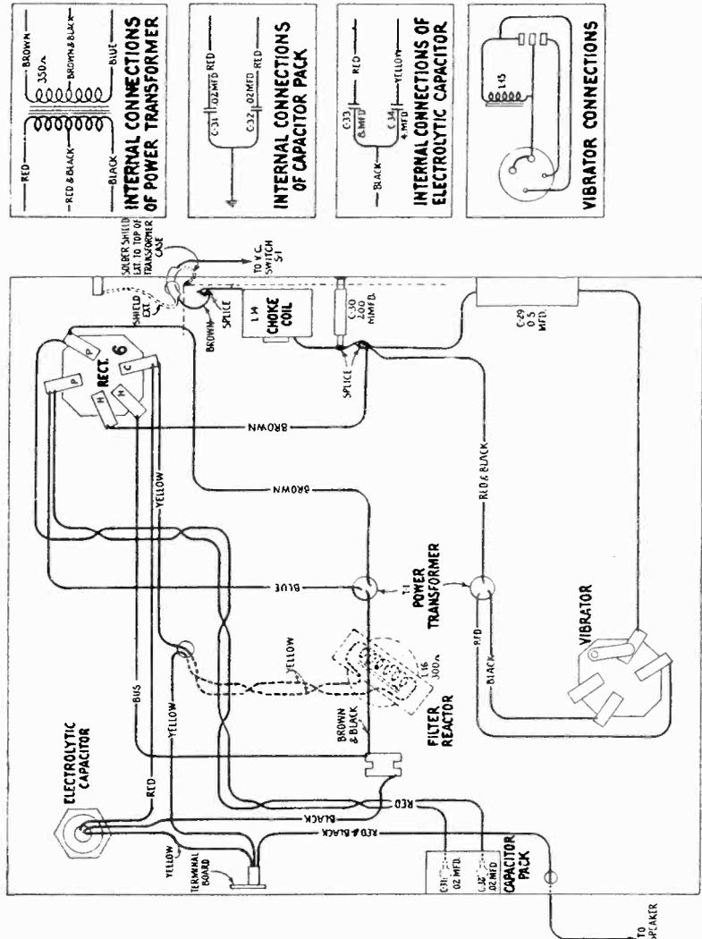
Figure 7—Power Unit Wiring Diagram
