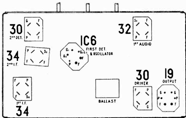
FIG. 3—Tube Socket Layout (View of Underside)
