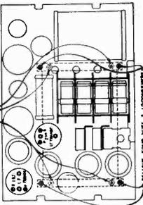
Figure E—Location of nuts and lockwashers to support coil assembly
