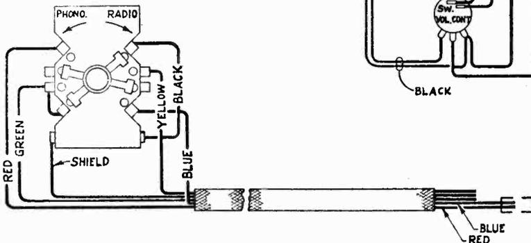
Figure 5—Cable Connections
