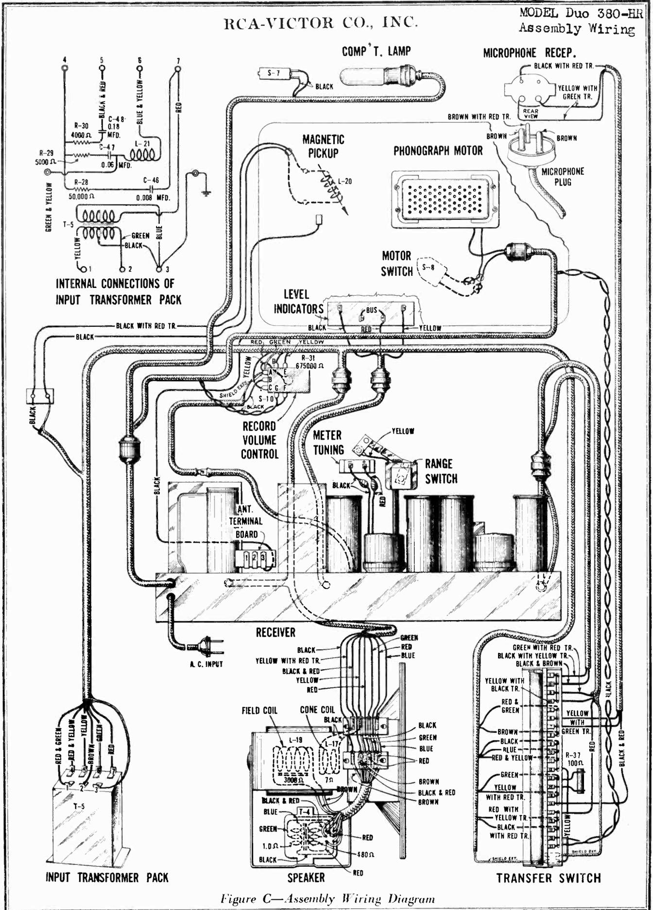
Figure C—Assembly Wiring Diagram
