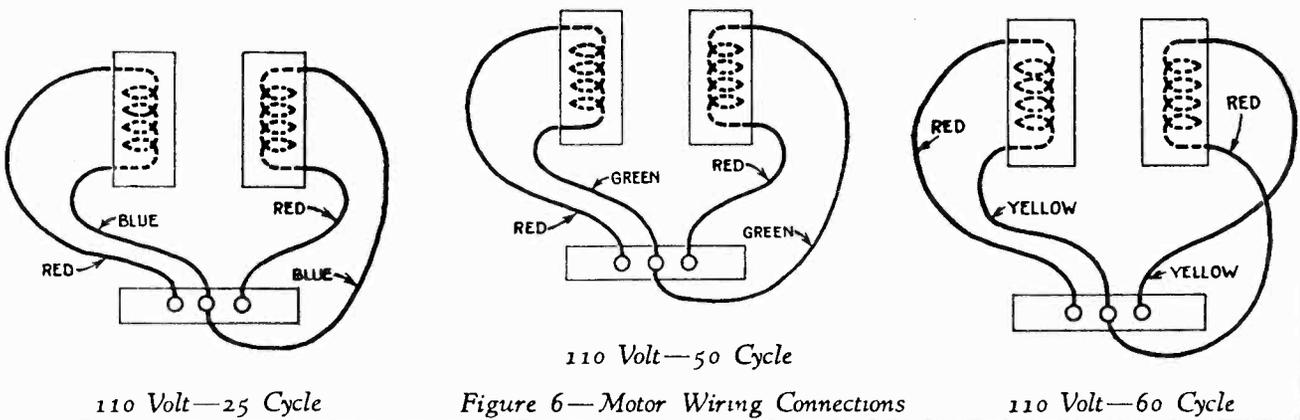
Figure 6—Motor Wiring Connections
