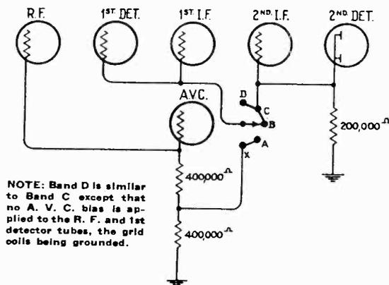
Figure 3—Switching Arrangement of Automatic Volume Control Systems
