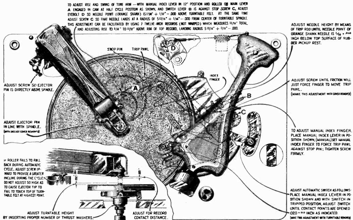
Figure 12—Automatic Record Changer Adjustments
