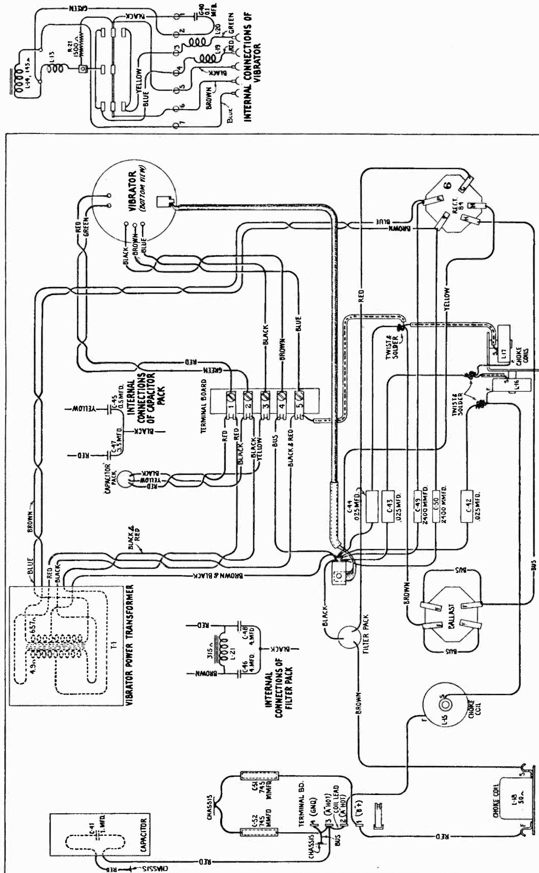
Figure 3—Power Unit Wiring Diagram
