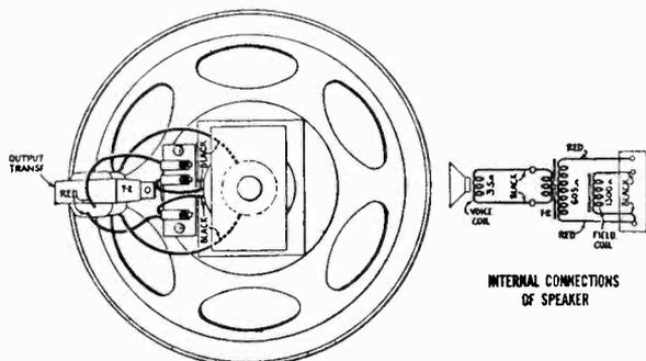
Figure C—Loudspeaker Wiring
