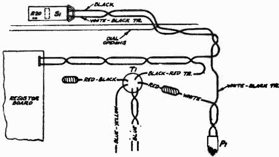
110 V. 25~ CONNECTIONS Figure G—100-115 Volt Connection of 25-60 Cycles Transformer
