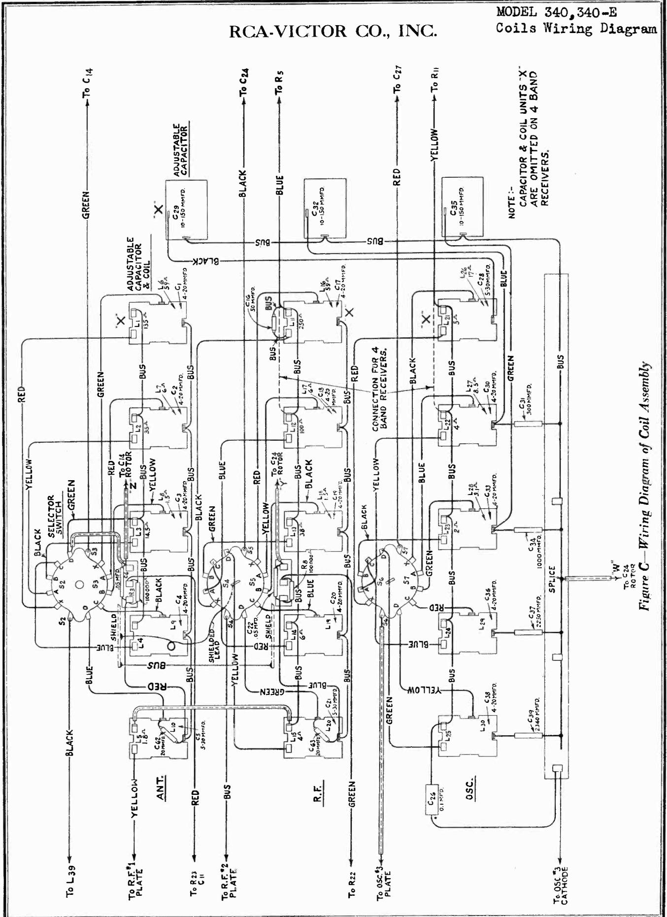
Figure C—Wiring Diagram of Coil Assembly
