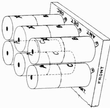
Figure 7—Location of Various Coils in Shields
