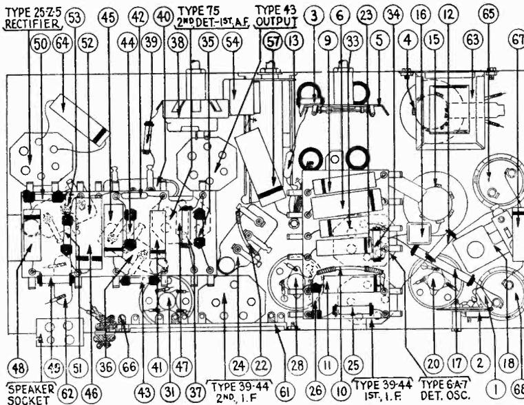
Fig. 4—Bottom View of Chassis Showing Parts.
