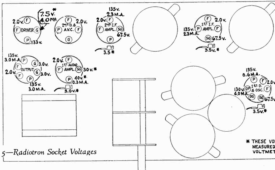
Figure 5—Radiotron Socket Voltages
