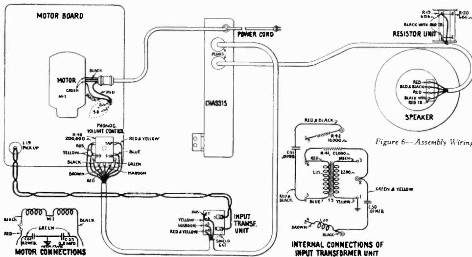
Figure 6—Assembly Wiring Diagram
