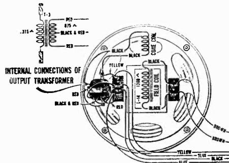
Figure 6—Loudspeaker Wiring
