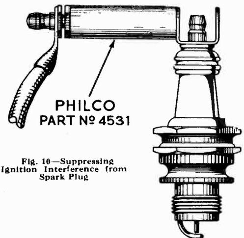
Fig. 10—Suppressing Ignition Interference from Spark Plug
