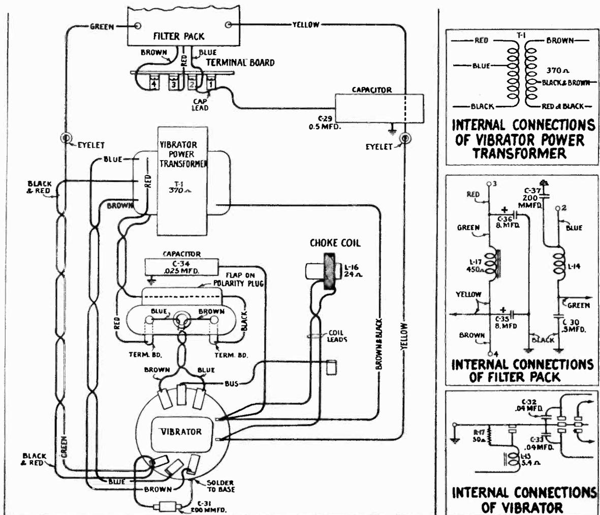
Figure 7—Vibrator Inverter-Rectifier Unit Wiring
