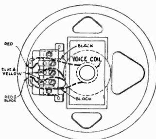
Figure 3—Table Model Loudspeaker Wiring
