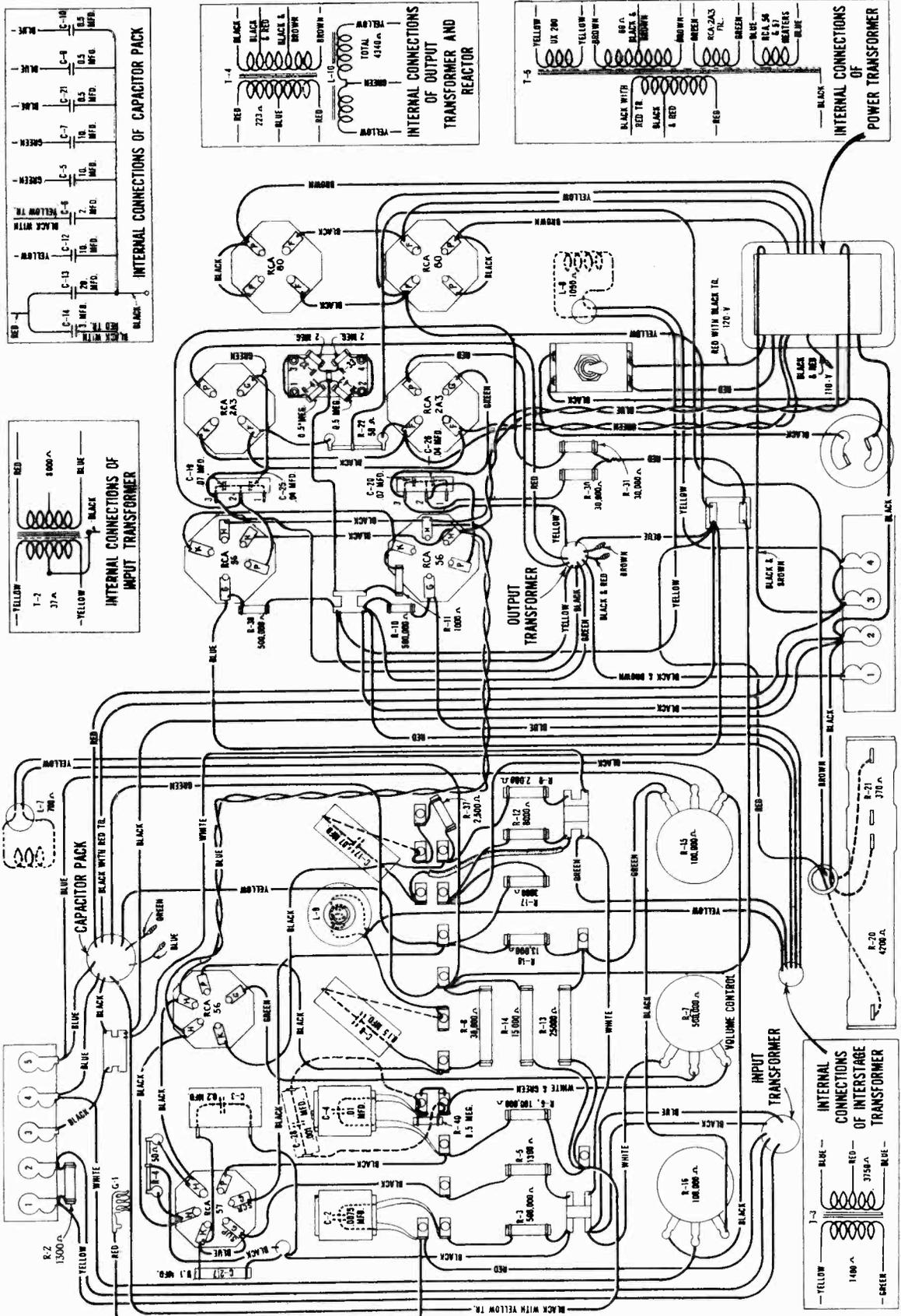
Figure 2—Amplifier Panel Wiring (PB82C1)—Connected for use with 50 inch baffles
