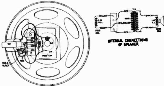
Figure 3—Loudspeaker Wiring
