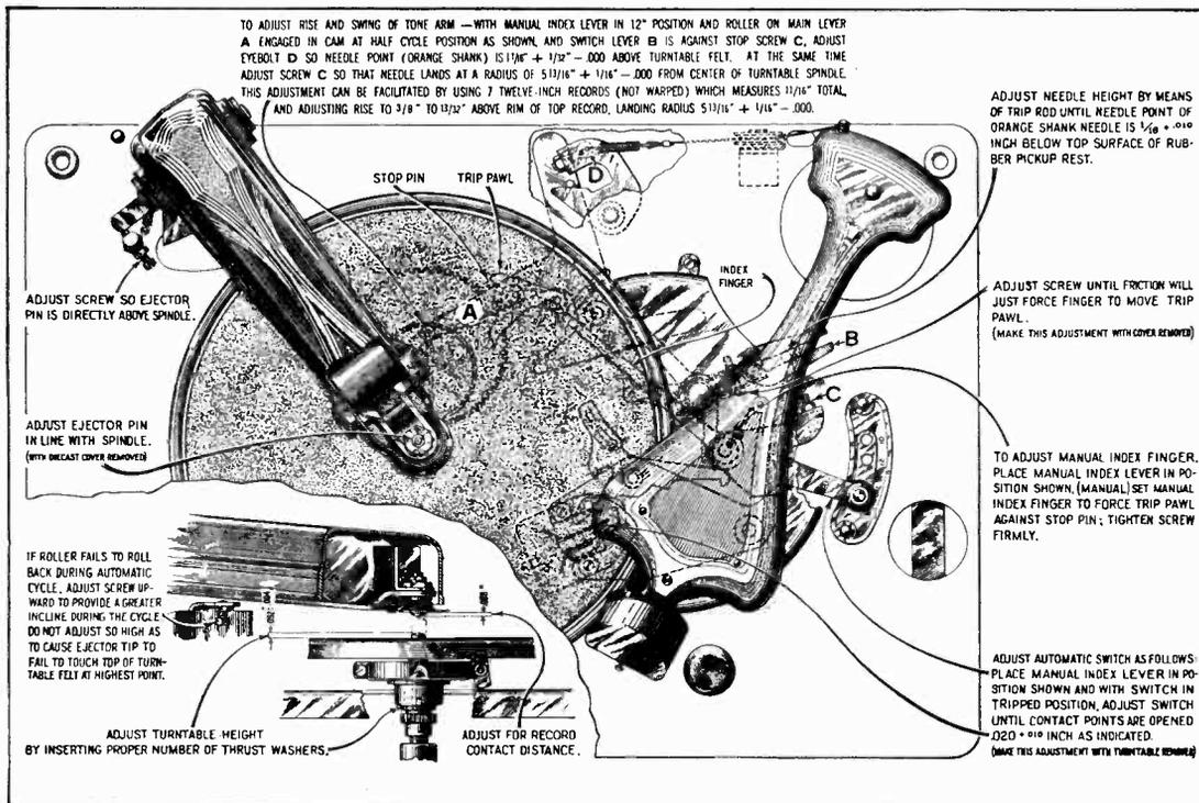
Figure 14—Automatic Record Changer Adjustments
