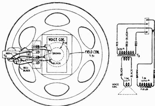
Figure 3—Console Loudspeaker Wiring
