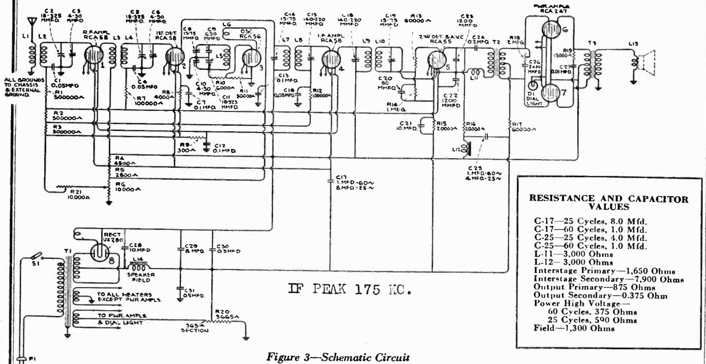
Figure 3—Schematic Circuit
