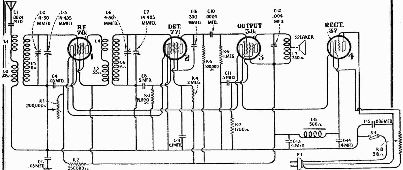
Figure A—Schematic Circuit Diagram
