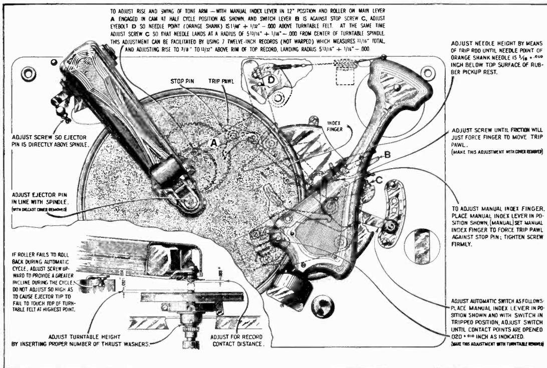
Figure H—Automatic Record Changer Adjustments
