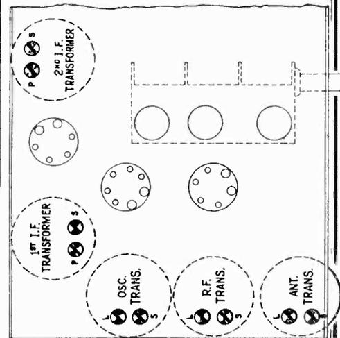
Figure 4—Location of Line-up Capacitors—Viewing bottom of chassis
