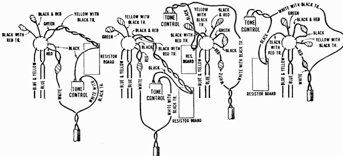
Figure H—Power Transformer Connections (50-60 cycles)
