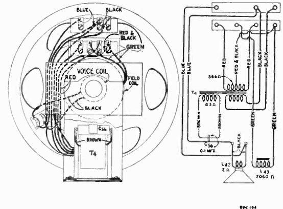
Figure 6—Loudspeaker Wiring
