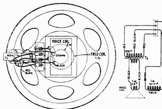
Figure 3—Loudspeaker Wiring
