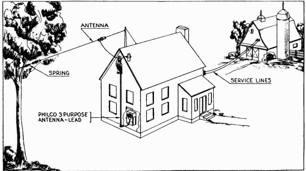
Fig. 8—Best Method of Antenna Installation for Model 32
