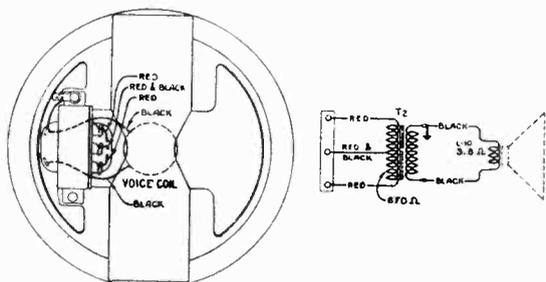
Figure 3—Loudspeaker Wiring
