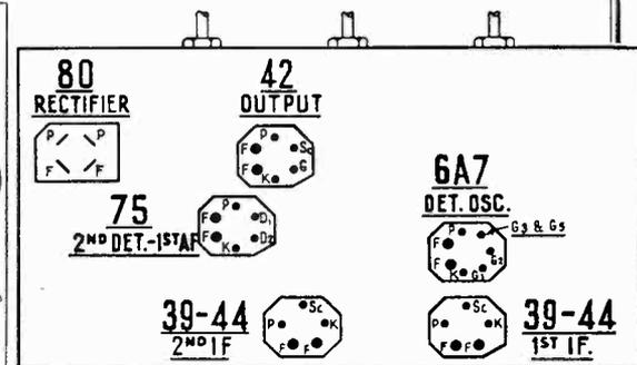
Fig. 1—Tube Socket Layout
