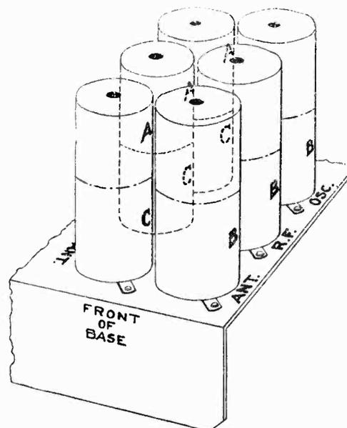
Figure 5—Location of Coils in Shields
