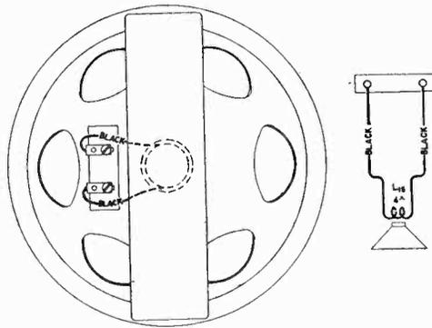
Figure 3—Loudspeaker Wiring
