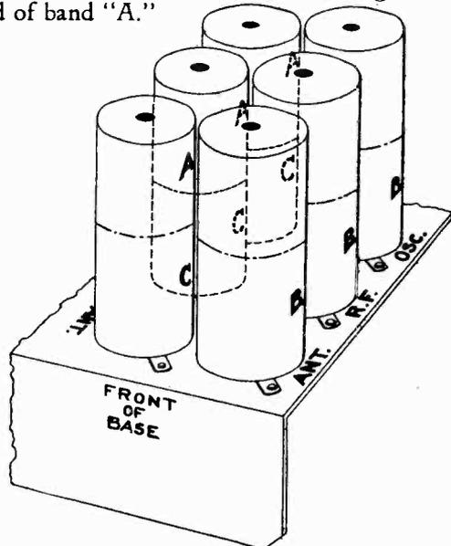
Figure 8—Location of Coils in Shields
