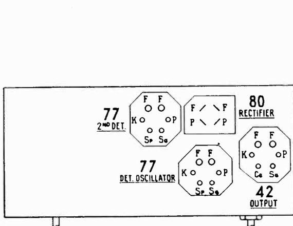
Fig. 1—Tube Socket Layout (Viewed from Bottom)
