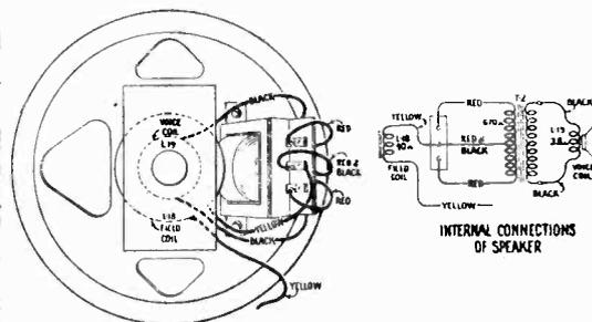
Figure 3—Loudspeaker Wiring
