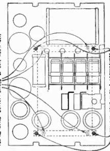
Figure E—Location of nuts and lockwashers holding coil assembly.
