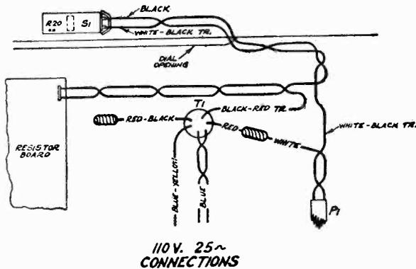
Figure G—100-115 Volt Connection of 25-60 Cycles Transformer
