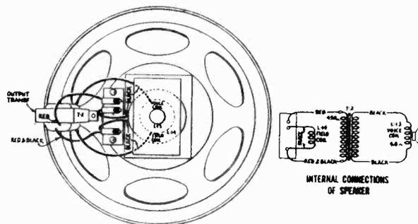
Figure 4—Console Model Loudspeaker Wiring
