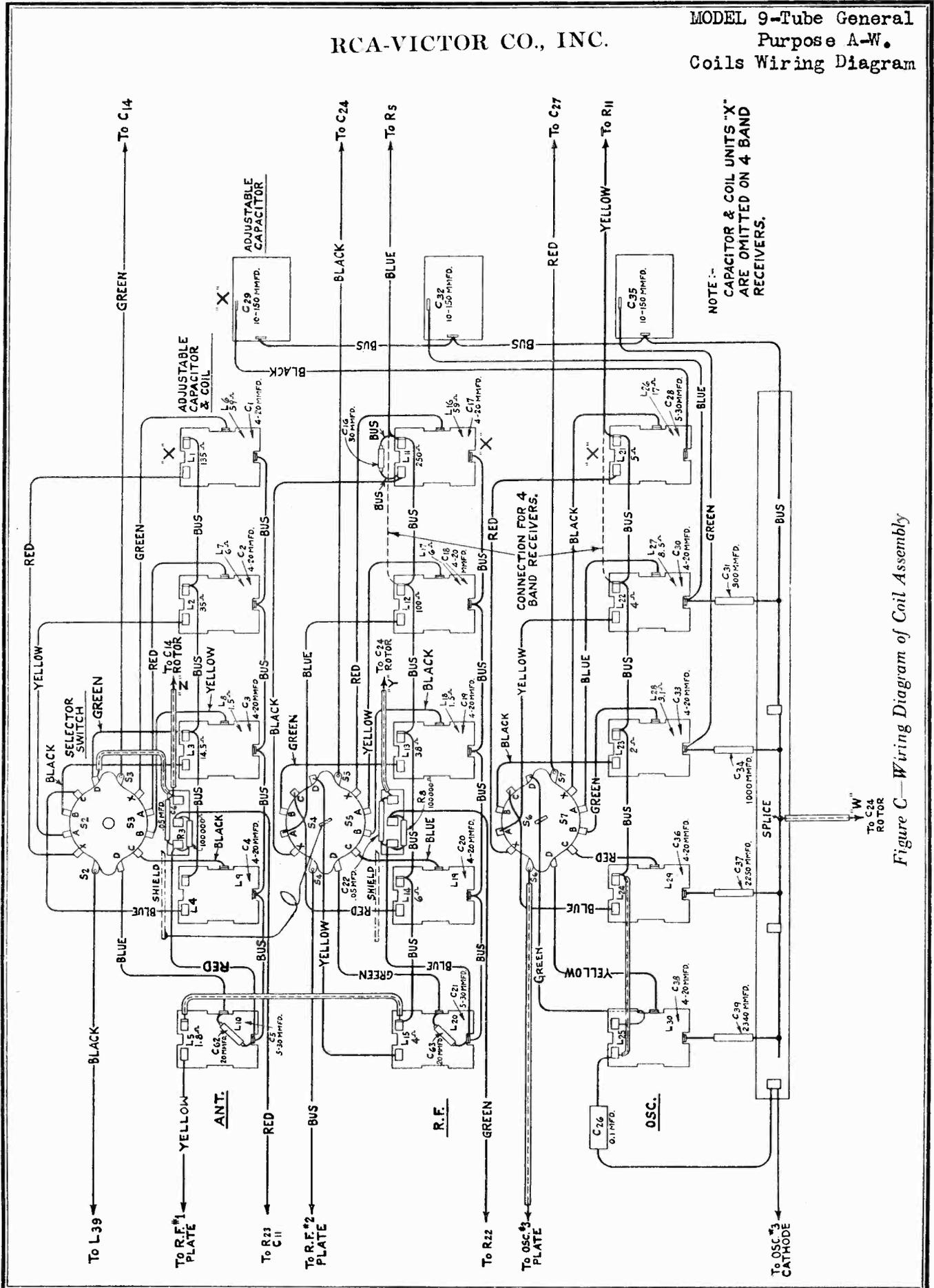
Figure C—Wiring Diagram of Coil Assembly
