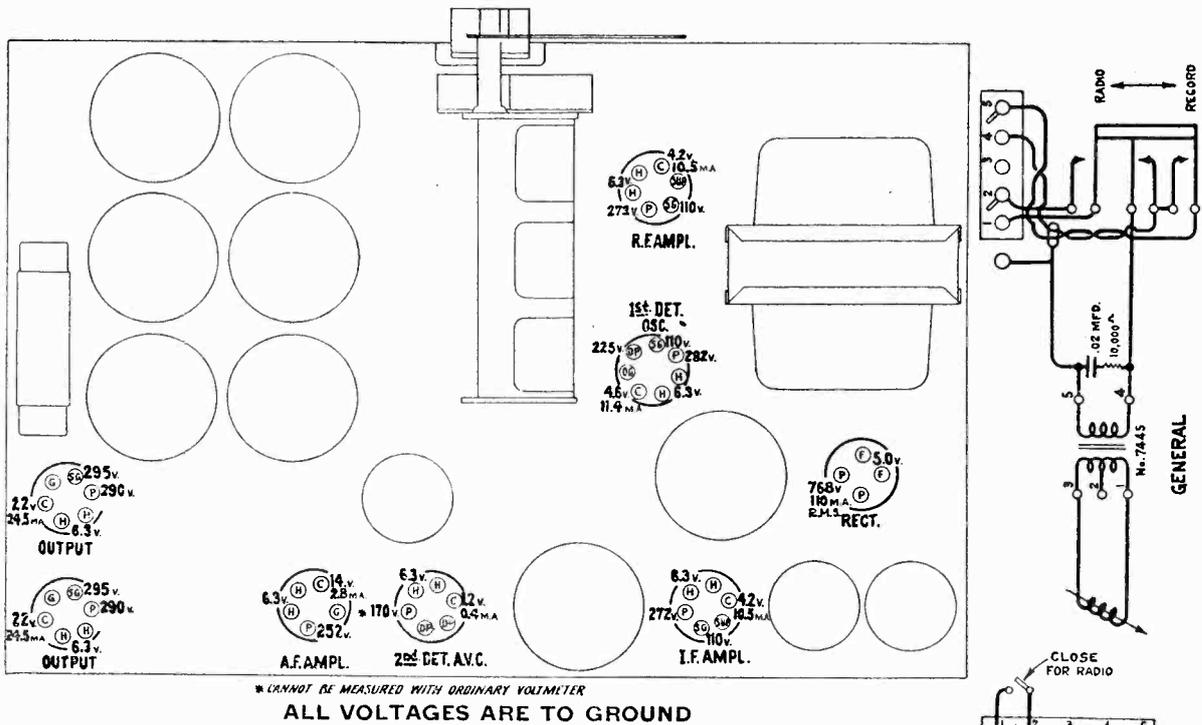
Figure 10—Radiotron Socket Voltages
