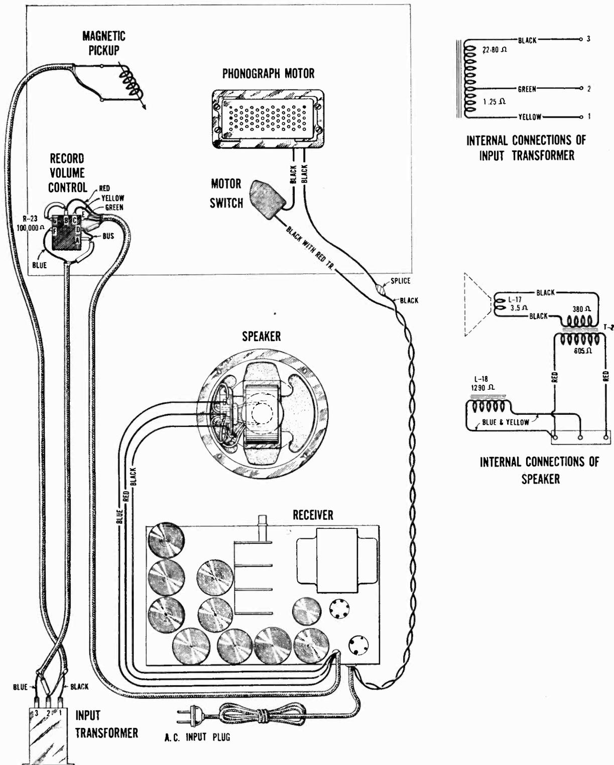
Figure C—Assembly Wiring Diagram
