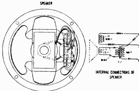
Figure C—Loudspeaker Wiring
