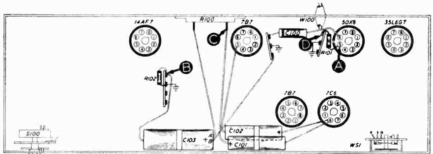
Figure 1. Bottom View, Showing Section 1 Test Points TP-3395A
