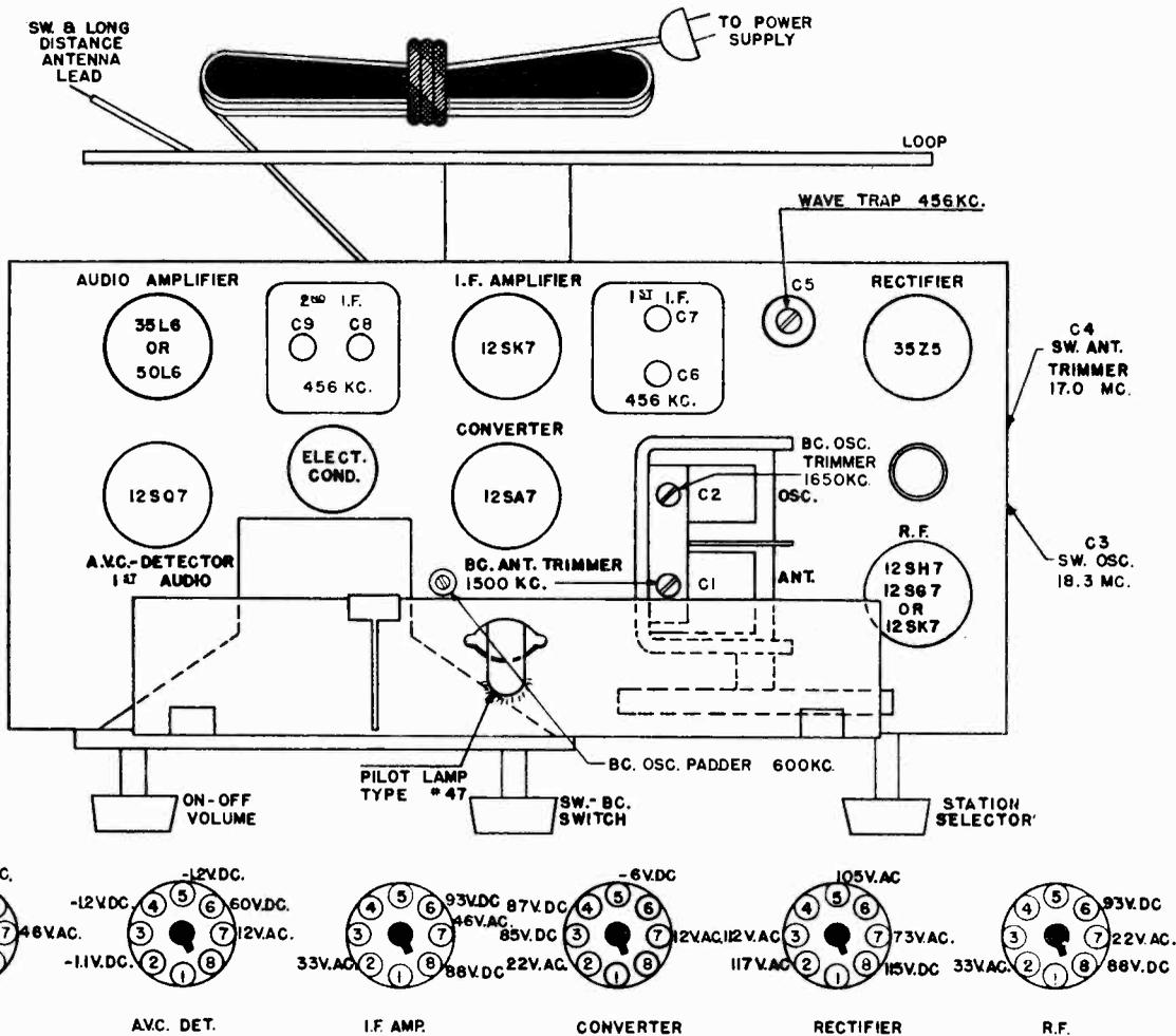
VOLTAGES TAKEN WITH 20KΩ PER VOLT METER WITH CHASSIS GROUND, AT 1000KC.
