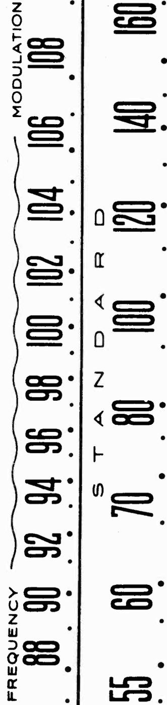
The dial scale drawing shown is a full size reproduction. It can be used as a reference in alignment procedure.
