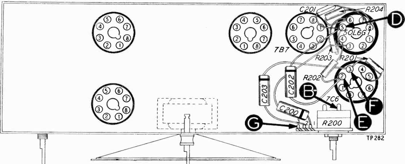
Figure 6. Bottom view, showing section 2 test points.
