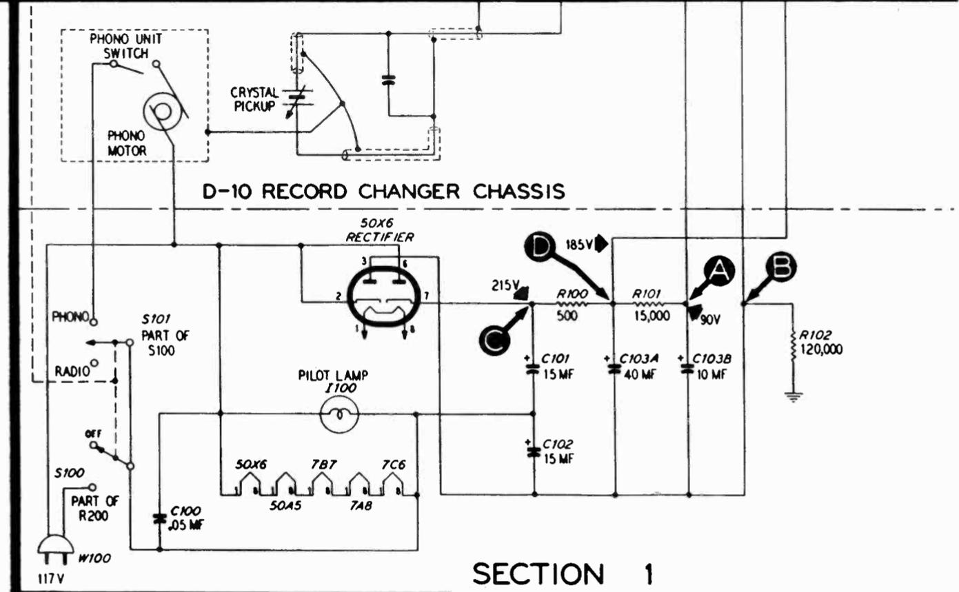
Figure 5. Philco Radio-Phonograph Models 48-1201 and 48-1260. Sectionalized Schematic Diagram, Showing Test Points
