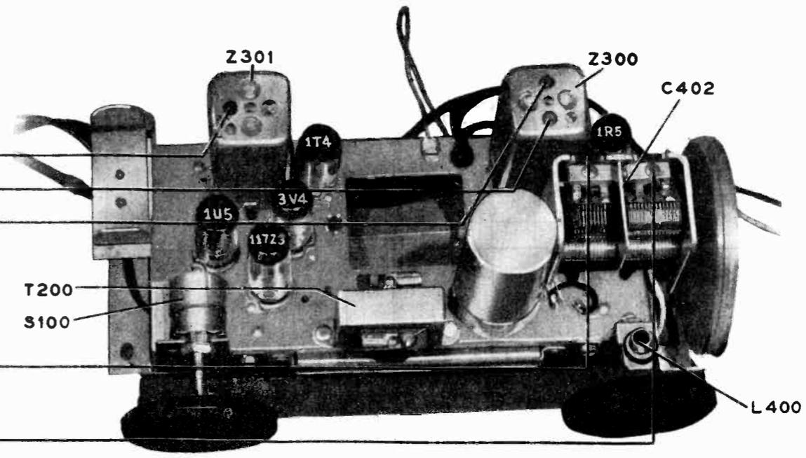
FIGURE 6. TOP VIEW, SHOWING TRIMMER LOCATIONS
