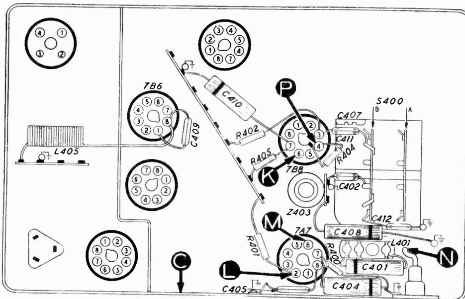
Bottom view, showing Section 4 test points.
