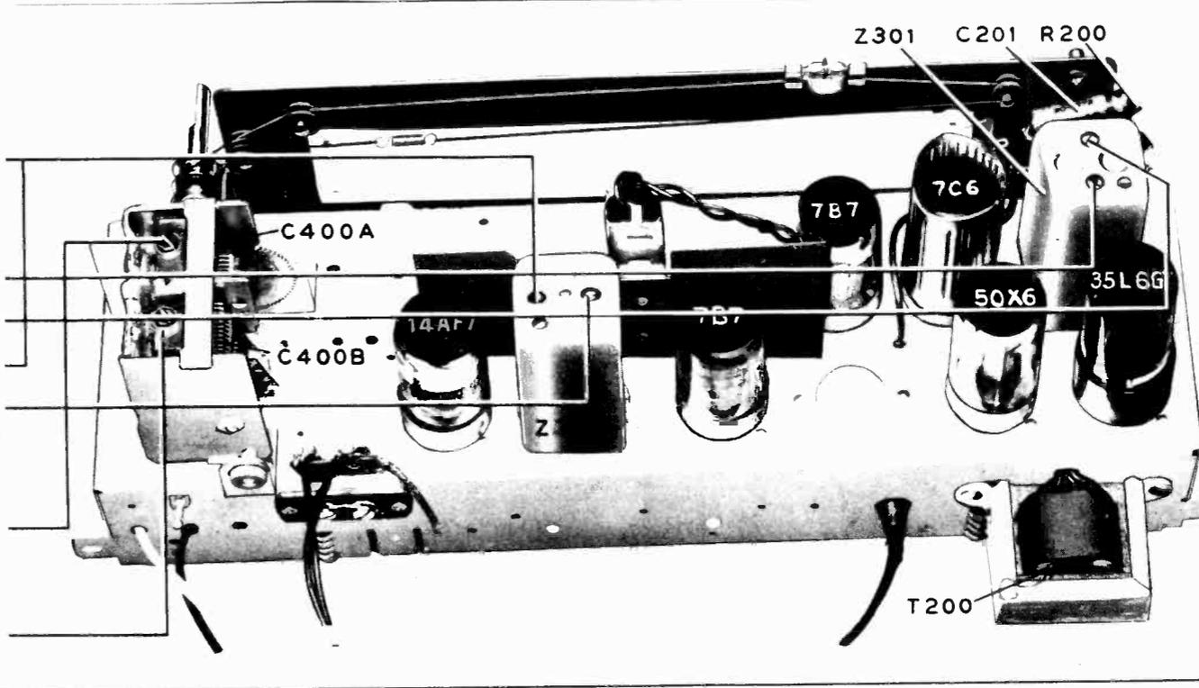
Figure 7. Top View, Showing Trimmer Locations
