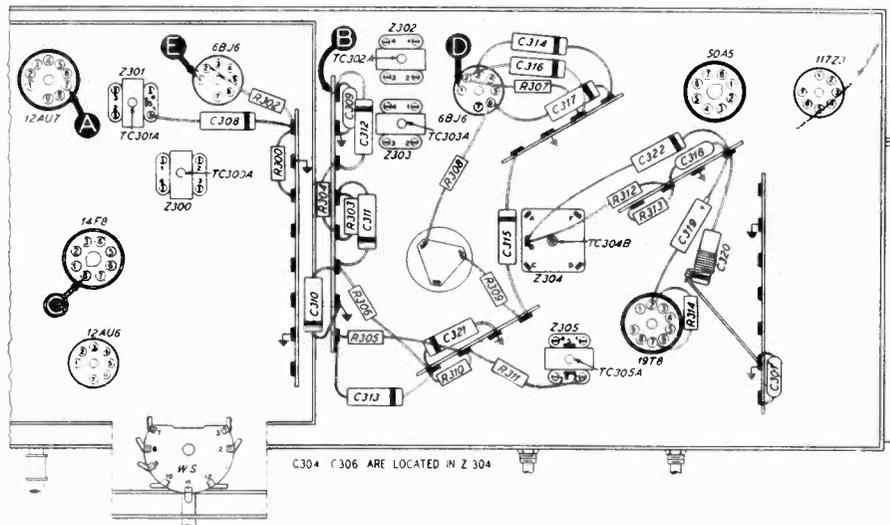
Figure 3. Bottom View, Showing Section 3 Test Points TP-5398C
