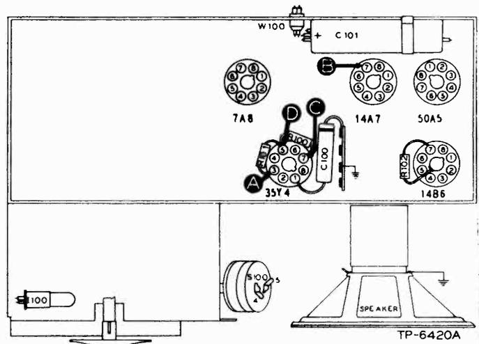
Figure 1. Bottom View, Showing Section 1 Test Points
