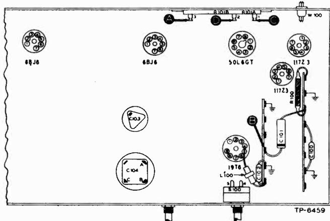
Figure 1. Bottom View, Showing Section 1 Test Points
