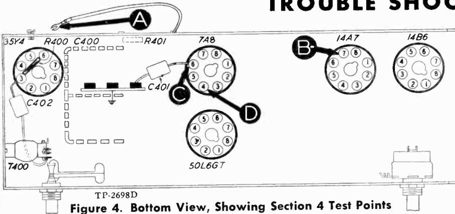
Make tests for this section by using an r-f signal generator with modulated output. Set frequency as noted in chart. Connect generator ground lead to B-; connect output lead through a .1-mf condenser to the test points indicated in the chart.
