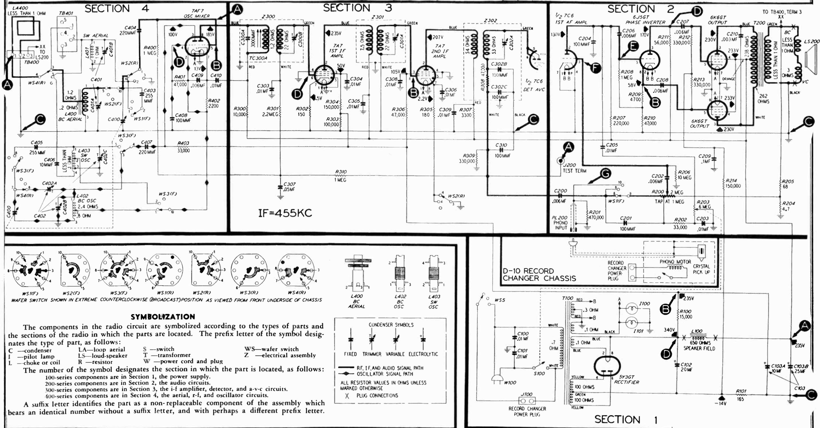
Figure 5. Philco Radio-Phonograph Model 48-1263, Sectionalized Schematic Diagram, Showing Test Points
