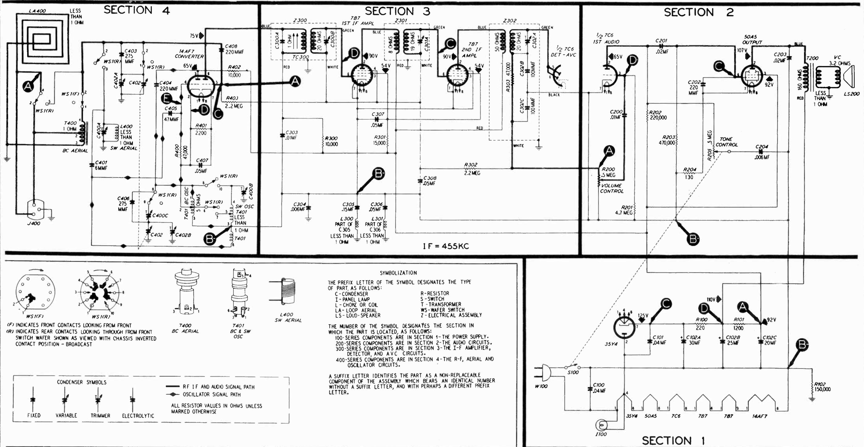
FIGURE 5. PHILCO RADIO MODEL 48-464, SECTIONALIZED SCHEMATIC, SHOWING TEST POINTS.
