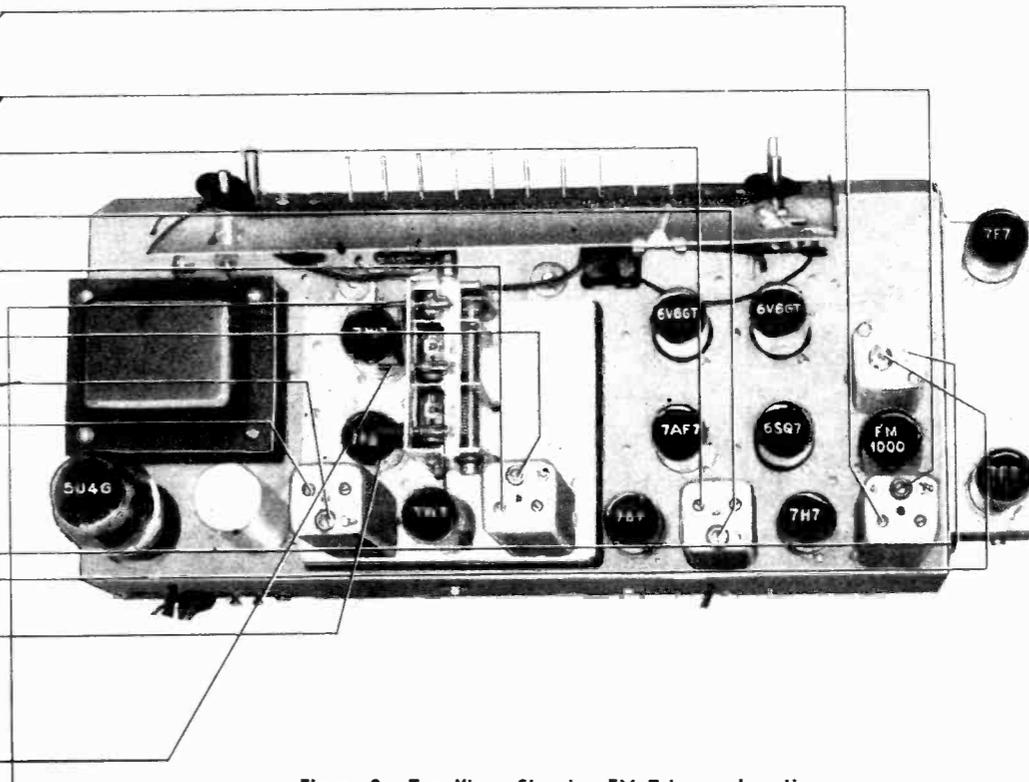
Figure 9. Top View, Showing FM Trimmer Locations
