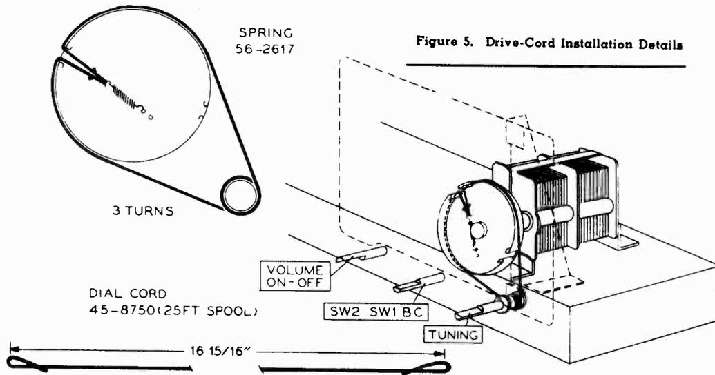
Figure 5. Drive-Cord Installation Details
