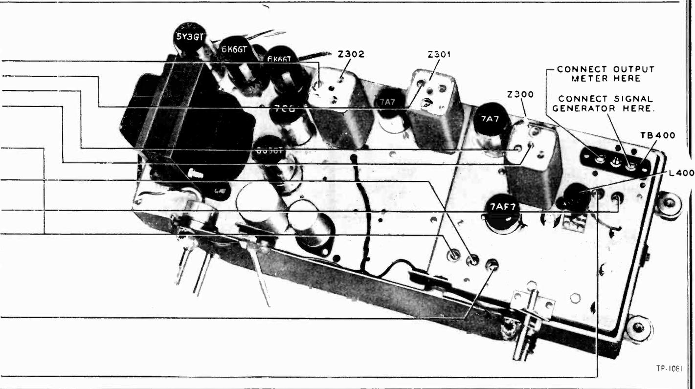
Figure 7. Top View, Showing Trimmer Locations
