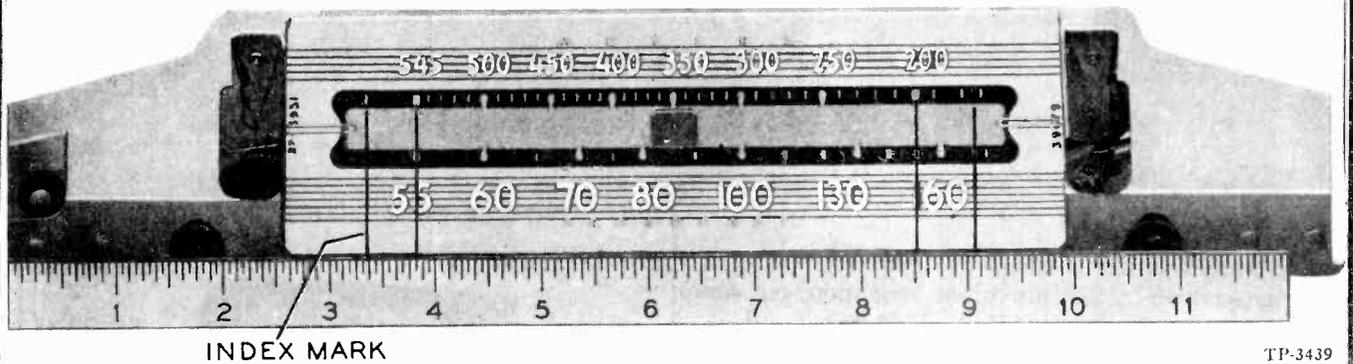
Figure 8. Composite Dial and Backplate, Calibration Details
