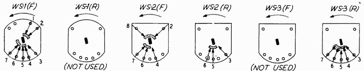
ROTARY WAFER SWITCH SECTIONS ARE SHOWN (AS VIEWED WITH CHASSIS INVERTED) IN THE POSITION FOR BROADCAST, SHORT-WAVE, PUSH-BUTTON, OR PHONO OPERATION. THESE SECTIONS ARE THROWN TO THE FM POSITION WHEN ACTUATED BY THE FM PUSH BUTTON. WAFER SECTIONS ARE SYMBOLIZED WS-1, WS-2, WS-3, FROM FRONT OF CHASSIS TOWARD REAR. (F) INDICATES FRONT CONTACTS, LOOKING FROM FRONT. (R) INDICATES REAR CONTACTS, LOOKING THROUGH FROM FRONT.
