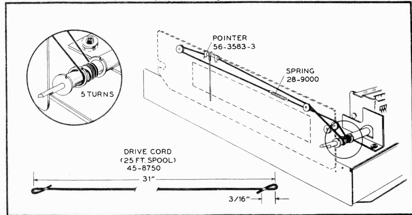
Figure 8. Drive-Cord Installation Details
