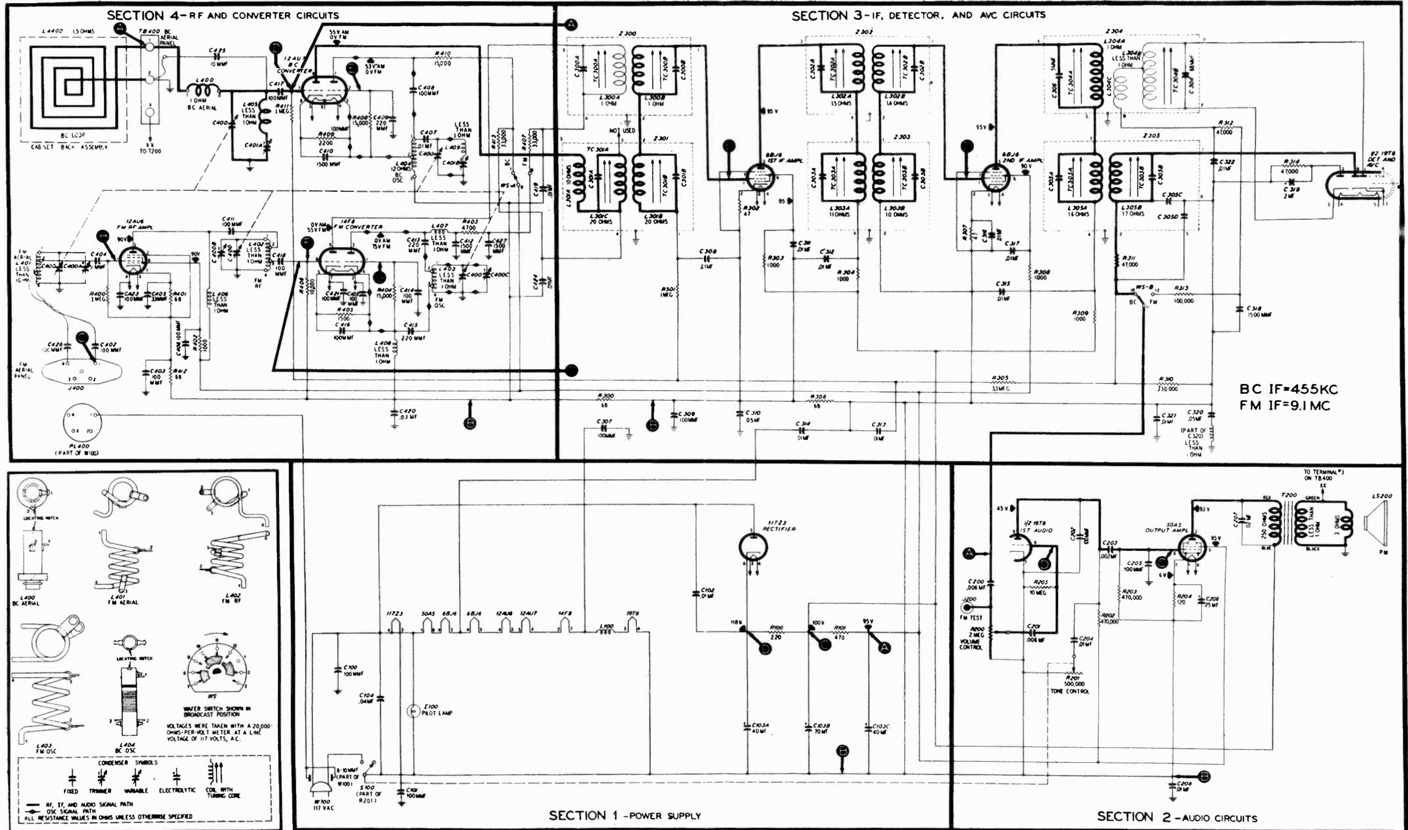
Figure 6. Philco Radio Model 48-472, Code 122, Sectionalized Schematic Diagram, Showing Test Points
