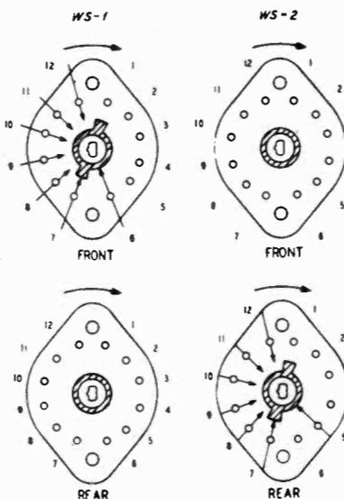
SIX POSITION WAFER SWITCH SHOWN IN BROADCAST POSITION.
