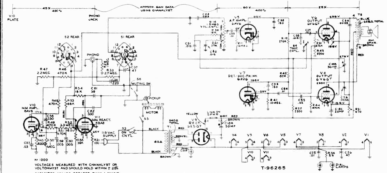
NOTE: VOLTAGES MEASURED WITH CHANALYST OR VOLTCOMYST AND SHOULD HOLD WITHIN ± 20%. CAPACITOR VALUES GREATER THAN 1 IN MMF. UNLESS OTHERWISE INDICATED. LESS THAN 1 IN MF.
