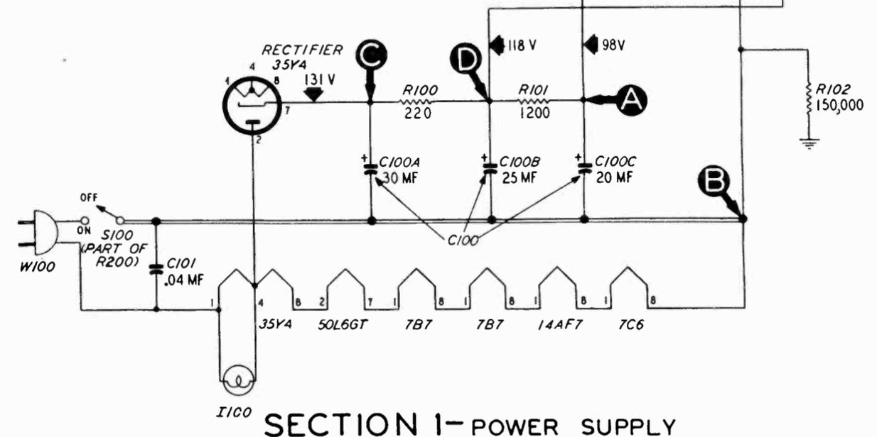
FIGURE 5. PHILCO RADIO, MODELS 49-900-E AND 49-900-I, SECTIONALIZED SCHEMATIC DIAGRAM, SHOWING TEST POINTS
