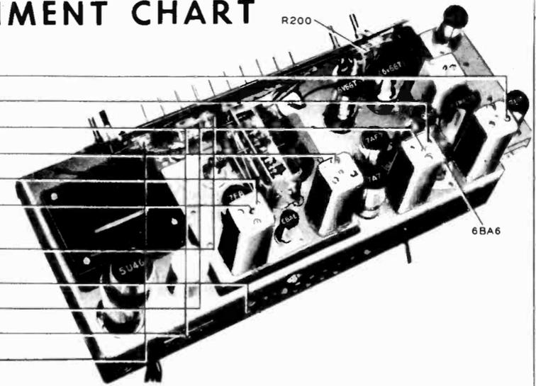
Figure 8. Top View, Showing AM Trimmer Locations
