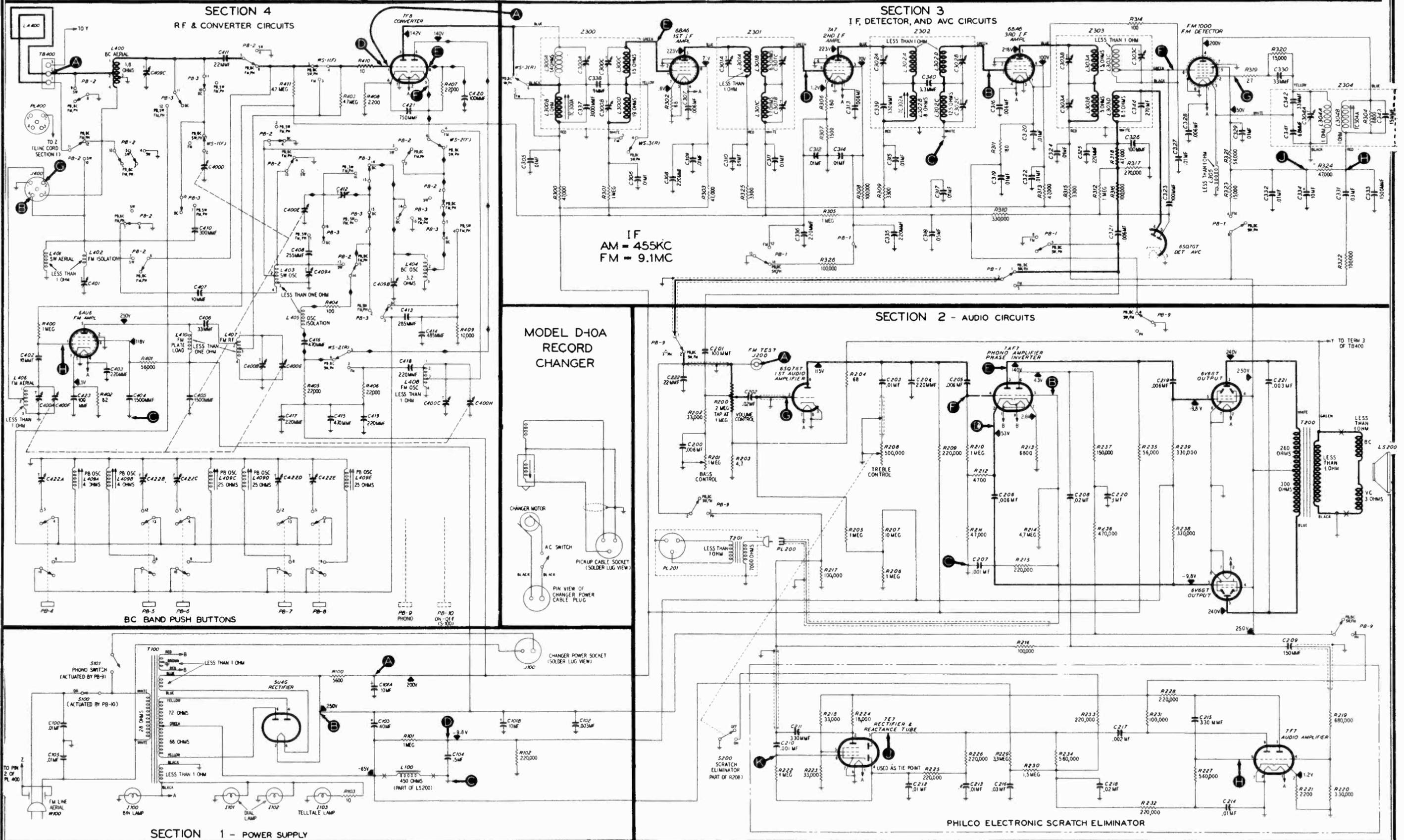
Figure 7. Philco Radio-Phonograph Model 48-1290, Sectionalized Schematic Diagram, Showing Test Points
