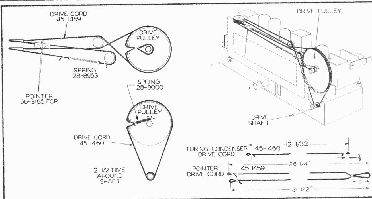
Figure 8. Drive-Cord Installation Details
