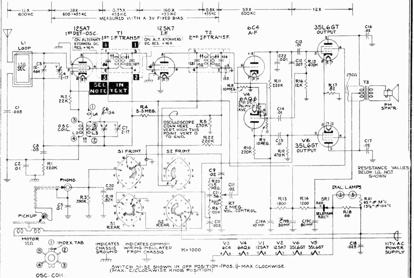
The first I-F transformer shown in the schematic is stamped 970441-1. Some chassis will have a first I-F transformer stamped 970441-5. Connections to this alternate transformer are as shown in the block letters. Performance will be identical for both sets.
