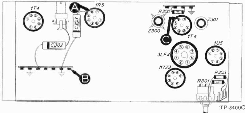
Figure 3. Bottom View, Showing Section 3 Test Points
