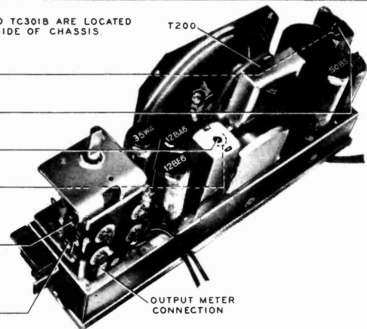
Figure 6. Top View, Showing Trimmer Locations
