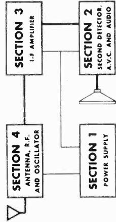
Block diagram (Heavy lines indicate signal path.)
