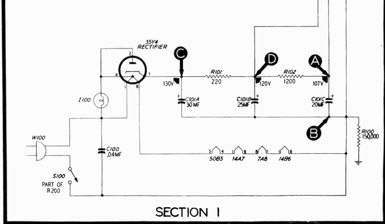
FIGURE 5. PHILCO RADIO MODELS 48-250 AND 48-250-I, SECTIONALIZED SCHEMATIC DIAGRAM, SHOWING TEST POINTS
