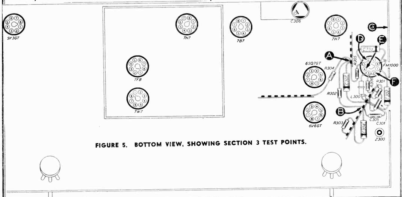
FIGURE 5. BOTTOM VIEW, SHOWING SECTION 3 TEST POINTS.
