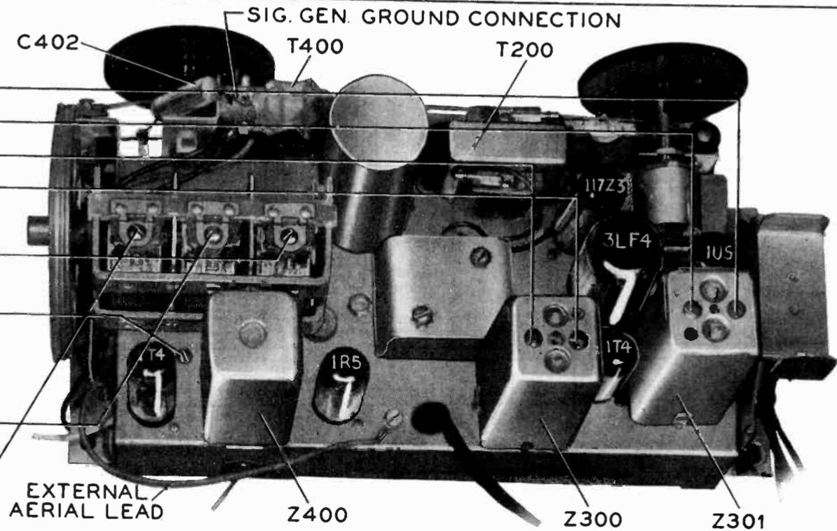
Figure 6. Top View, Showing Trimmer Locations
