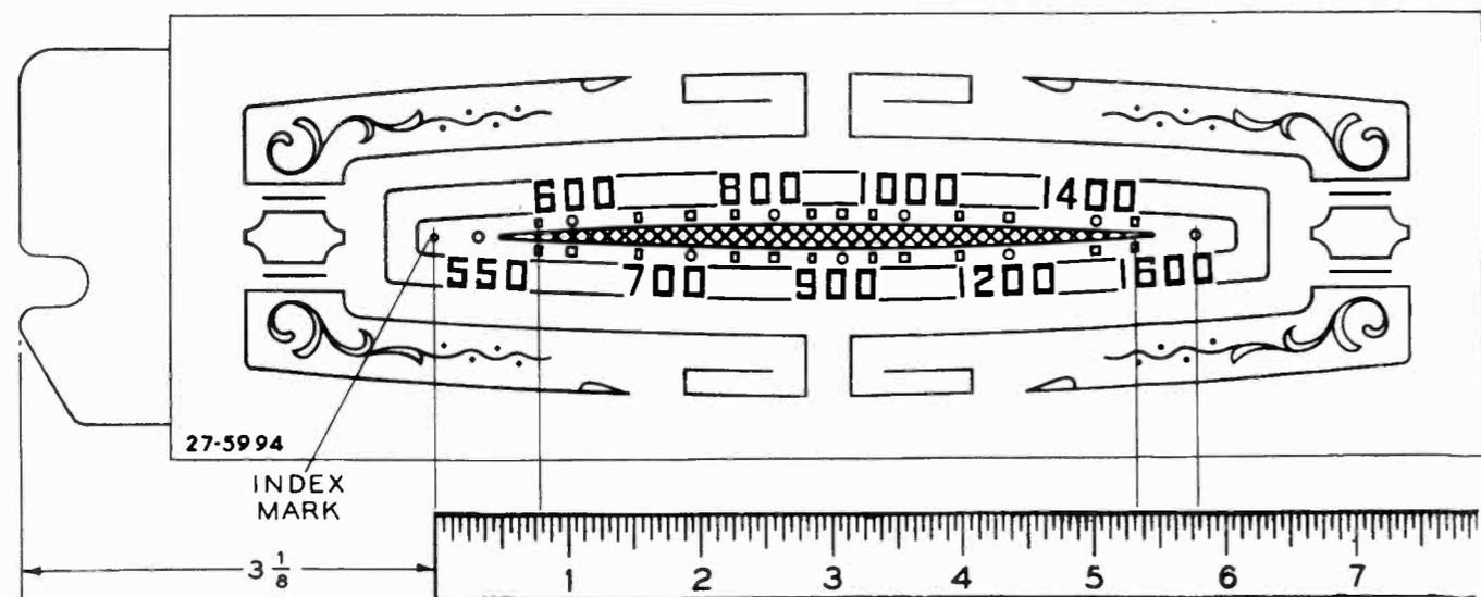
Figure 6. Calibration Measurements for Dial Backplate
