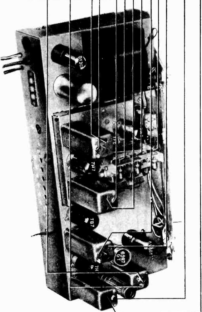
FIGURE 10. CHASSIS VIEW, SHOWING FM TRIMMER LOCATIONS.
