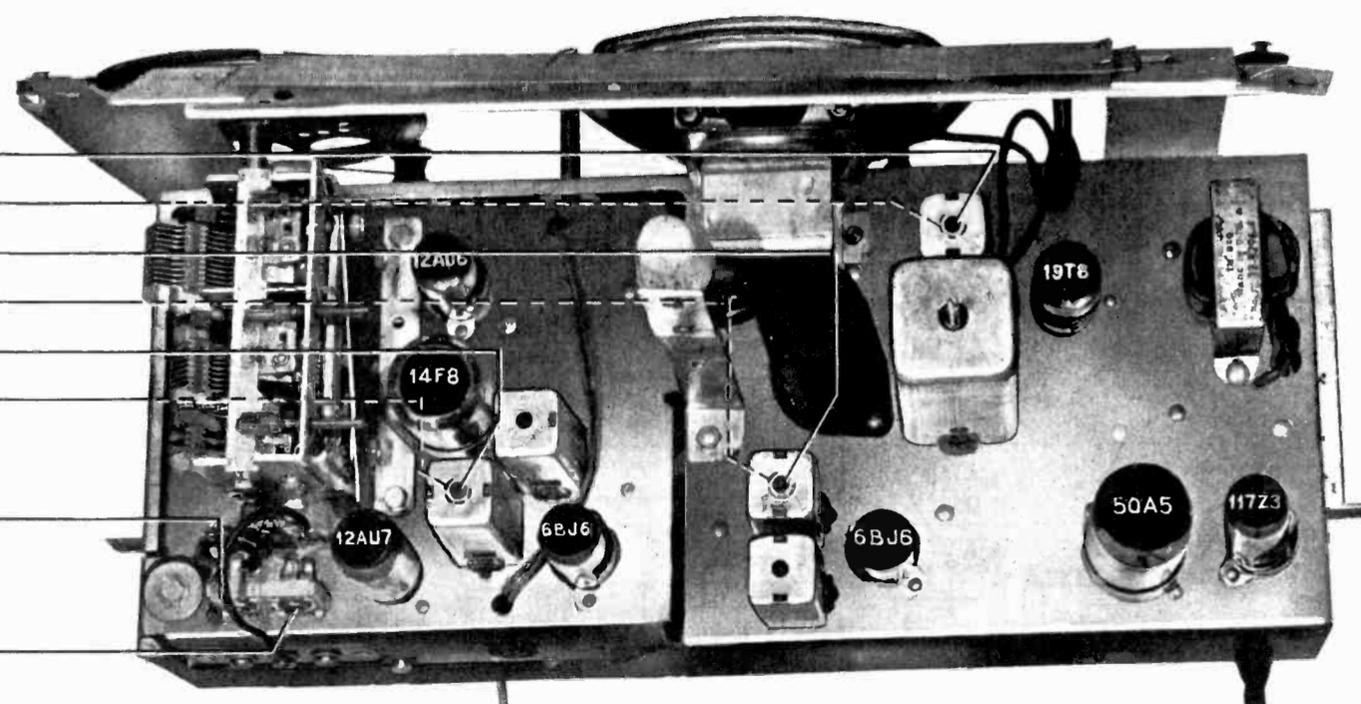
Figure 8. Top View, Showing AM Trimmer Locations
