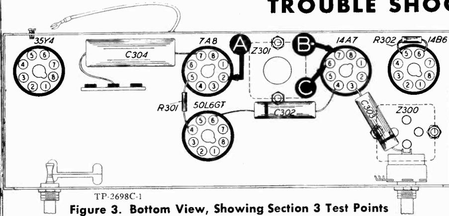
Make tests for this section by using an r-f signal generator with modulated output. Set generator frequency to 455 kc. Connect ground lead of signal generator to B-; connect output lead through a .1-mf condenser to the test points indicated in the chart. Set the volume control at maximum. If "NORMAL INDICATION" is obtained in step 1, proceed with tests for Section 4; if not, isolate and correct the trouble within this section.
