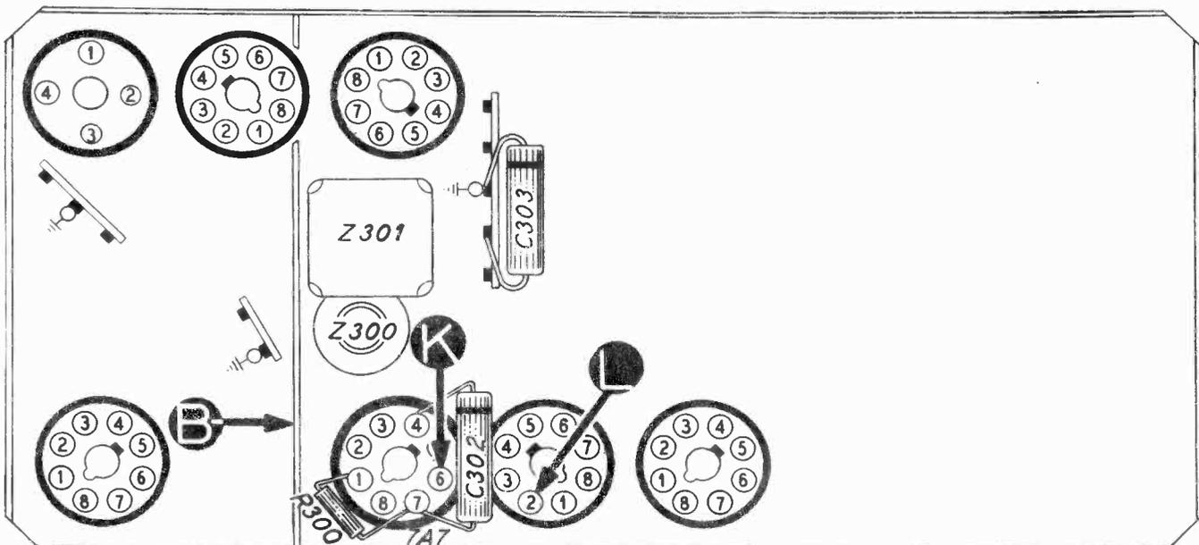
Bottom view, showing Section 3 test points.
