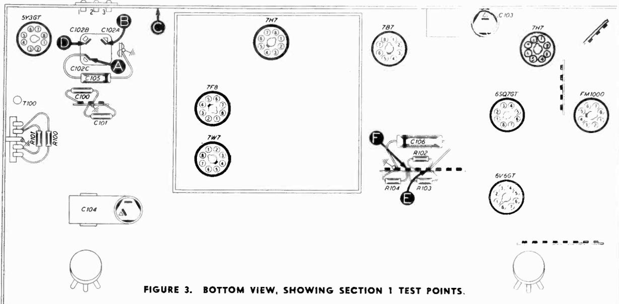
FIGURE 3. BOTTOM VIEW, SHOWING SECTION 1 TEST POINTS.
