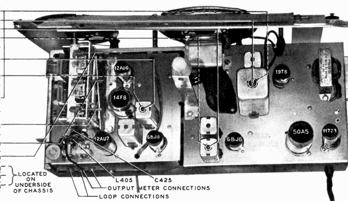
Figure 9. Top View, Showing FM Trimmer Locations
