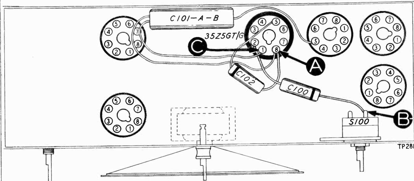
Figure 4. Bottom view, showing section 1 test points.
