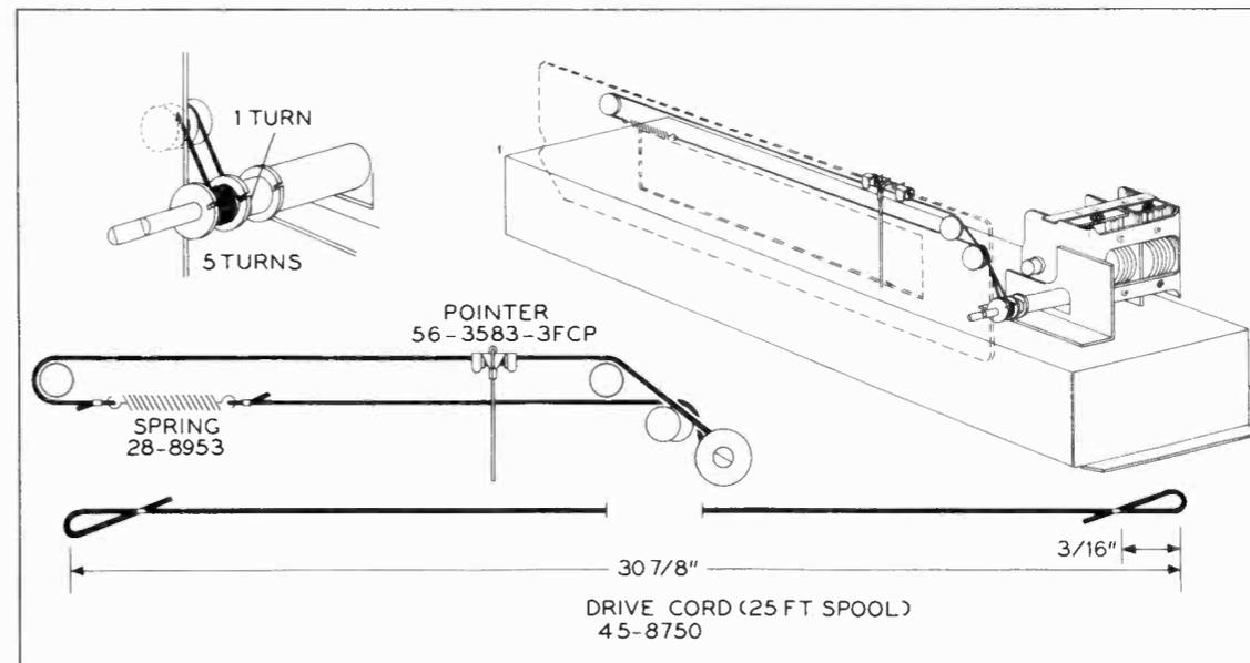
Figure 8. Drive-Cord Installation Details
