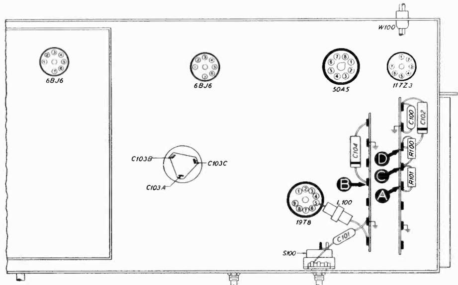
Figure 1. Bottom View, Showing Section 1 Test Points
