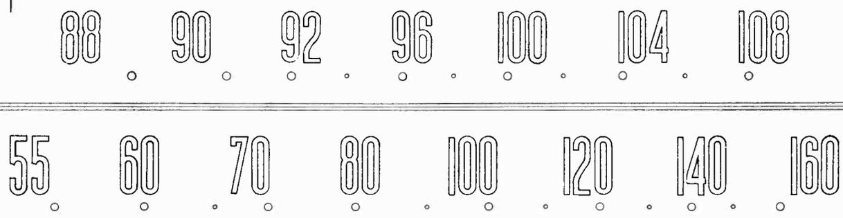
The dial scale drawing shown is a full size reproduction. It can be used as a reference in alignment procedure.
