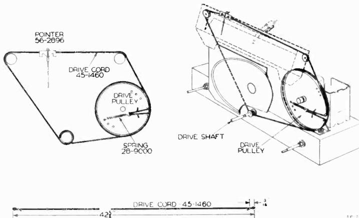
Figure 13. Drive cord installation details.
