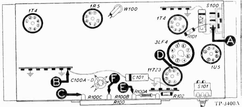
Figure 1. Bottom View, Showing Section 1 Test Points
