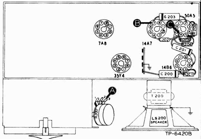
Figure 2. Bottom View, Showing Section 2 Test Points
