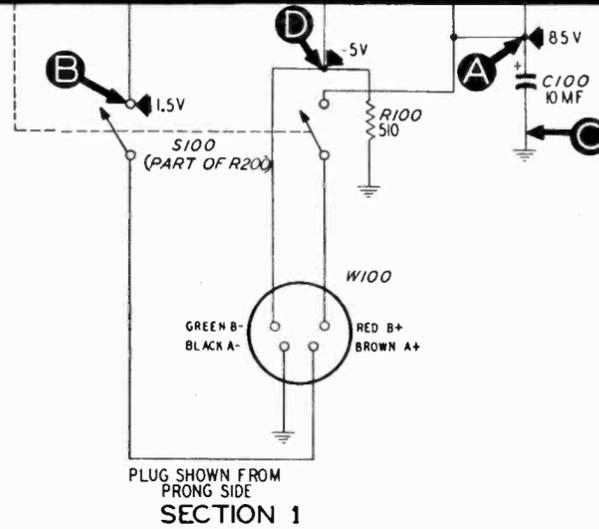
FIGURE 5. PHILCO RADIO MODELS 48-141 AND 48-145, COMPLETE SECTIONALIZED SCHEMATIC, SHOWING ALL TEST POINTS
