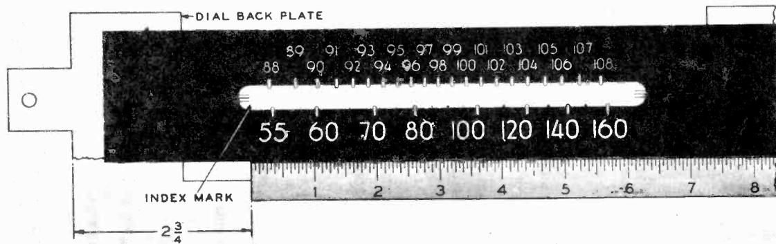
Figure 7. Dial-Backplate Calibration Measurements
