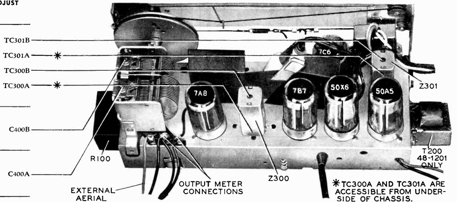
Figure 7. Top View, Showing Trimmer Locations
