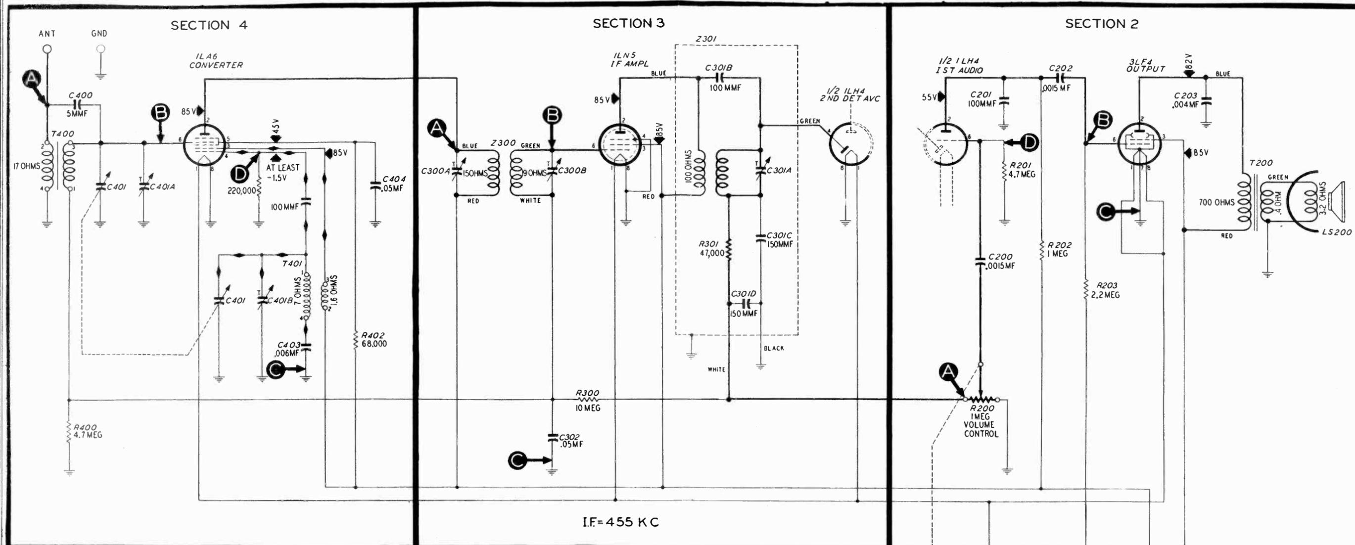
NOTE: THE VOLTAGES INDICATED ON THE SCHEMATIC DIAGRAM ARE AVERAGE VALUES. THE VOLTAGES WERE MEASURED BETWEEN THE POINTS INDICATED AND THE CHASSIS, USING A 20,000-OHMS PER-VOLT METER, WITH A FRESH BATTERY. OSCILLATOR GRID VOLTAGE WAS MEASURED BETWEEN THE CHASSIS AND OSC. GRID (PIN 4) OF THE 1LA6 TUBE, USING A 100,000-OHM ISOLATING RESISTOR IN SERIES WITH THE PROD END OF THE NEGATIVE VOLTMETER LEAD.
