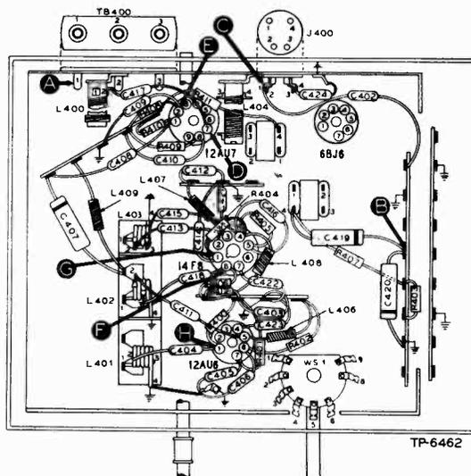
Figure 4. Bottom View, Showing Section 4 Test Points
