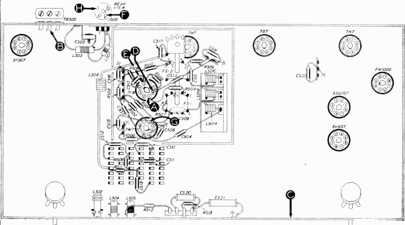
BOTTOM VIEW, SHOWING SECTION 5 TEST POINTS.
