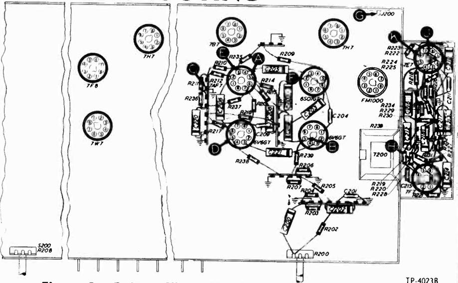
Figure 3. Bottom View, Showing Section 2 Test Points
