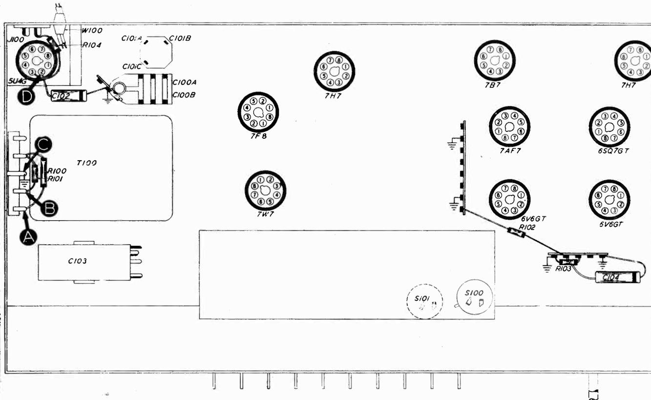
**Figure 2. Bottom View, Showing Section 1 Test Points**
