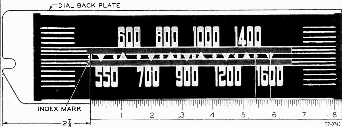
Figure 6. Calibration Measurements for Dial Backplate
