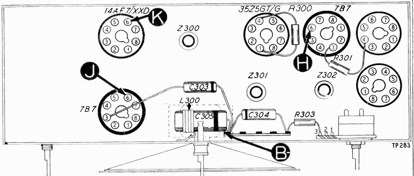
Figure 8. Bottom view, showing section 3 test points.
