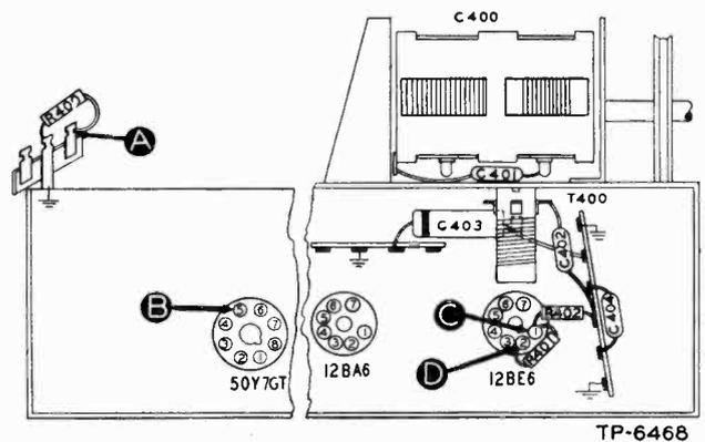
**Figure 4. Bottom View, Showing Section 4 Test Points**
