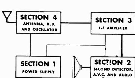
Figure 1. Block diagram (Heavy lines indicate signal path).
