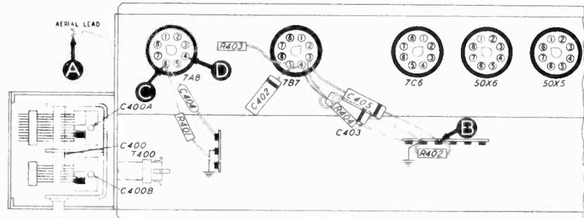
**Figure 4. Bottom View, Showing Section 4 Test Points**
