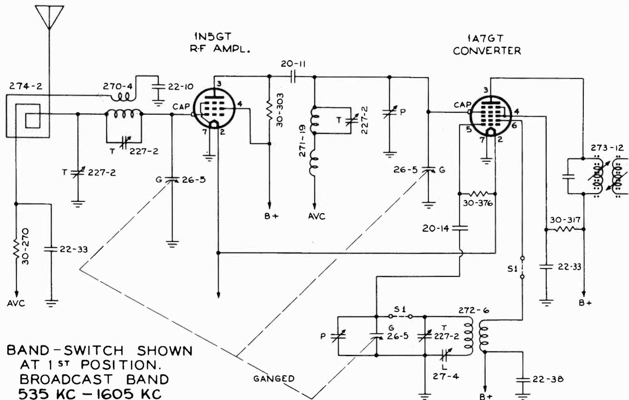
BAND-SWITCH SHOWN AT 1<sup>ST</sup> POSITION. BROADCAST BAND 535 KC - 1605 KC
