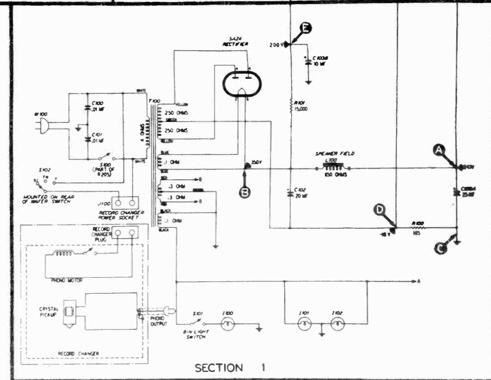
Figure 7. Philco Radio-Phonograph Model 48-1264, Sectionalized Schematic Diagram, Showing Test Points
