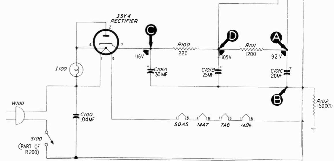
Philco Radio Models 49-501 and 49-501-I, Sectionalized Schematic Diagram, Showing Test Points
