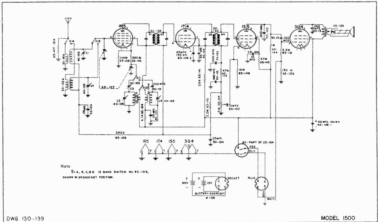
THE MODEL 1500 is a 4-tube battery-operated superheterodyne farm radio receiver with two tuning ranges for reception of standard broadcast and short-wave stations. The tuning range of the broadcast frequency is 540 to 1650 kilocycles, or 560 to 182 meters. The short wave frequency is 5.8 to 18.3 in megacycles, or 16 to 49 meters, which include the following 16, 19, 25, 31, 39 and 49 meter bands.
