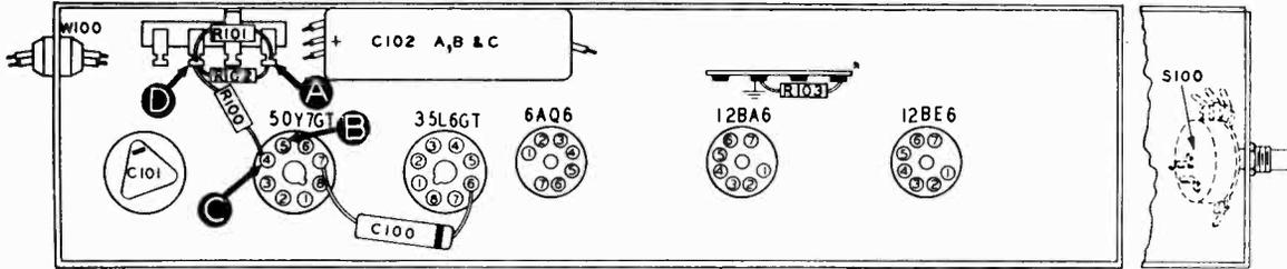
Figure 1. Bottom View, Showing Section 1 Test Points
