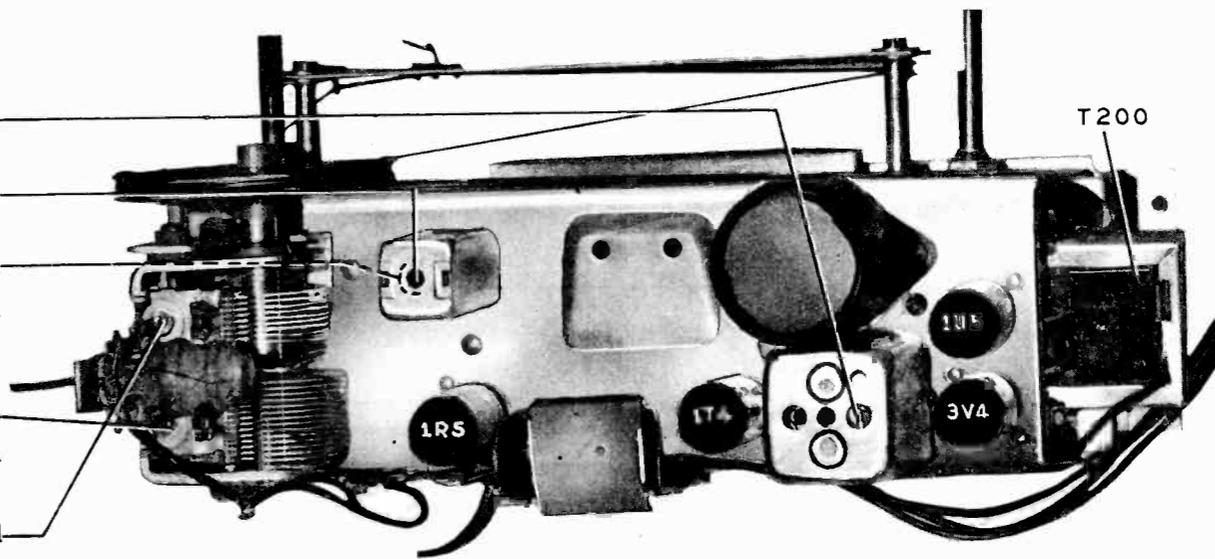
Figure 6. Top View, Showing Trimmer Locations
