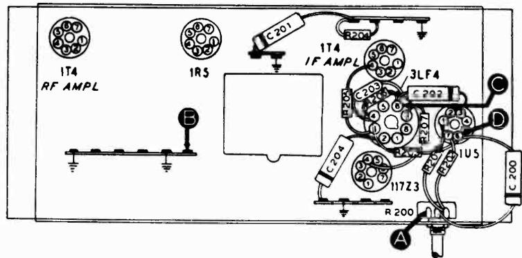
FIGURE 2. BOTTOM VIEW, SHOWING SECTION 2 TEST POINTS
