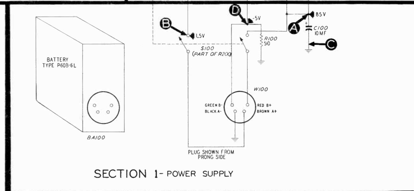
FIGURE 5. PHILCO RADIO MODEL 49-100, COMPLETE SECTIONALIZED SCHEMATIC, SHOWING ALL TEST POINTS
