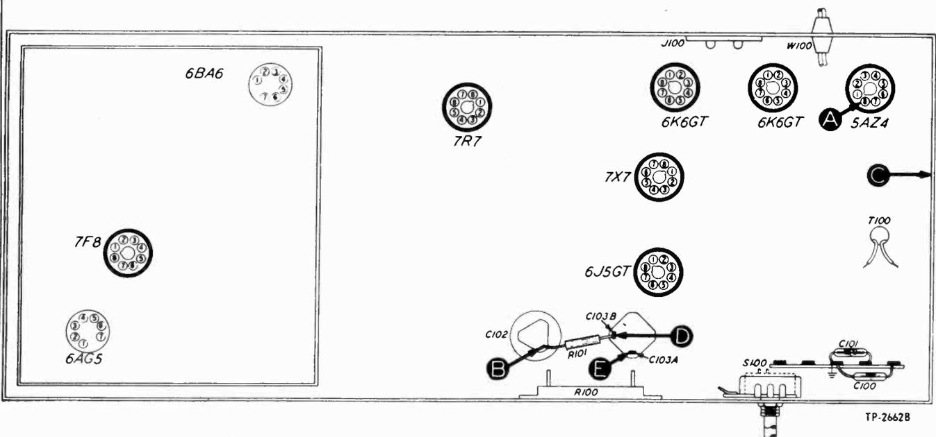
FIGURE 3. BOTTOM VIEW, SHOWING SECTION 1 TEST POINTS.
