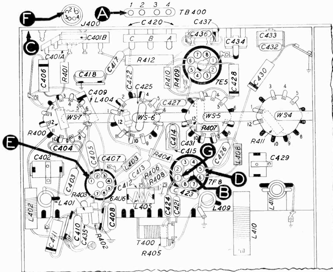
FIGURE 4. BOTTOM VIEW, SHOWING SECTION 4 TEST POINTS
