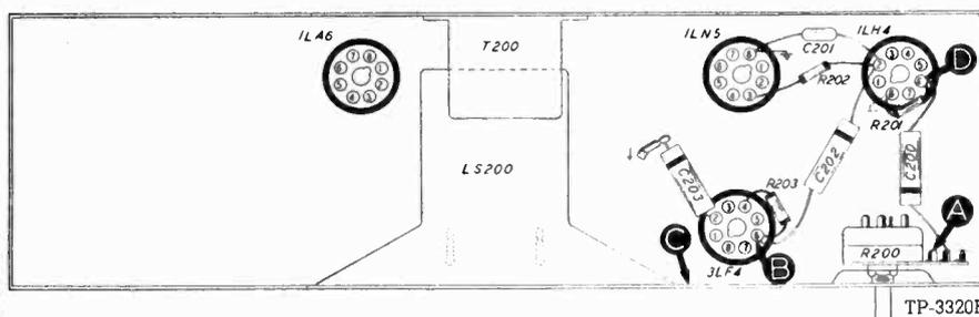
Figure 2. Bottom View, Showing Section 2 Test Points
