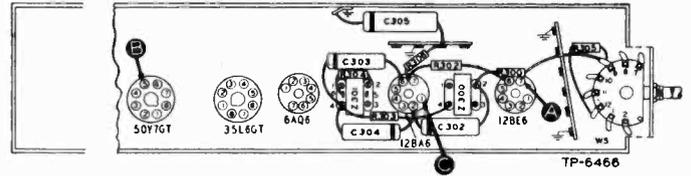
**Figure 3. Bottom View, Showing Section 3 Test Points**
