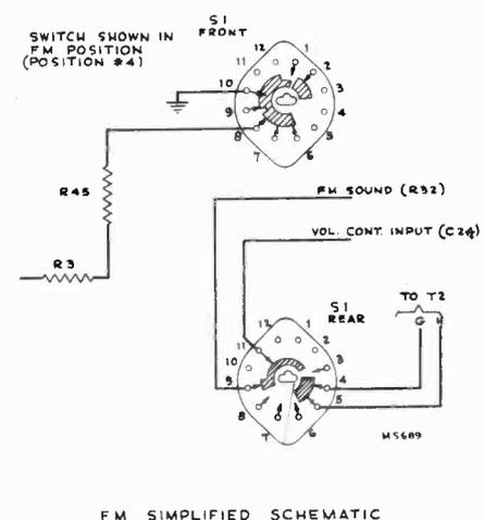
The schematic diagrams above show the selector switch (S1) used in RC-616H and RC-618A. The connections to S2 are identical in all chassis—note that position No. 2 (PHONO) of RC-616H and RC-618A corresponds to position No. 1 (PHONO) of RC-616A and RC-618. No connections are made through S2 when in AUX. position.
