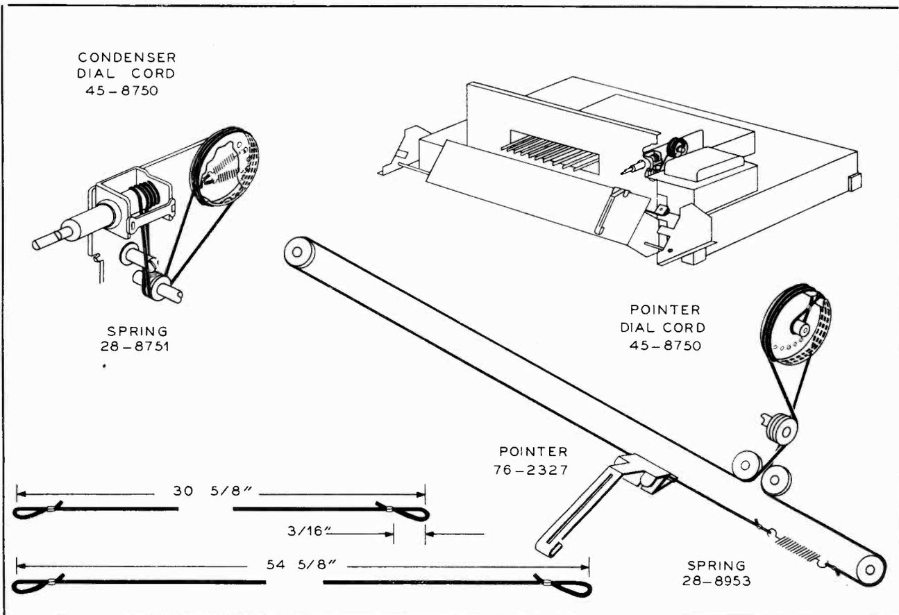
FIGURE 7. DRIVE-CORD INSTALLATION DETAILS
