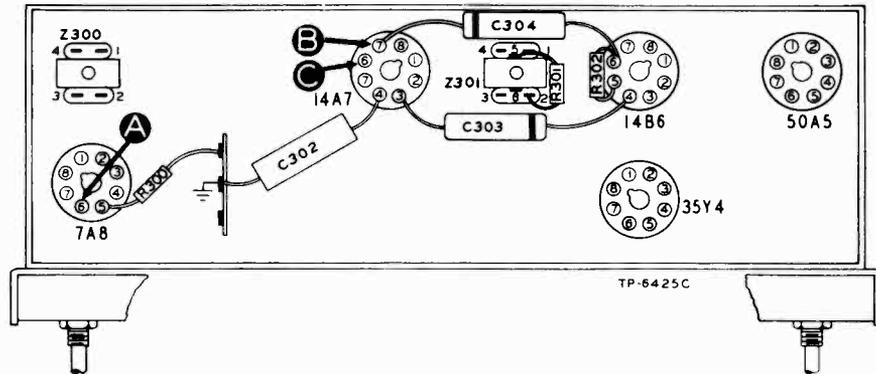
**Figure 3. Bottom View, Showing Section 3 Test Points**
