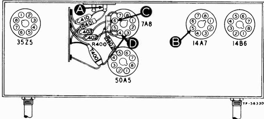
FIGURE 4. BOTTOM VIEW, SHOWING SECTION 4 TEST POINTS
