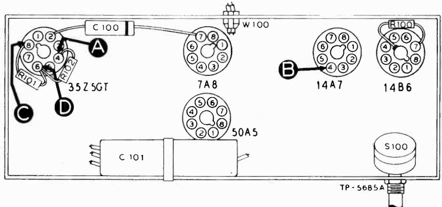
Figure 1. Bottom View, Showing Section 1 Test Points
