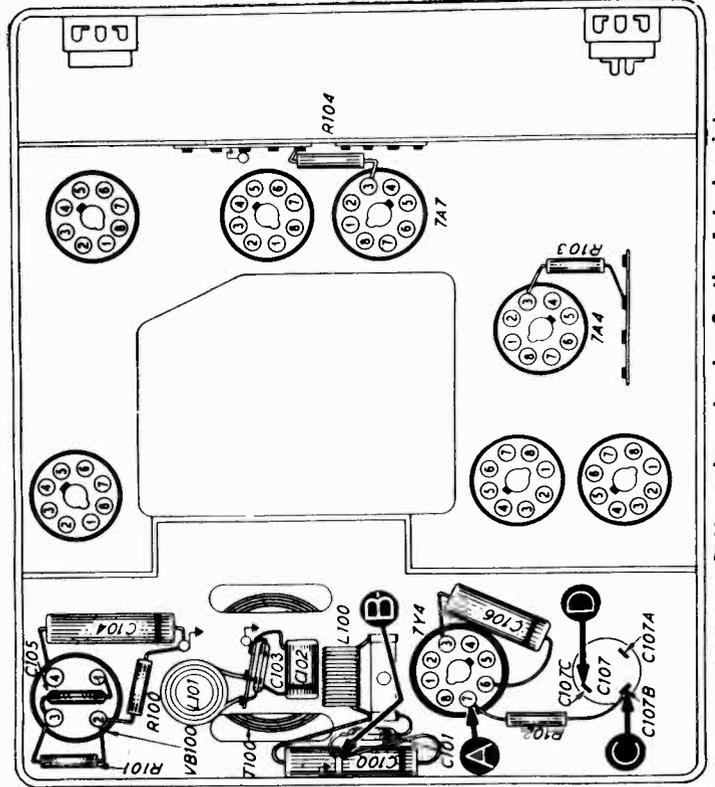
Bottom view, showing Section 1 test points.
