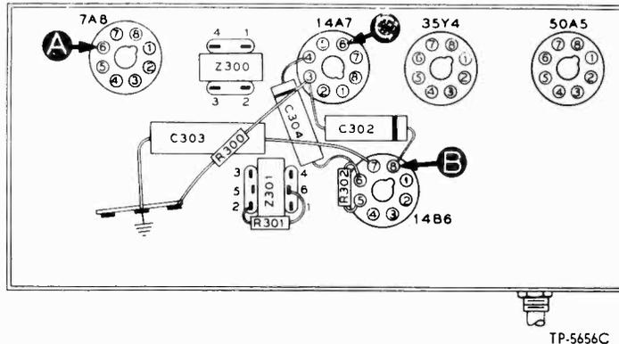
Figure 3. Bottom View, Showing Section 3 Test Points
