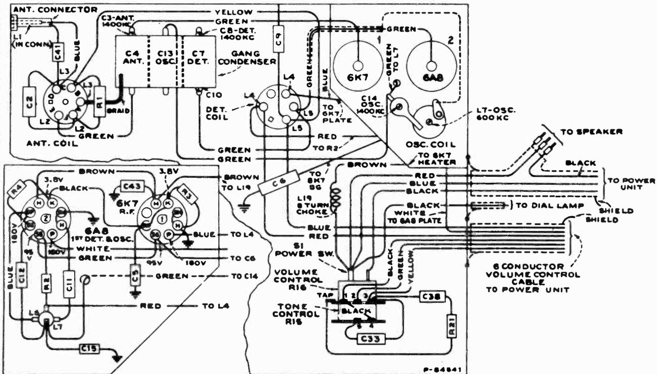
Control Unit Parts, Socket Voltages, and Trimmers
