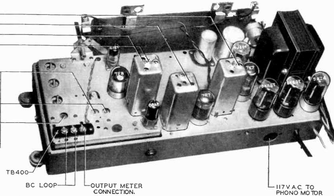
FIGURE 8. CHASSIS VIEW, SHOWING AM TRIMMER LOCATIONS.
