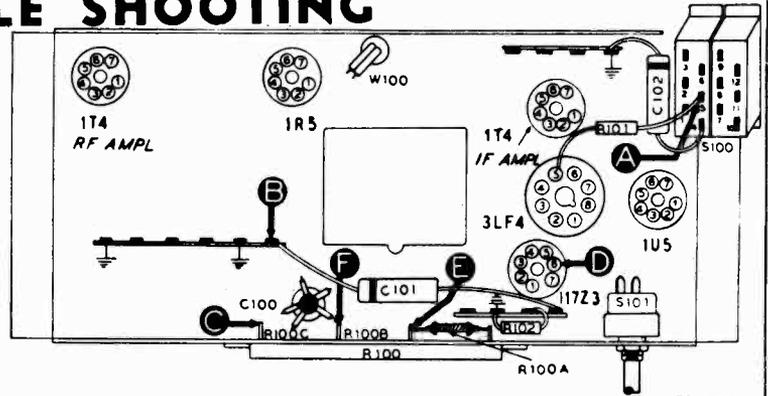
FIGURE 1. BOTTOM VIEW, SHOWING SECTION 1 TEST POINTS
