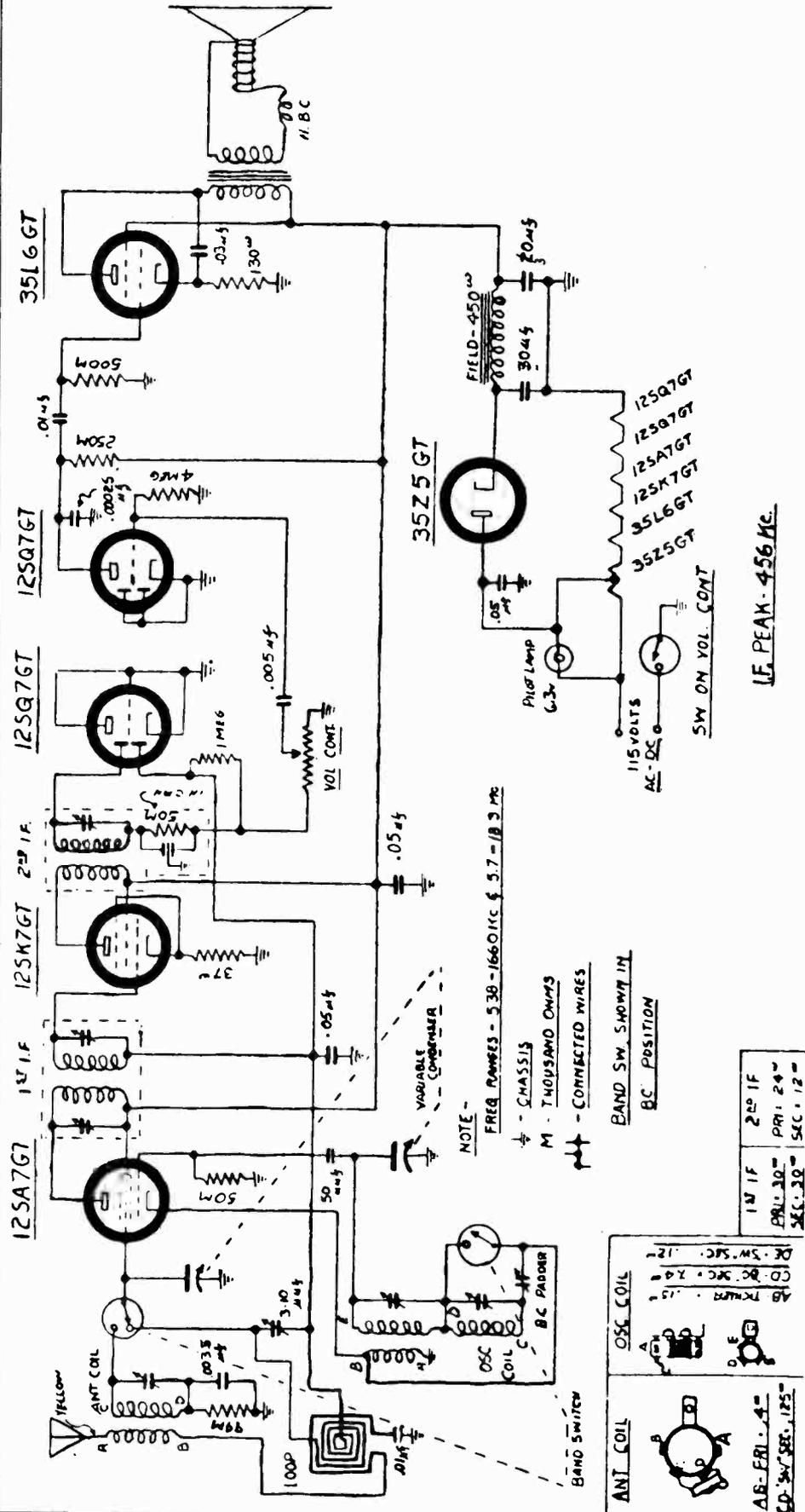
This 6 Tube Superheterodyne is designed to operate on 115 volts, 40 to 60 cycles, alternating current (AC) or 115 volts direct current (DC).
