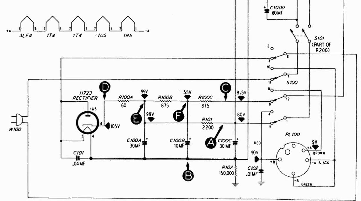
FIGURE 5. PHILCO RADIO MODEL 49-605, SECTIONALIZED SCHEMATIC DIAGRAM, SHOWING TEST POINTS
