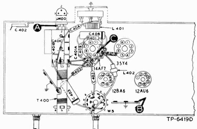
**Figure 4. Bottom View, Showing Section 4 Test Points**
