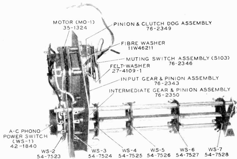
FIGURE 5. PHILCO AUTOMATIC-BAND-SELECTOR MECHANISM
