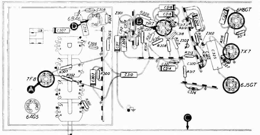
Figure 5. Bottom View, Showing Section 3 Test Points
