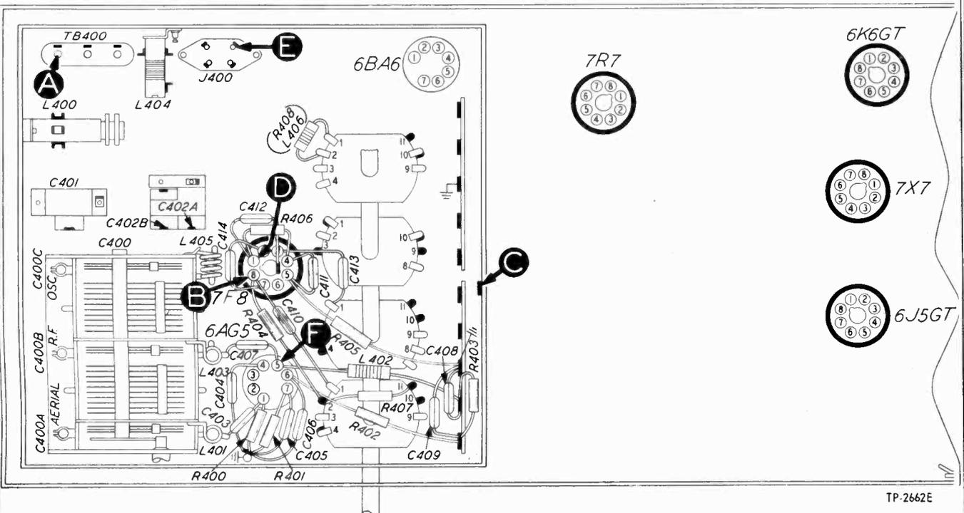
FIGURE 6. BOTTOM VIEW, SHOWING SECTION 4 TEST POINTS.
