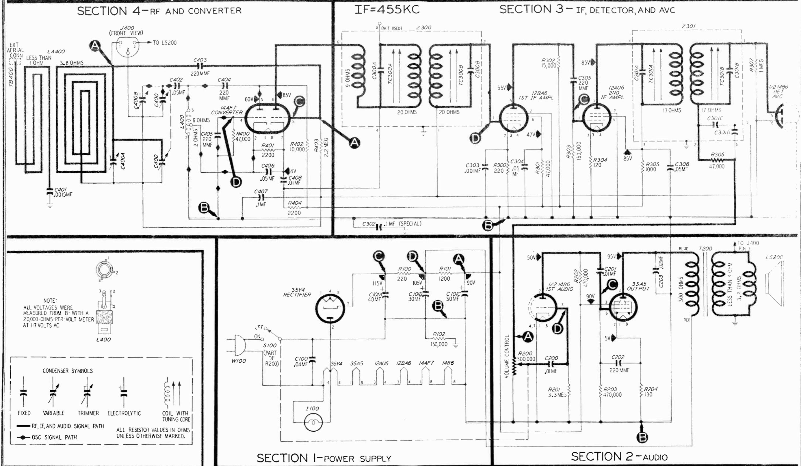
Figure 5. Philco Radio Model 49-902, Sectionalized Schematic Diagram, Showing Test Points
