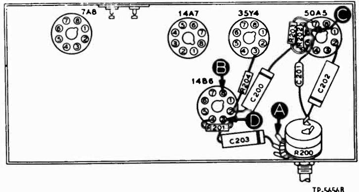
Figure 2. Bottom View, Showing Section 2 Test Points
