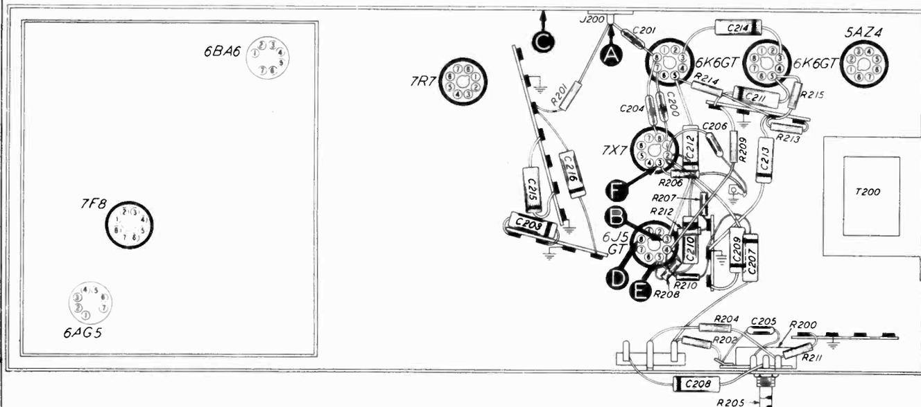
Figure 4. Bottom View, Showing Section 2 Test Points
