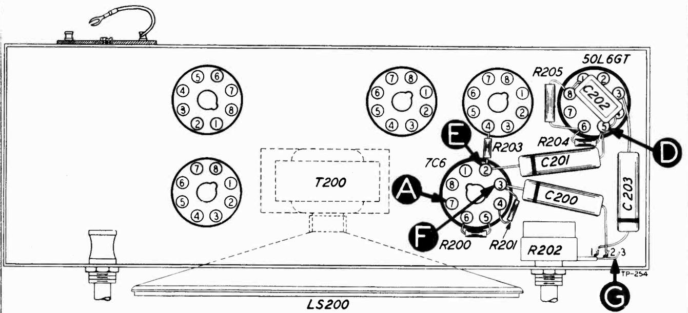
Figure 6. Bottom view showing section 2 test points.
