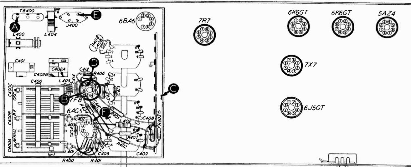
Figure 6. Bottom View, Showing Section 4 Test Points
