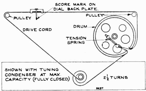
Dial Indicator and Drive Mechanism — Model 8V90
