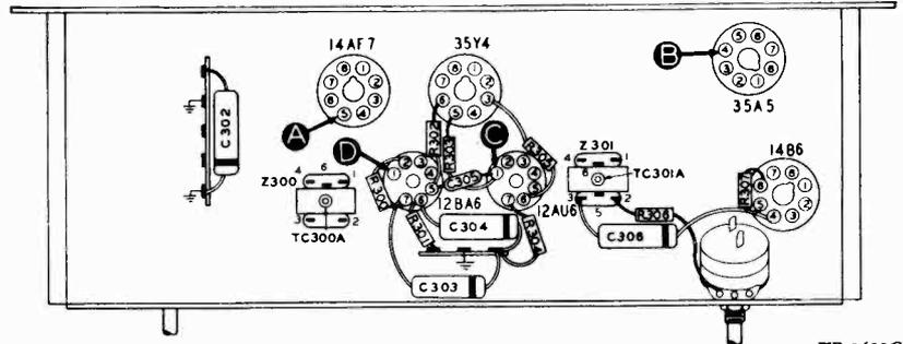
Figure 3. Bottom View, Showing Section 3 Test Points
