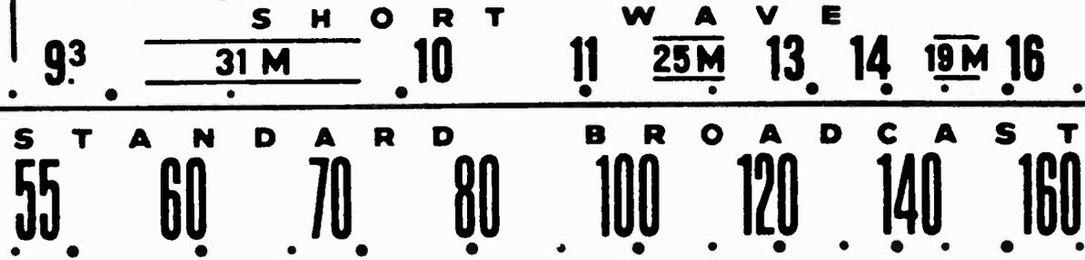
The dial scale drawing shown is a full size reproduction. It can be used as a reference in alignment procedure.
