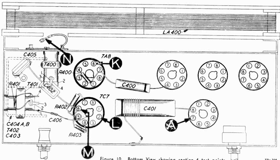
Figure 10. Bottom View showing section 4 test points.
