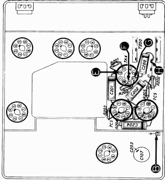
Bottom view, showing Section 2 test points.
