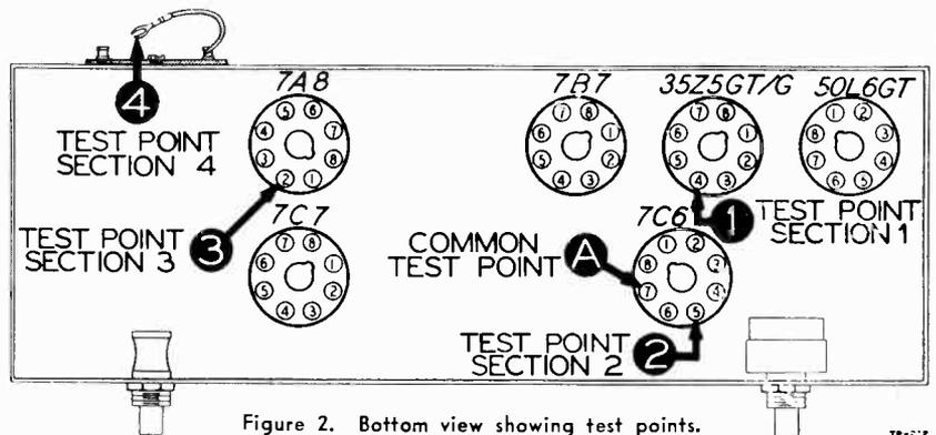
Figure 2. Bottom view showing test points.
