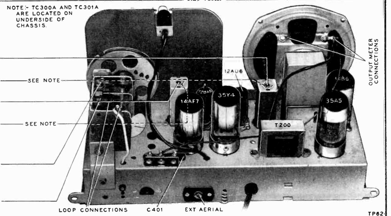
Figure 6. Top View of Chassis, Showing Trimmer Locations
