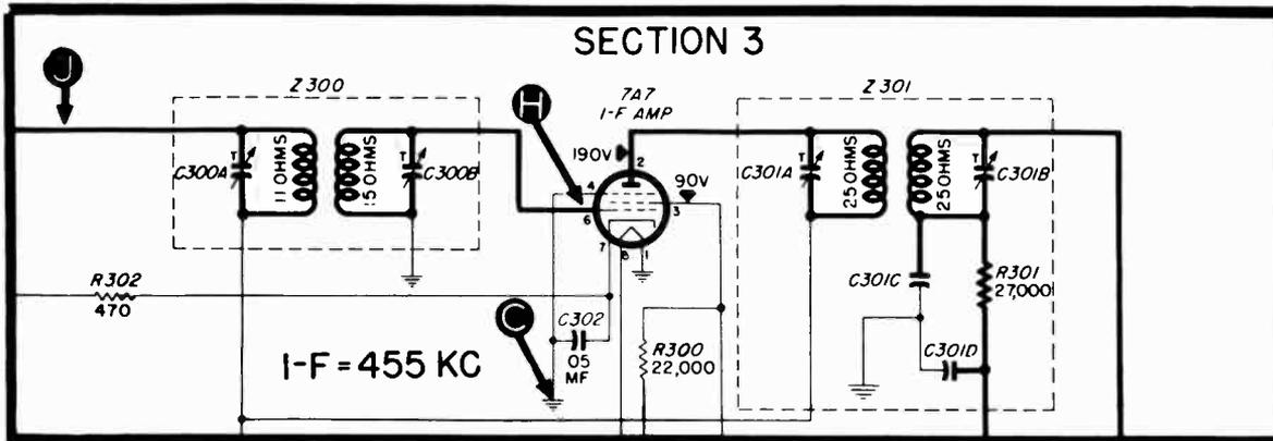
Figure 7. Section 3 schematic.
