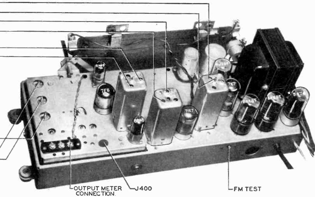
FIGURE 9. CHASSIS VIEW, SHOWING FM TRIMMER LOCATIONS.
