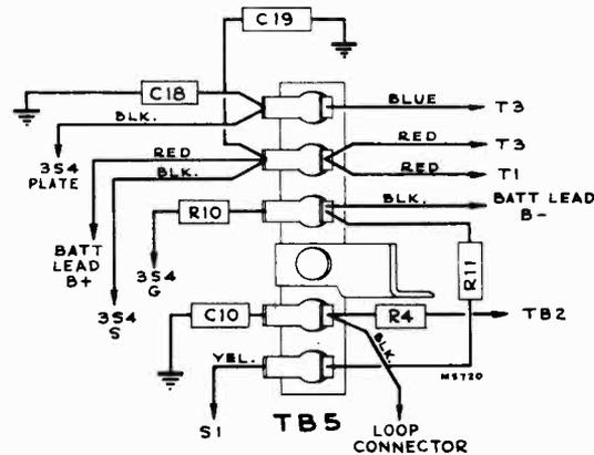
Terminal Board Wiring
