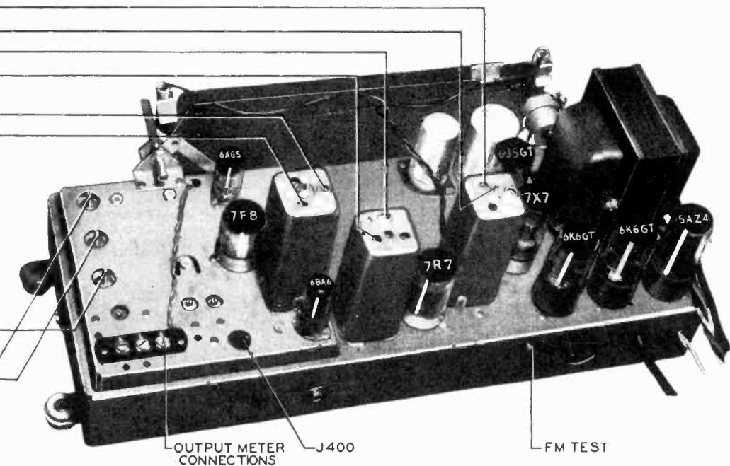
Figure 9. Top View, Showing FM Trimmer Locations
