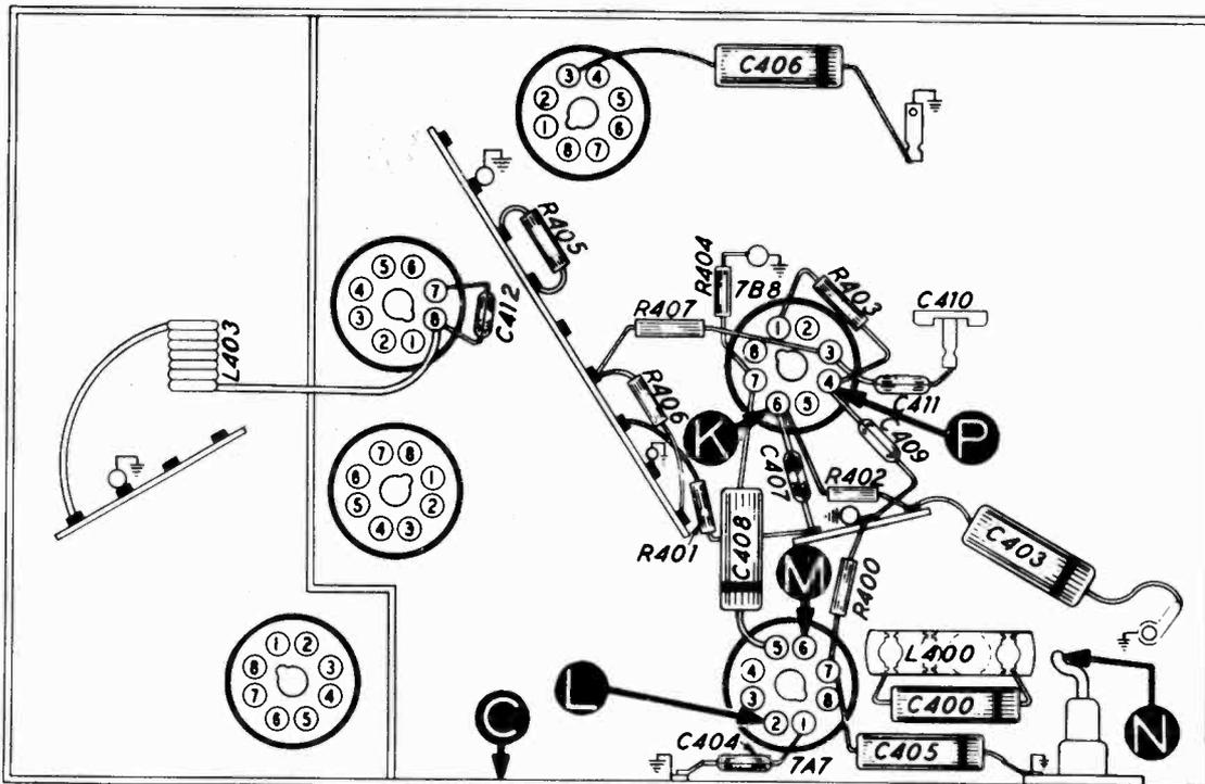
Figure 10. Bottom view, showing Section 4 test points.
