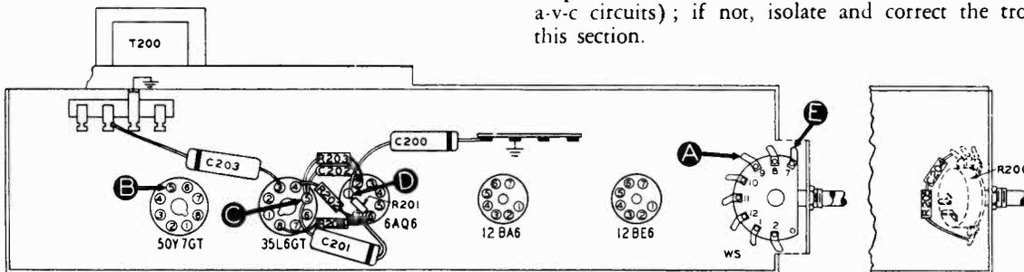
Figure 2. Bottom View, Showing Section 2 Test Points
