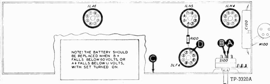
Figure 1. Bottom View, Showing Section 1 Test Points
