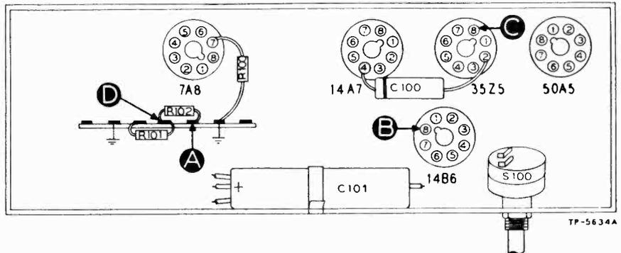
FIGURE 1. BOTTOM VIEW, SHOWING SECTION 1 TEST POINTS
