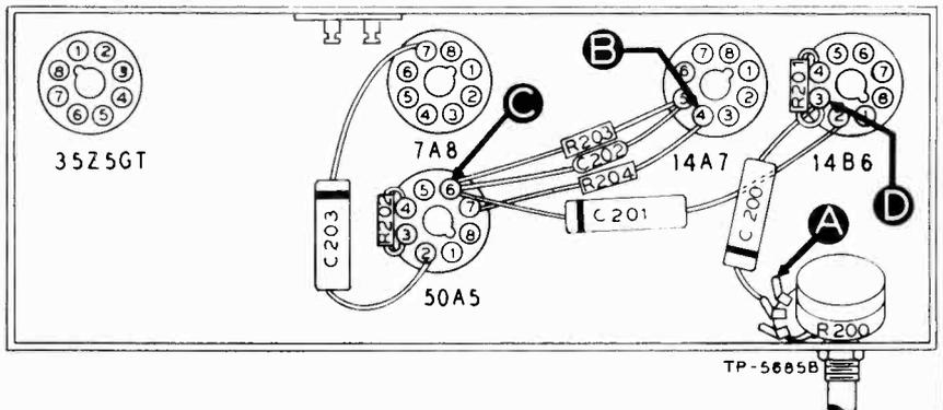
Figure 2. Bottom View, Showing Section 2 Test Points
