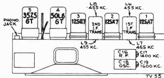
**1st I.F. Trans. Substitution.**—The first I.F. transformer may differ from that shown in the schematic diagram. Transformers stamped 970441-1 are as shown in the schematic. Transformers stamped 970441-5 are connected as follows: term. #4 to plate of 12SA7, term. #3 to B+, term. #1 to grid of 12SK7, term. #2 to A.V.C. The d-c resistance of each winding is 16 ohms. The primary capacitor C20 is 131 mmf., the secondary capacitor is 106 mmf.
