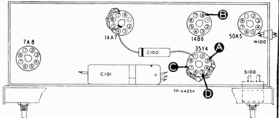
**Figure 1. Bottom View, Showing Section 1 Test Points**
