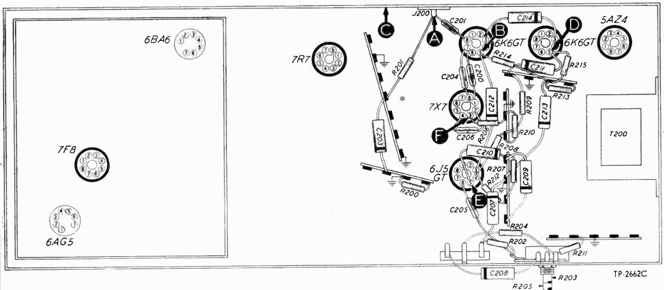
FIGURE 4. BOTTOM VIEW, SHOWING SECTION 2 TEST POINTS.
