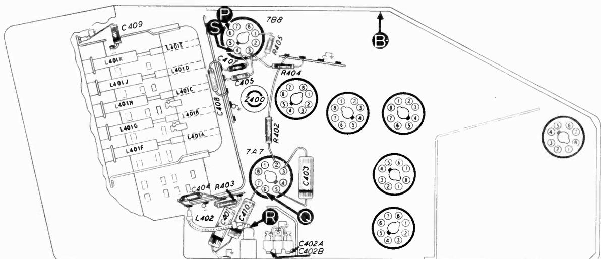
Figure 8. Bottom view, showing Section 4 test points.
