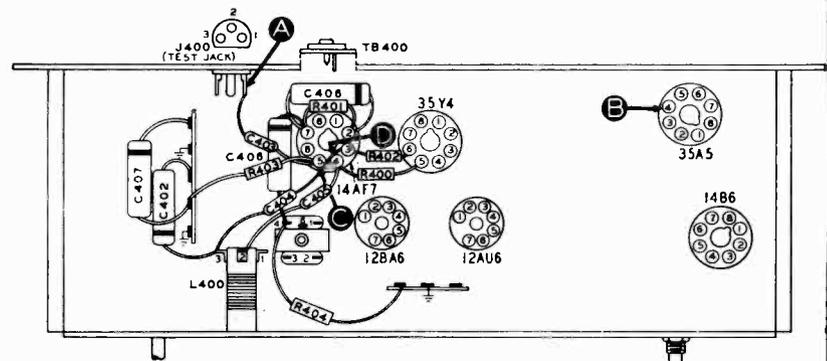
Figure 4. Bottom View, Showing Section 4 Test Points
