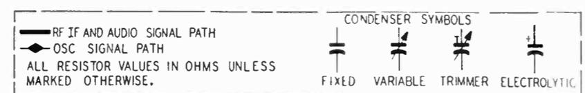
NOTE: ALL VOLTAGES AND CAPACITY AND RESISTANCE VALUES SHOWN ARE AVERAGE. THE VOLTAGES BETWEEN TEST POINT B AND OTHER POINTS INDICATED WERE MEASURED WITH A 20,000-OHMS-PER-VOLT METER VOLUME CONTROL AT MINIMUM AND TUNING CONDENSER PLATES FULLY MESHED.
