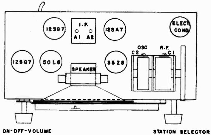
This Model is a 5 tube, 1 Band super-heterodyne with a built in Regaloop Antenna. The tuning range of the Broadcast Band is 540 to 1650 kilocycles or 560 to 182 meters. This receiver operates on 105-125 volts, 50-60 cycles alternating current or on 105-125 volts direct current.
