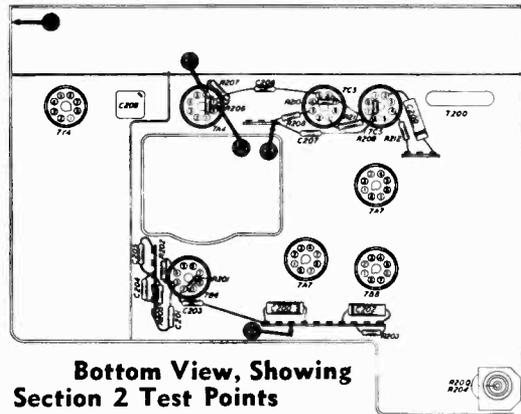
Bottom View, Showing Section 2 Test Points
