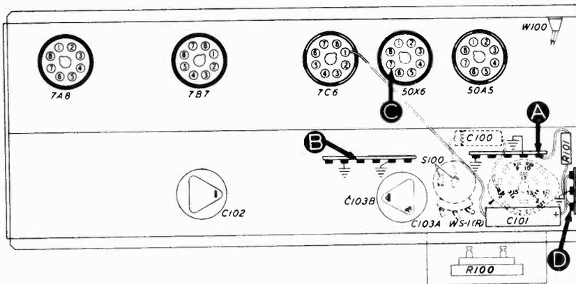
Figure 1. Bottom View, Showing Section 1 Test Points
