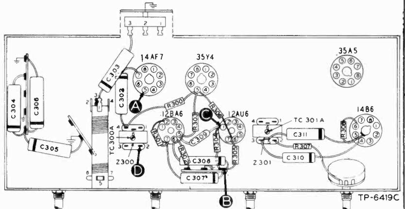
**Figure 3. Bottom View, Showing Section 3 Test Points**
