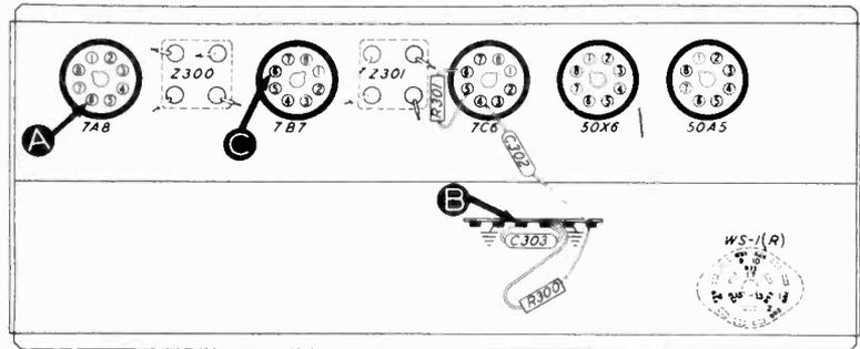
**Figure 3. Bottom View, Showing Section 3 Test Points**
