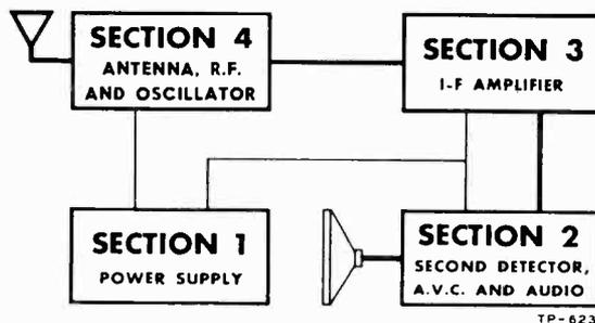
Figure 1. Block diagram (Heavy lines indicate signal path.)
