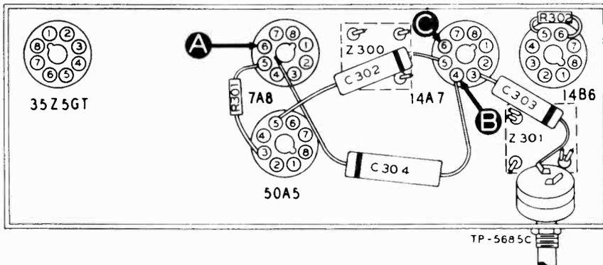
**Figure 3. Bottom View, Showing Section 3 Test Points**
