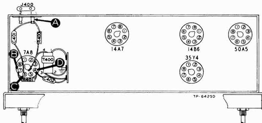
**Figure 4. Bottom View, Showing Section 4 Test Points**
