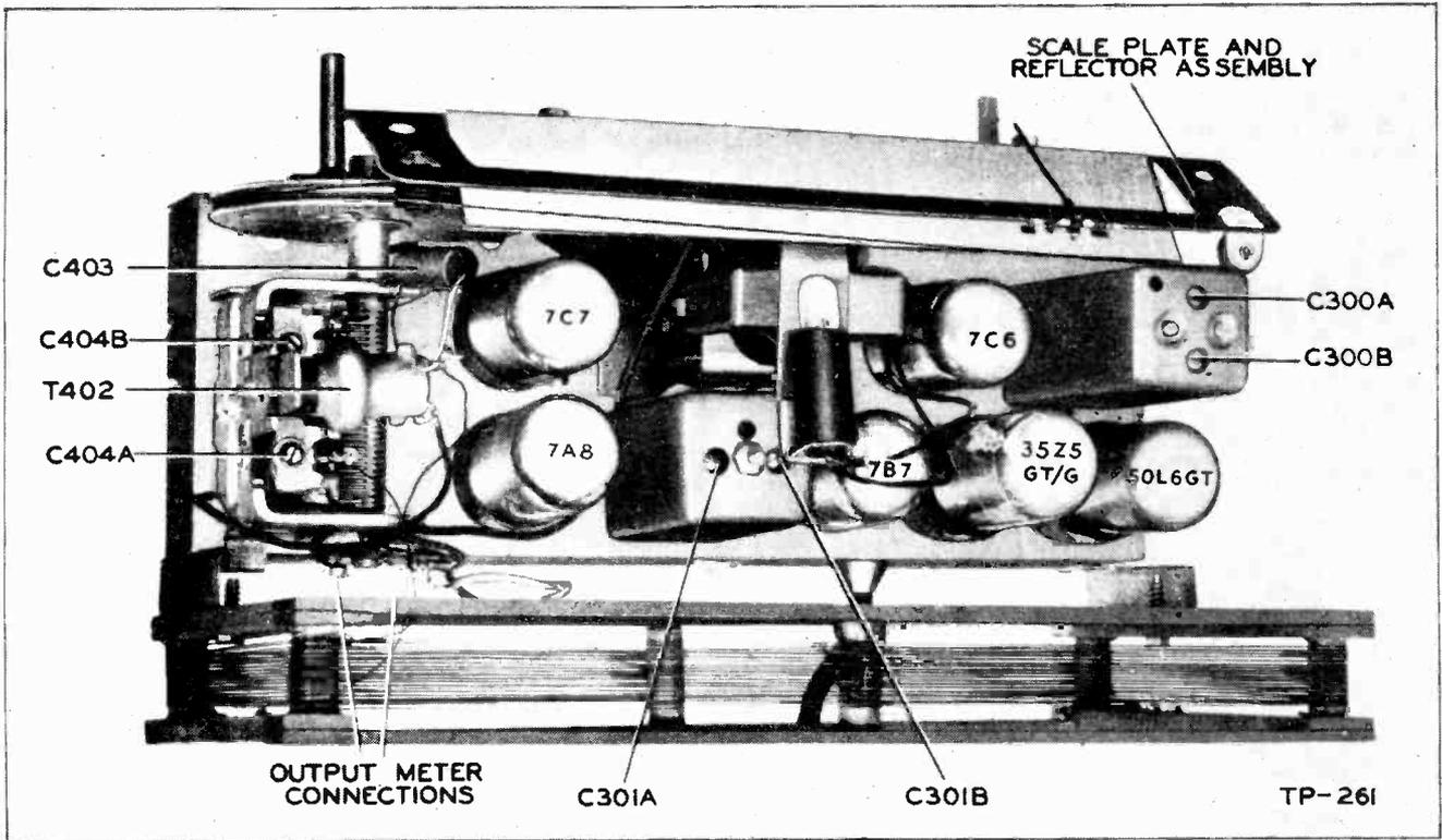
Figure 11. Top view showing trimmer condenser locations.
