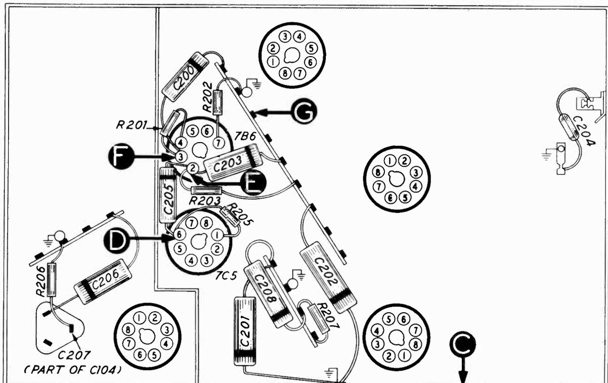
Figure 6. Bottom view, showing Section 2 test points.
