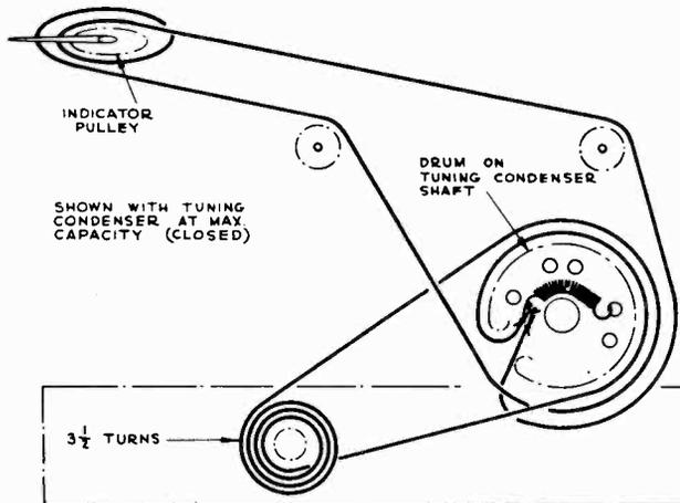
Dial Indicator and Drive Mechanism DC51
