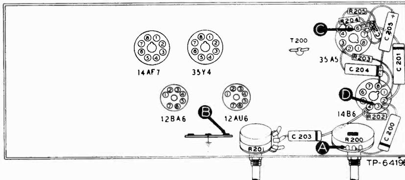
Figure 2. Bottom View, Showing Section 2 Test Points
