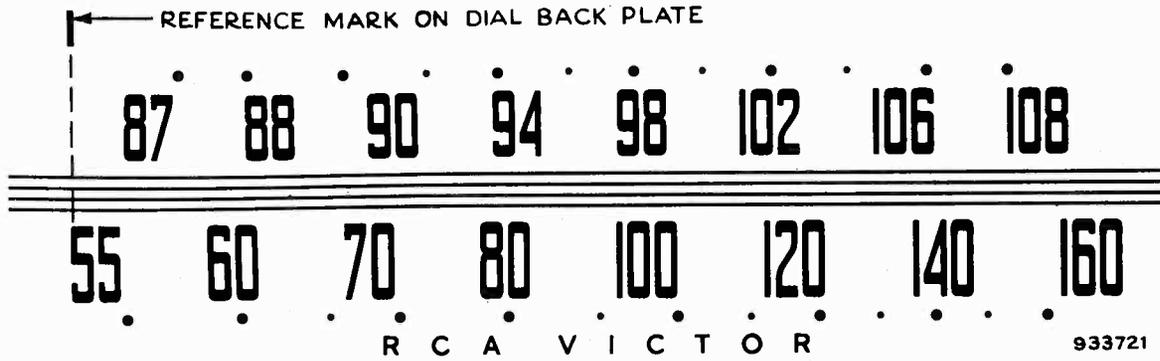
The dial scale drawing shown is a full size reproduction. It can be used as a reference in alignment procedure.
