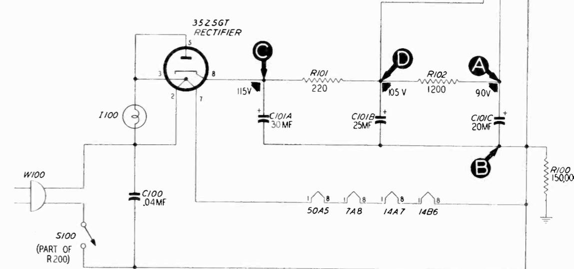
Figure 5. Philco Radio Model 49-503, Sectionalized Schematic Diagram, Showing Test Points
