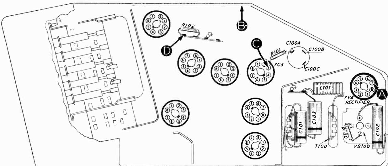
Figure 2. Bottom view, showing Section 1 test points.
