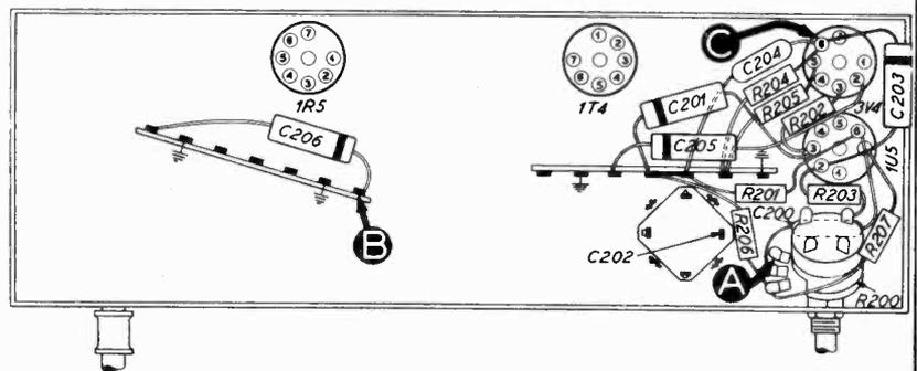
Figure 2. Bottom View, Showing Section 2 Test Points
