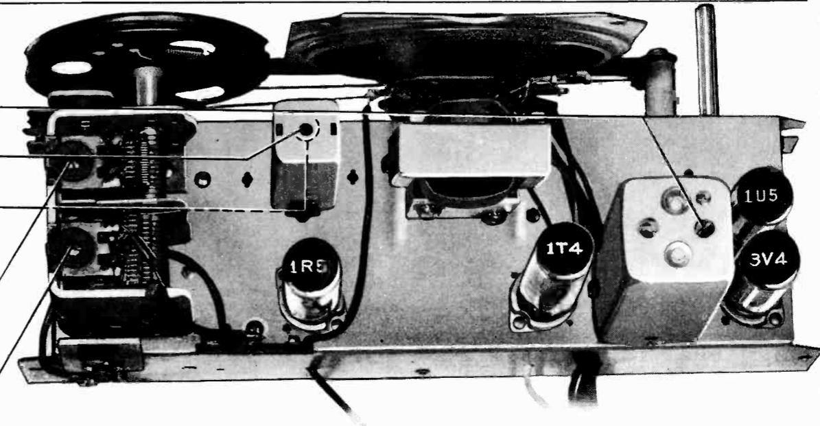
Figure 6. Top View, Showing Trimmer Locations
