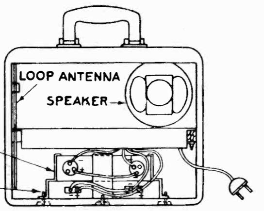
REAR VIEW OF CABINET SHOWING BATTERIES IN PLACE
