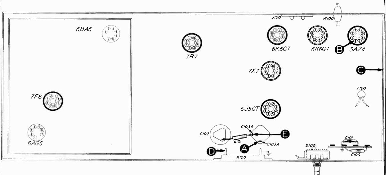
Figure 3. Bottom View, Showing Section 1 Test Points
