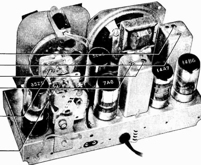
FIGURE 6. TOP VIEW, SHOWING TRIMMER LOCATIONS
