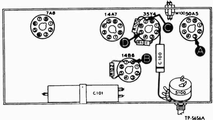
Figure 1. Bottom View, Showing Section 1 Test Points
