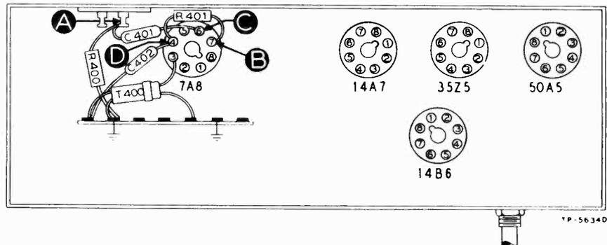
FIGURE 4. BOTTOM VIEW, SHOWING SECTION 4 TEST POINTS
