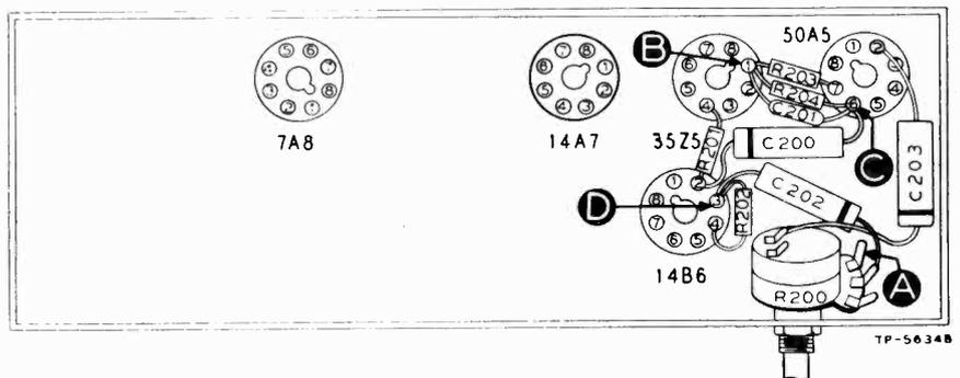
FIGURE 2. BOTTOM VIEW, SHOWING SECTION 2 TEST POINTS
