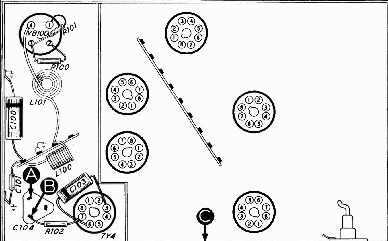
Figure 4. Bottom view, showing Section 1 test points.
