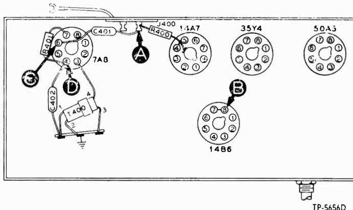
Figure 4. Bottom View, Showing Section 4 Test Points
