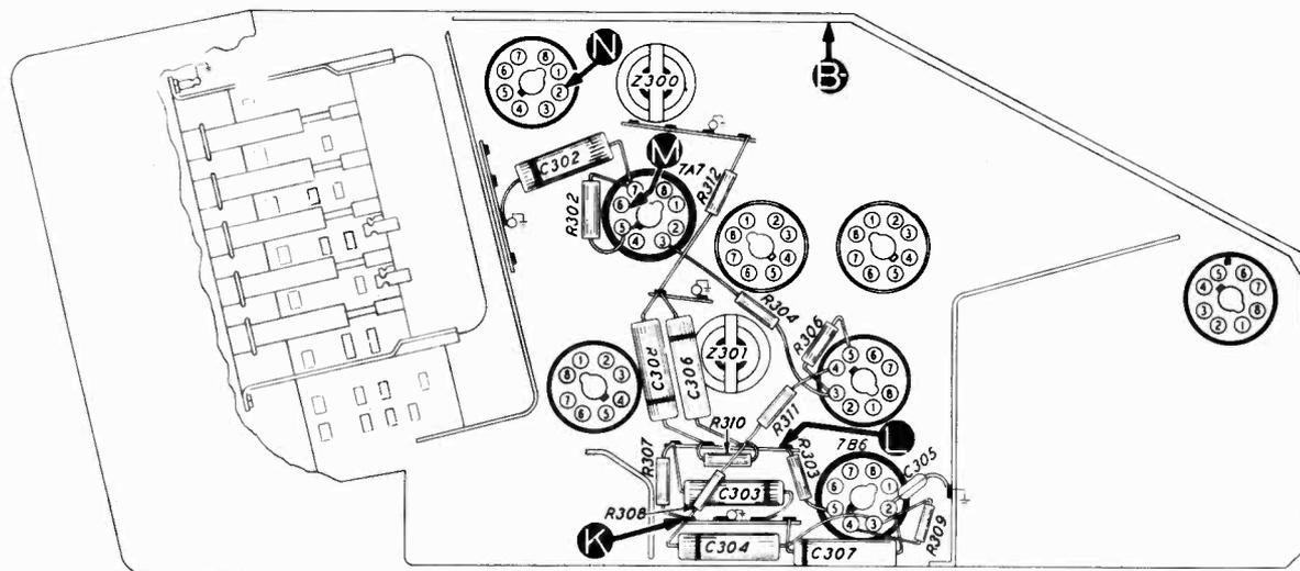
Figure 6. Bottom view, showing Section 3 test points.
