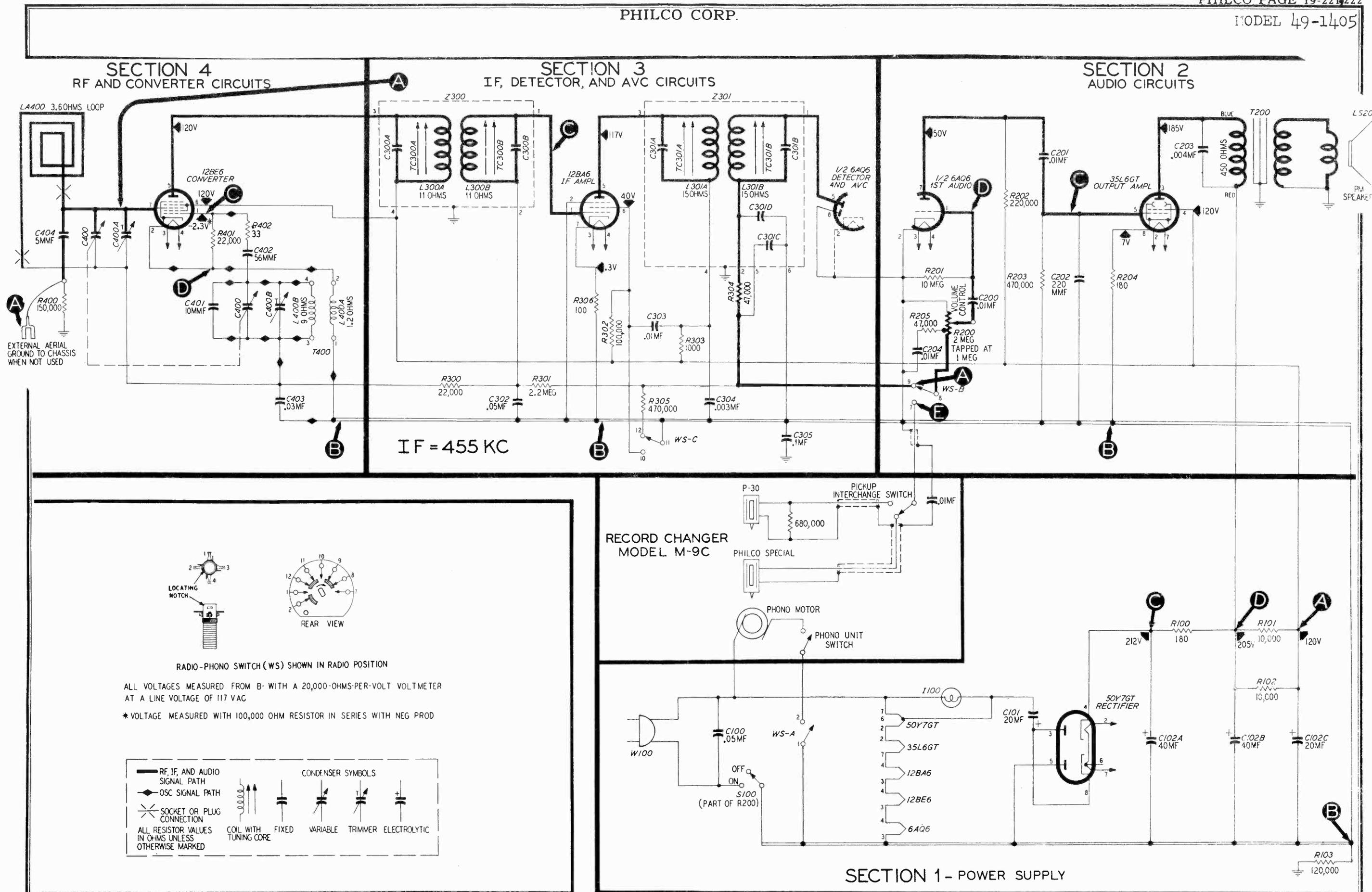
Figure 5. Philco Model 49-1405, Sectionalized Schematic Diagram, Showing Test Points
