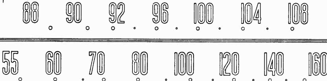
The dial scale drawing shown is a full size reproduction. It can be used as a reference in alignment procedure.
