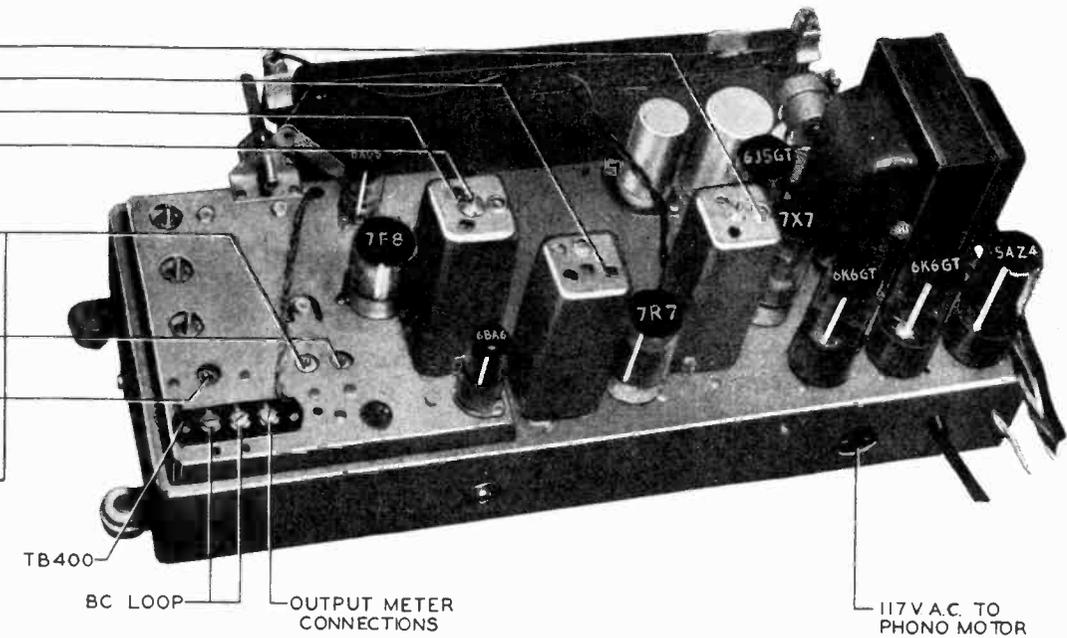
Figure 8. Top View, Showing AM Trimmer Locations
