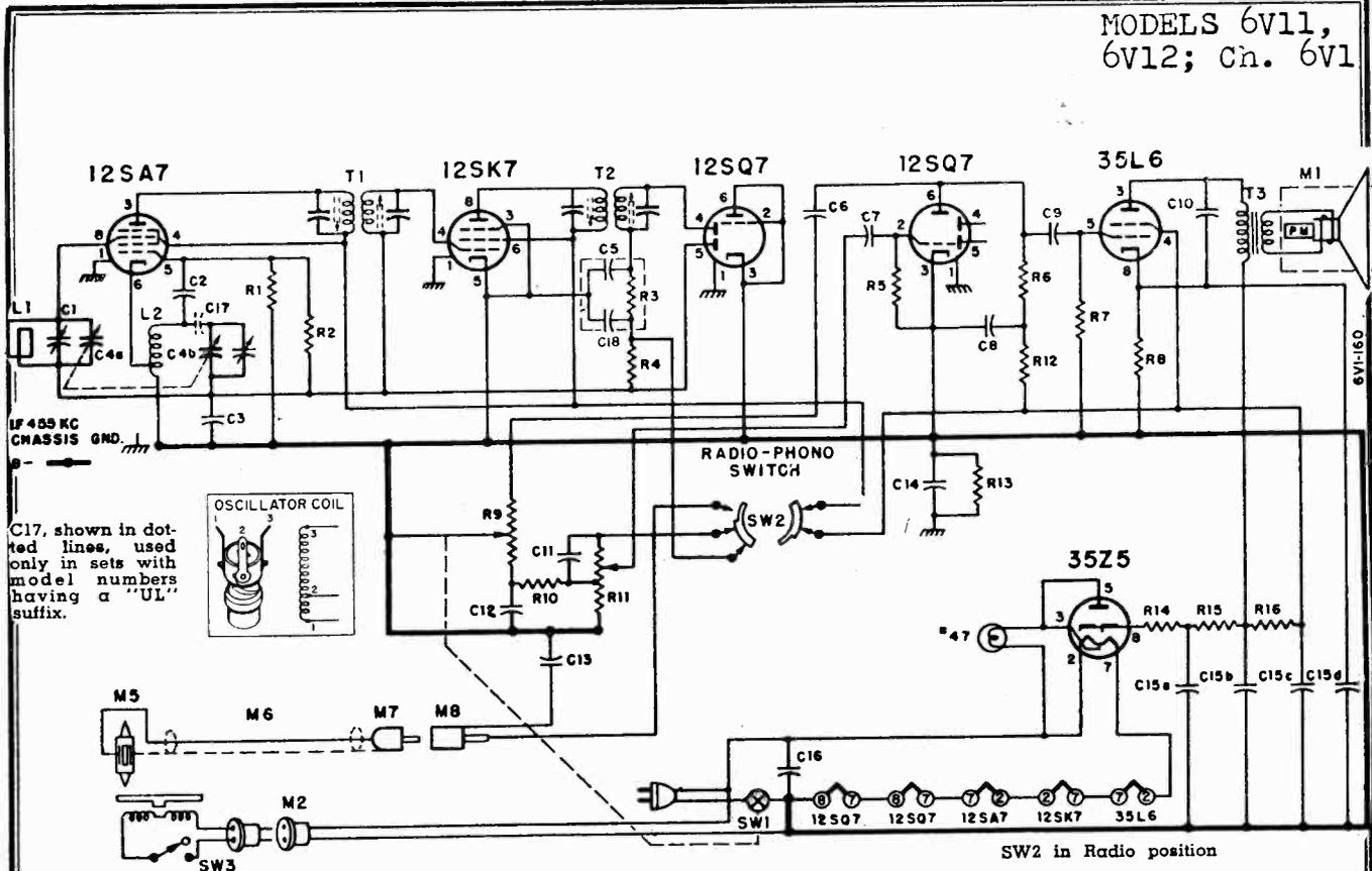
C17, shown in dotted lines, used only in sets with model numbers having a "UL" suffix.
