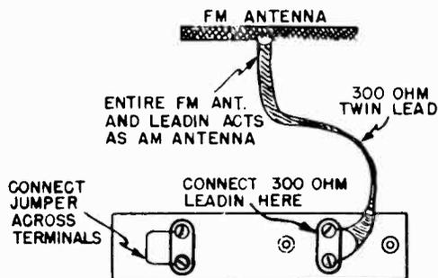
CONNECTIONS WHERE 300 OHM FM ANTENNA IS TO BE
