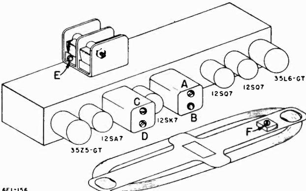
Adjustments B and D made from underside of chassis.
