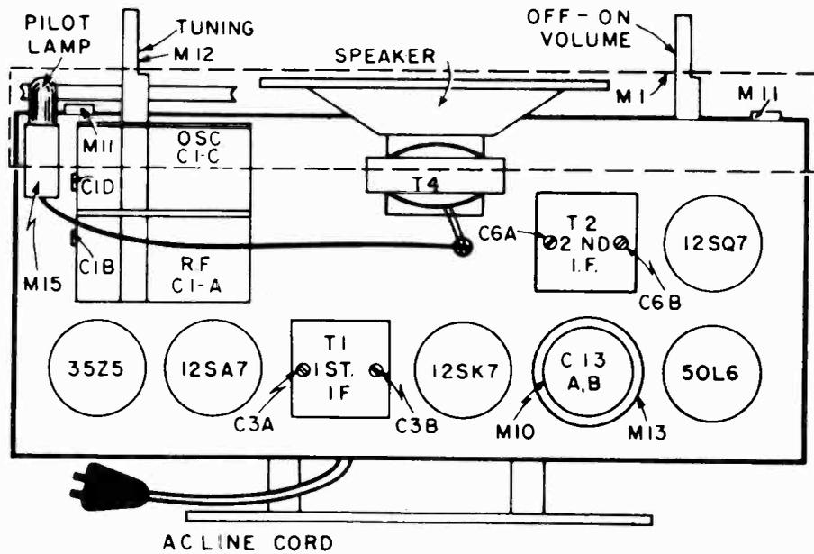
NOTE: In the O-1 chassis the positions of the electrolytic capacitor (C13a, b) and 2nd IF transformer (T2) are reversed.
