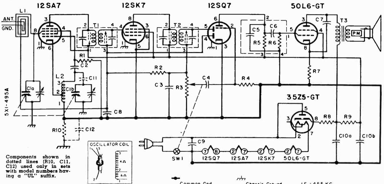
Components shown in dotted lines (R10, C11, C12) used only in sets with model numbers having a "UL" suffix.
