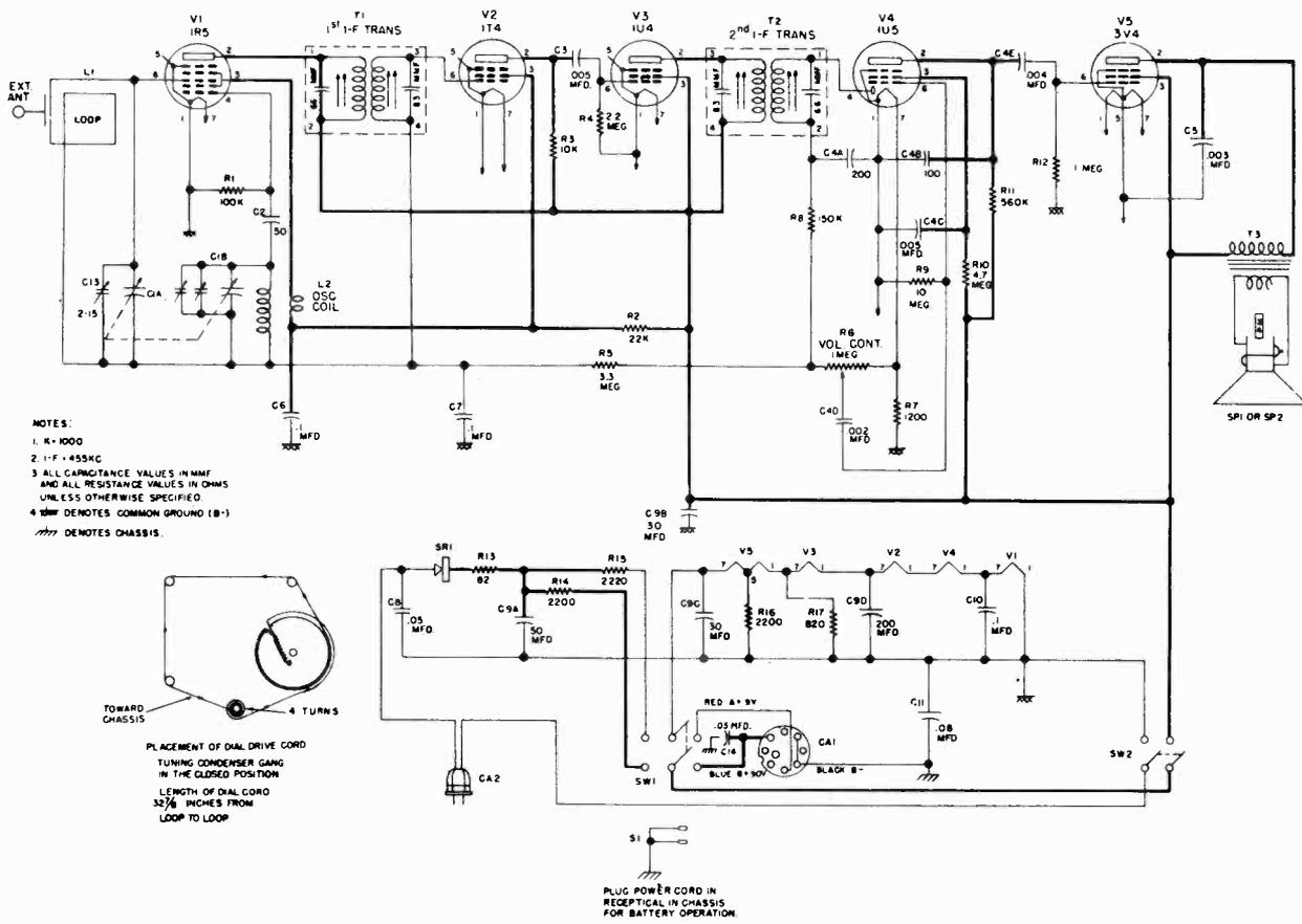
SCHEMATIC DIAGRAM — MODEL 10-307M
