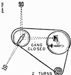
Dial stringing and pointer with solid lines shown with gang closed. Dashed line pointer positions (1400 KC and 900 KC) shown when tuning condenser is tuned to generator signal.
