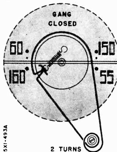
With gang fully closed, set pointer in horizontal position.
