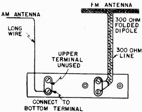
CONNECTIONS FOR SEPARATE ANTENNAS WHERE
