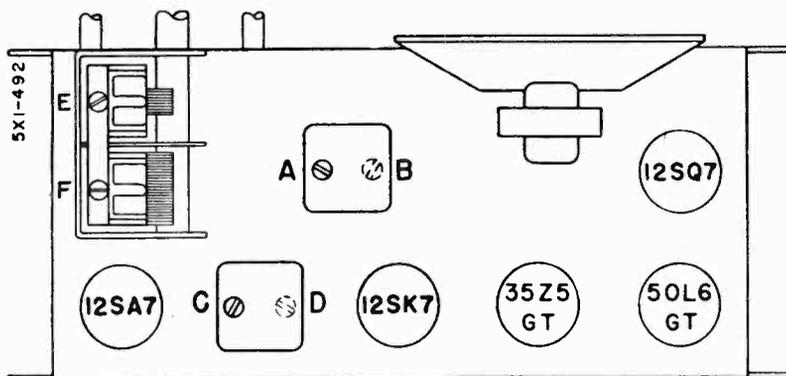
Adjustments B and D are made from underside of chassis.
