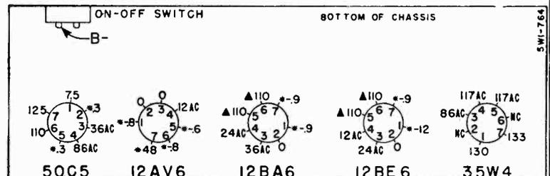
\* If taken with a 1000 ohm-per-volt meter, readings will be either lower or practically zero.
