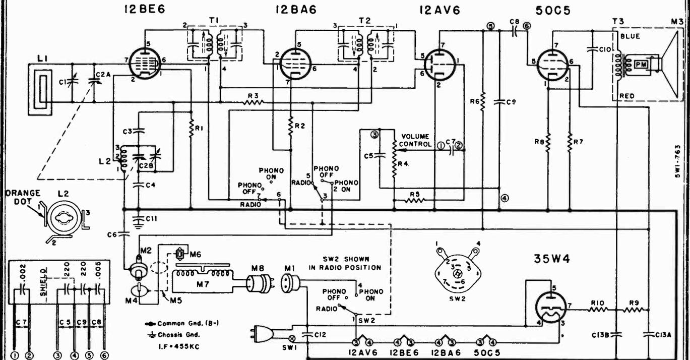
For models ending in "UL", a .05 mfd, 400 V, condenser is wired between terminal 3 of L2 and stator of C2B.
