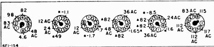
\* If taken with a 1000 ohm-per-volt meter, readings will be either lower or practically zero.
