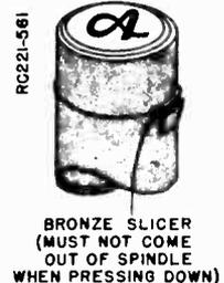
1. Place the 45 RPM Spindle in the hole in the center of the turntable and turn it so that "lock-in lugs" fall into slots in the turntable (do not lock the lugs into the turntable).
