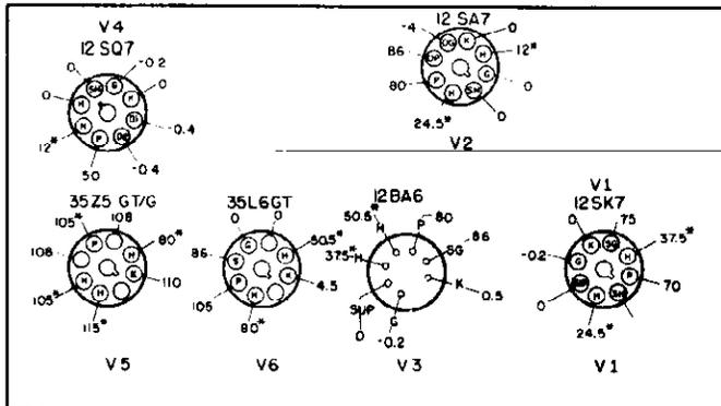
117 VOLTS AC LINE, NO SIGNAL INPUT.
