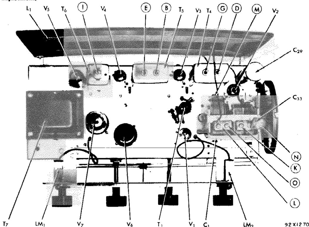
Fig. 5. Top view, alignment, adjustments and component location.
