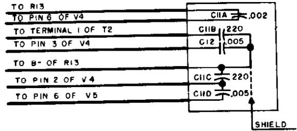
Fig. 2. Connections for Capacitor RCW-3015
