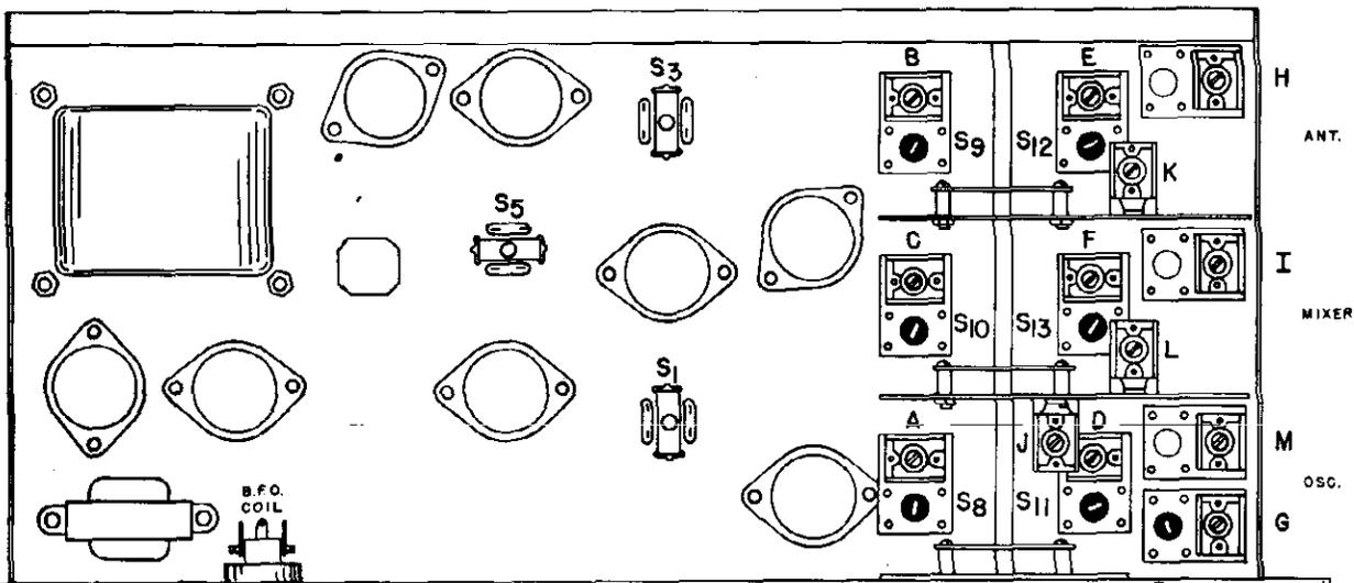
Fig. 3. Bottom view, alignment points
