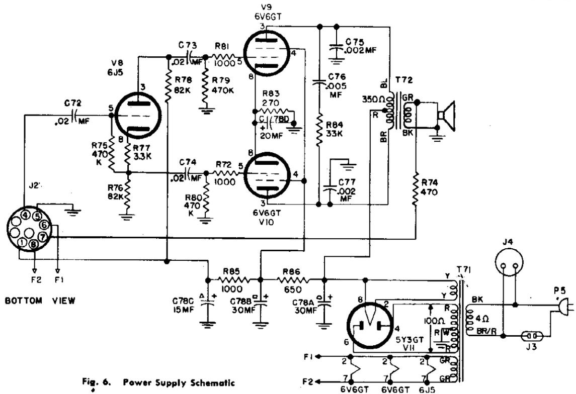
Fig. 6. Power Supply Schematic
