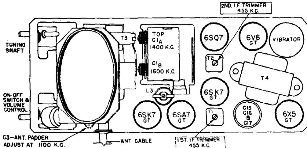
Figure 6 Tube & Trimmer Locations 43-5006B & 43-5006C
