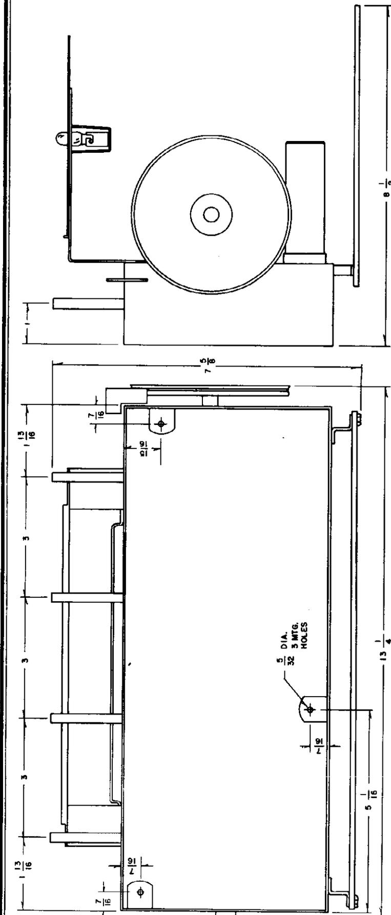
Fig. 8. Chassis mounting dimensions
