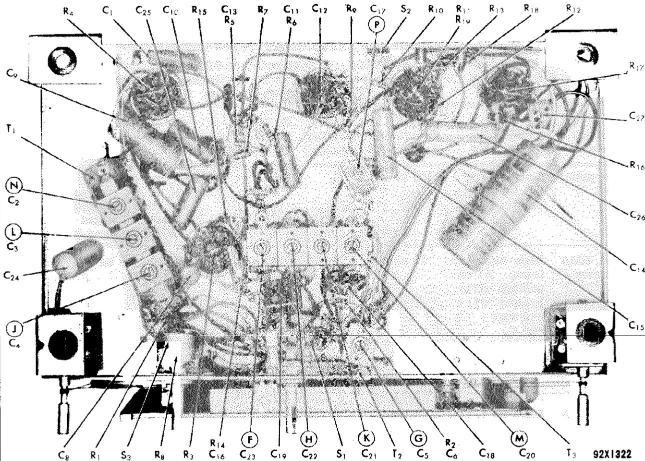
FIG. 9. BOTTOM VIEW, ALIGNMENT POINTS AND COMPONENT LOCATIONS
