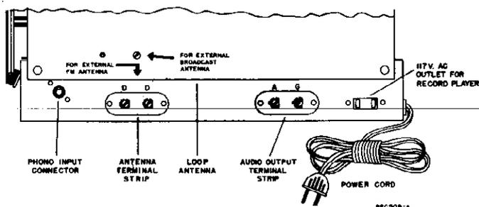
Fig. 3. Antenna & record player connections
