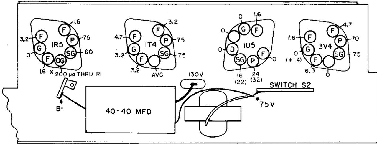
VOLTAGES MEASURED WITH 20,000Ω/VOLT METER TO B-; NO RF OR IF SIGNAL, SET OPERATING FROM 60 ~ 120 VOLT LINE.
