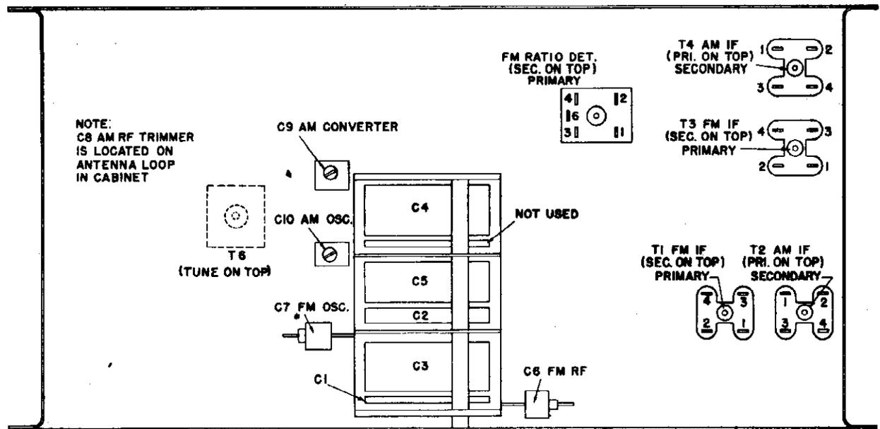
Figure 2. Trimmer Condenser Location - Bottom View
