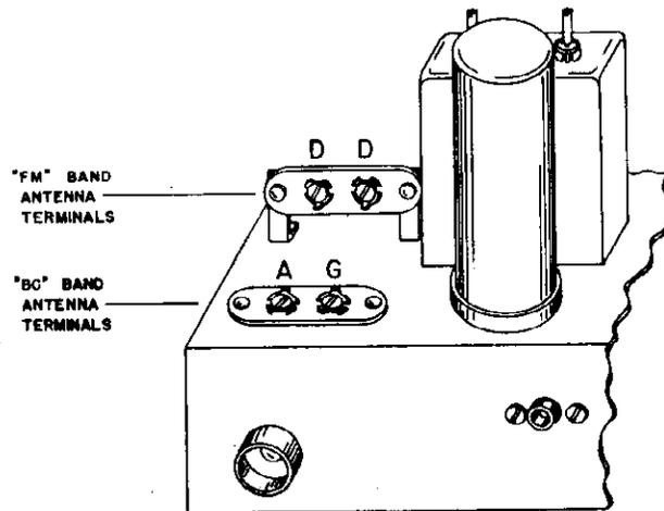
Fig. 2. Antenna terminal strip connections
