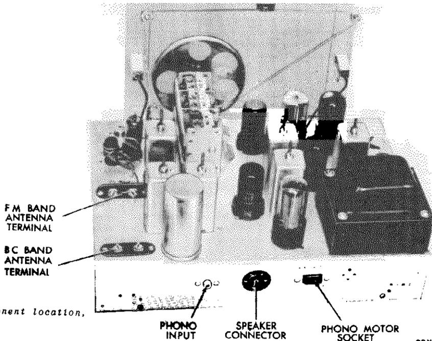
Fig. 4. Component location, rear view
