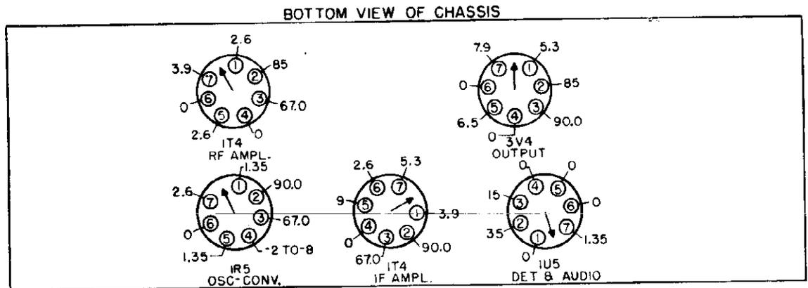
DC VOLTAGES TO B- UNLESS OTHERWISE SPECIFIED. ALL ALL RATINGS ARE A.G. OPERATION MEASURED WITH REFERENCE TO B-. VOLTAGE IS MEASURED WITH 20,000 OHMS PER VOLT METER.
