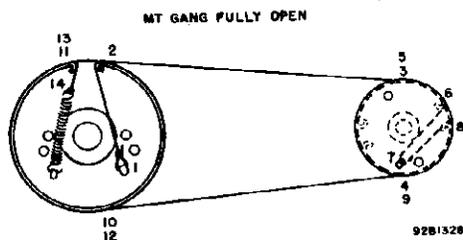
**FIG. 5. MAIN TUNING GANG DRIVE STRINGING PROCEDURE**
