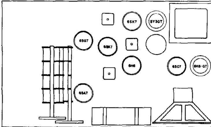
Fig. 7. Top view, location of tubes and dial lamps 92D1132
