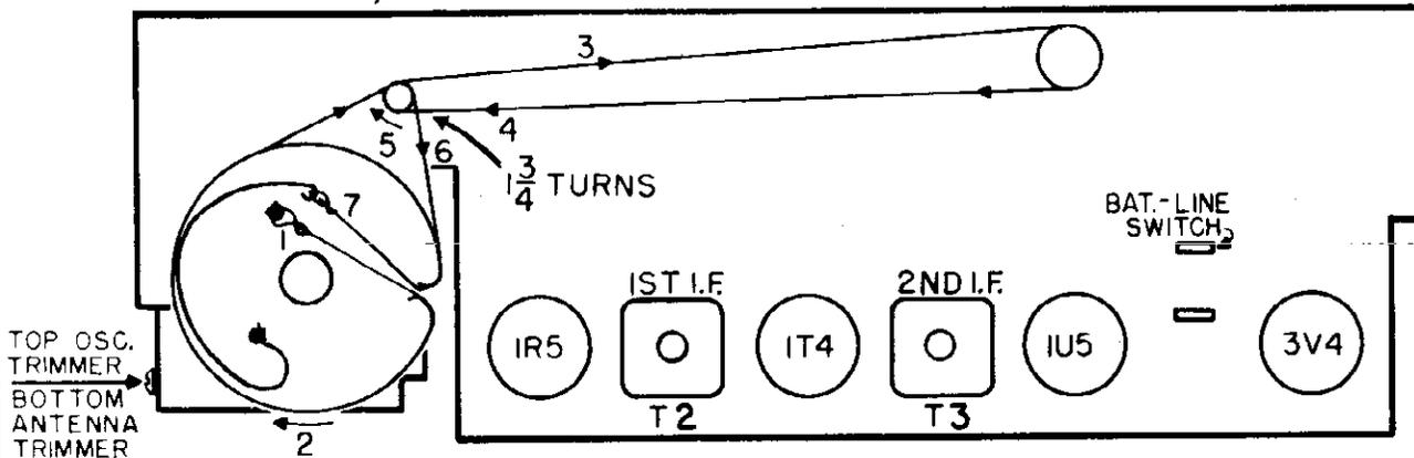
Fig. 4. Dial Stringing and Tube and Trimmer Location
