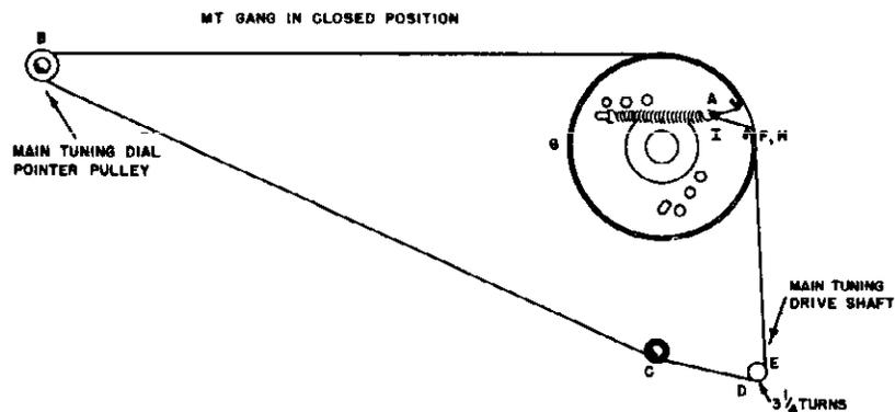
FIG. 4. MAIN TUNING DIAL POINTER DRIVE STRINGING PROCEDURE
