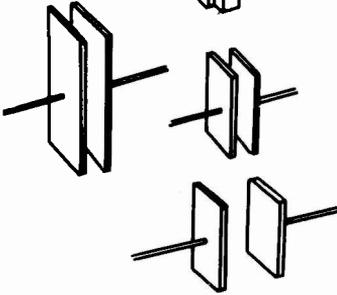
**FACTORS OF CAPACITANCE** — Plate area, the distance between the plates and the dielectric material determine capacitance.
