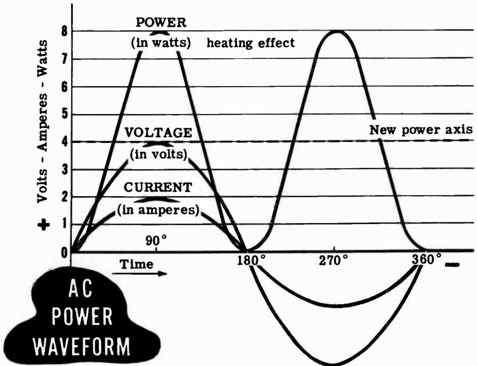
The power used in an AC circuit is the average of all the instantaneous values of power or heating effect for a complete cycle. To find the power, all of the corresponding instantaneous values of voltage and current are multiplied together to find the instantaneous values of power, which are then plotted for the corresponding time to form a power curve. The average of this power curve is the actual power used in the circuit.
