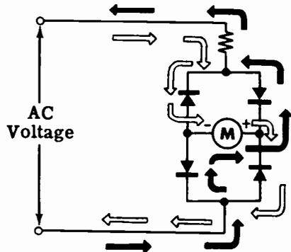
Because the meter reading is the average of the half-cycle current pulses, the scale is not the same as that used for DC. Although the amount of deflection is a result of average current flow through the meter movement, the scale is calibrated to read effective values of voltage.
