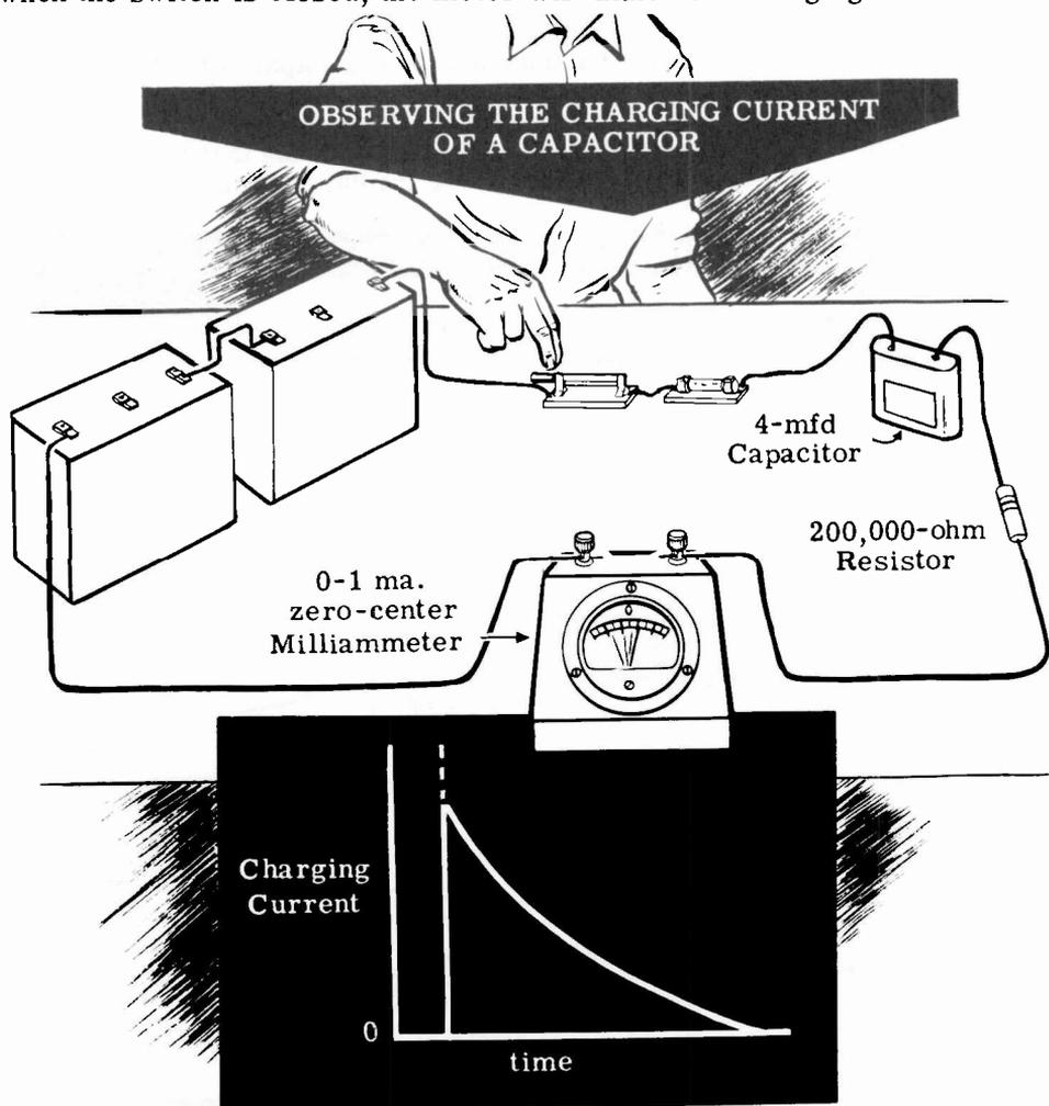
Substituting capacitors having various values, the instructor shows that the current flow lasts longer when charging larger capacitors. Notice that, for small values of capacitance, the time required to charge them is so short that it is difficult to read the current indicated on the meter.
