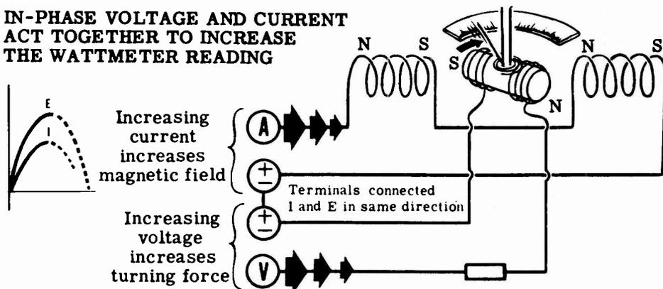
If the current lags the voltage, the meter field does not increase at the same time as the moving coil current. This results in less turning force on the wattmeter pointer. The power indicated then is less than with in-phase voltage and current of the same magnitude.
