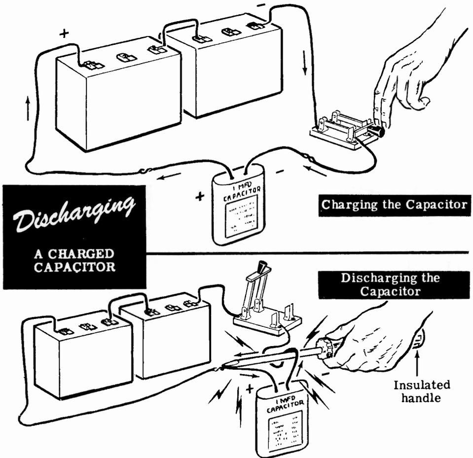
As the instructor repeatedly charges and discharges the capacitor, you see that the resulting arc is the same each time. This shows that the charge left in a capacitor when the circuit voltage is removed is always maximum in a DC circuit. **CAUTION:** Never discharge a capacitor while it is connected to the circuit voltage, whether the voltage source is a battery or AC power line.
