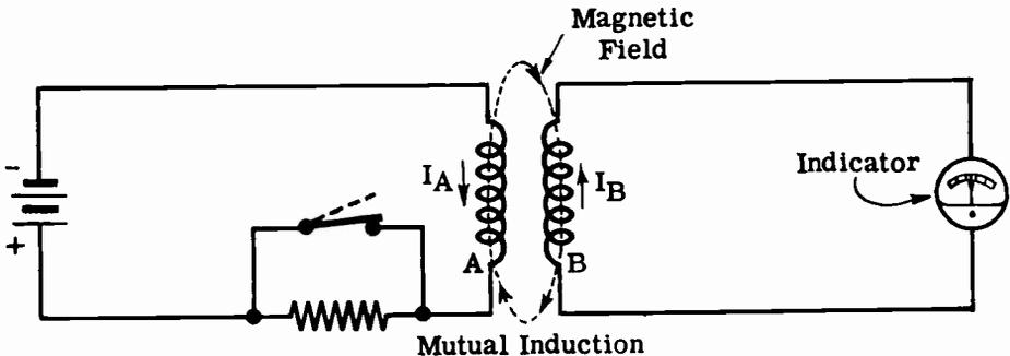
A battery is used in the above diagram as a source of emf. The only way current variations can be developed, then, is by the opening or closing of the switch. If an AC voltage source with an extremely low frequency (one cycle per second) is used to replace the battery, the indicator shows continuous variations in current. The indicator needle moves to the left (or right) first, and then reverses its position, to show the reversal in AC flow.
