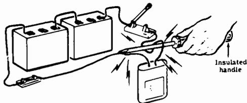
**CAPACITOR DISCHARGE** — Flow of electrons from the negatively charged plate of a capacitor to the positively charged plate, eliminating the charges on the plate.
