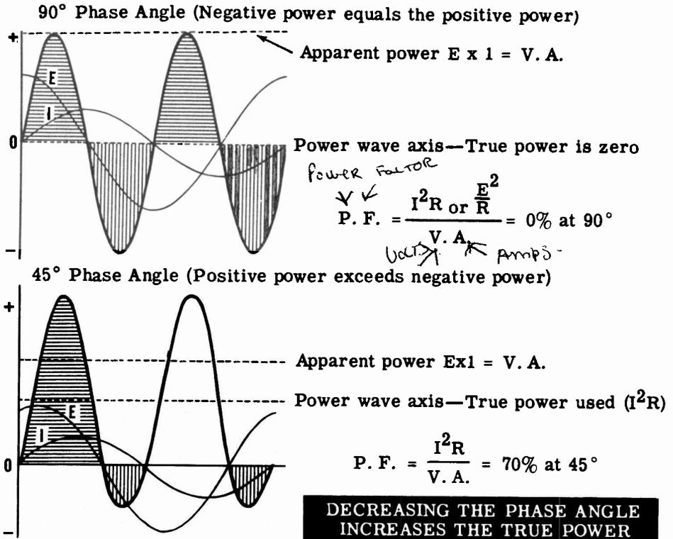
The average value of actual power, called "true power," is represented by an axis drawn through the power wave halfway between the opposite maximum values of the wave. As the phase angle increases, this axis moves nearer to the axis for voltage and current. In AC circuits the apparent power is found by multiplying the voltage and current just as in DC circuits (Apparent power = Voltage x Current). When apparent power is divided into true power, the resultant decimal is the power factor.
