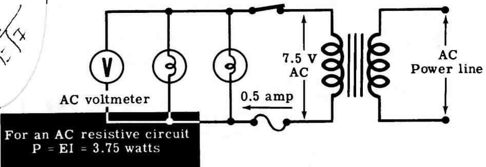
Next the battery is disconnected and the DC voltmeter is replaced with an AC meter of the same range. The 6.3-volt transformer is used as an AC voltage source, and you see that the lamps light as brightly as they did in the DC circuit. Notice that the voltmeter reading is almost the same as that obtained using DC, about 7.5 volts.
