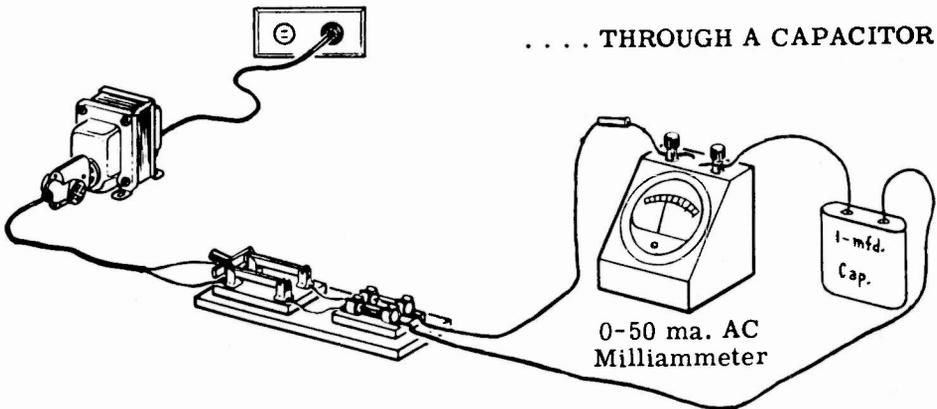
To prove that capacitors appear to block DC but permit AC to pass, the instructor sets up the circuit shown to the right. When DC is applied the lamp will not glow and a DC voltmeter across the lamp will read zero volts. When AC is applied the lamp will glow and an AC voltmeter across the lamp will give a reading.
