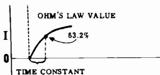
**INDUCTIVE TIME CONSTANT** — The ratio of L to R which gives the time in seconds required for the circuit current to rise to 63.2 percent of its maximum value.
