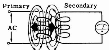
**TRANSFORMER ACTION** — The method of transferring electrical energy from one coil to another by means of an alternating magnetic field. The coil which generates the magnetic field is called the primary, and the coil in which the voltage is induced is called the secondary. The voltage induced in the secondary depends upon the turns ratio between the secondary and primary.
