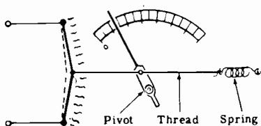
**HOT-WIRE AMMETER** — Meter movement based on the expansion of a wire heated by current flow through it. Used only to measure current.
