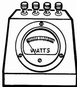
Remember that the power formula ( $P = EI$ ) can be used to find the power used in a resistive AC circuit, provided effective values of  $E$  and  $I$  are used.
