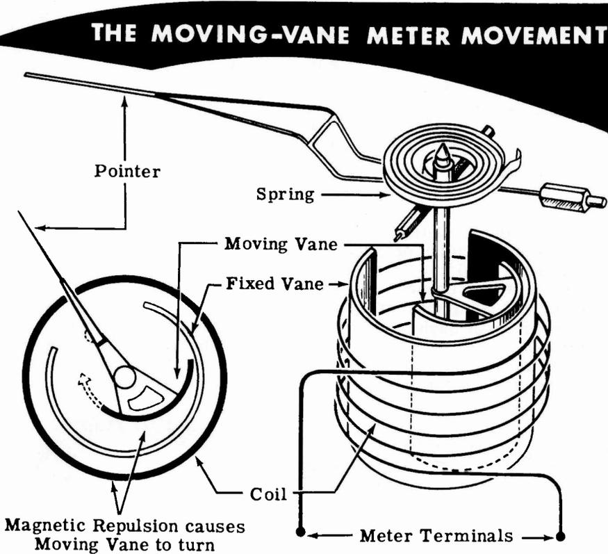
Moving-vane meters may be used for voltmeters, in which case the field coil consists of many turns of fine wire which generate a strong field with only a small current flow. Ammeters of this type use fewer turns of a heavier wire, and depend on the larger current flow to obtain a strong field. These meters are generally calibrated at 60 cycles AC, but may be used at other AC frequencies. By changing the meter scale calibration, moving-vane meters will measure DC current and voltage.
