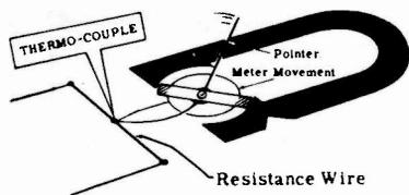
**THERMO-COUPLE AMMETER** — Meter movement utilizing the heat of a resistor through which current flows to develop a measurable current in a thermo-couple.
