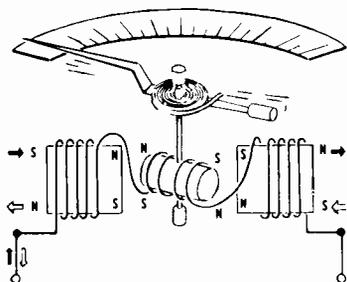
**ELECTRODYNAMOMETERS** — Commonly used in wattmeters rather than voltmeters and ammeters. Basic principle is identical to that of a D'Arsonval movement except that field coils are used instead of a permanent magnet.
