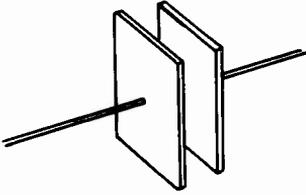
**CAPACITOR PLATES** — Metallic or metalized plates which can be charged.
