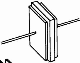
**DIELECTRIC** — Insulating material between the plates of a capacitor.
