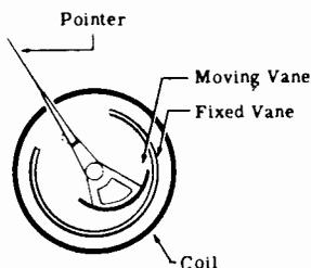
**MOVING-VANE METER** — Meter which operates on magnetic repulsion principle, using one movable and one fixed vane. Can be used on AC or DC to measure either voltage or current.
