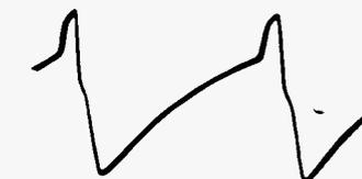
Figure 15. Waveform on Grid Pin 1 of V403 With Sync Pulse.
