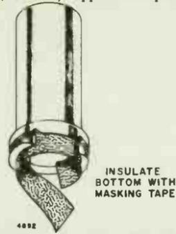
Figure 35. Special Tube Shield for IF Amplifier Alignment and IF Response Curve Check.
