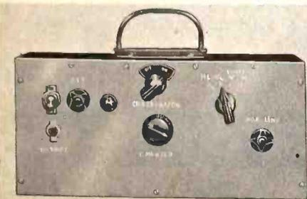
Fig. 1. Photograph of cross-bar TV test pattern generator.
