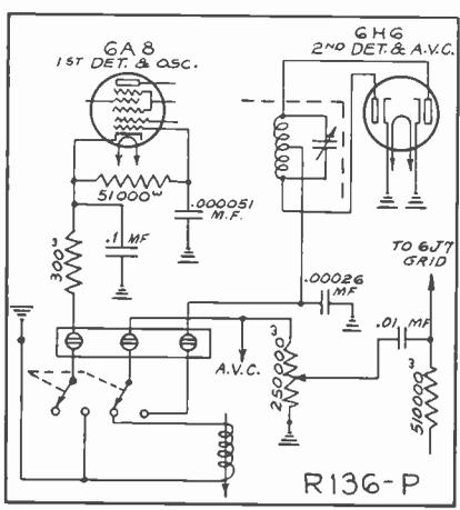
Schematic diagram of the Stewart Warner R-136-P chassis with phonograph pickup indicated.
