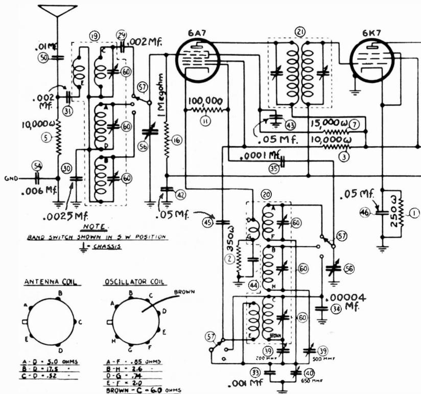
Fada Model 1463 is the revised Model 1462. This schematic shows the partial circuit for the new 1463, which is for three wavebands.
