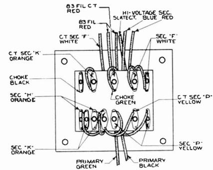
Connections to the new power transformer used in the Silvertone 1640
