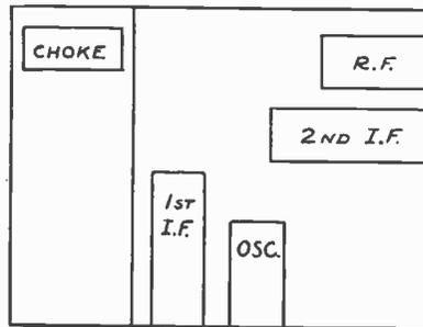
Location of essential parts on under side of chassis for aligning.
