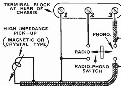
Fig. 3. When turntable is used near the receiver, the setup above is employed.
