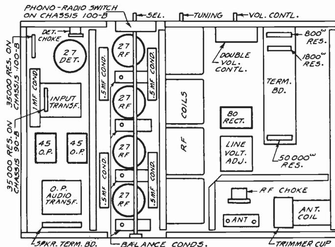
Chassis layout for Majestic Chassis 90-B and 100-B. Note the different positions of the 35,000-ohm resistor and the addition of the phono-radio switch for Chassis 100-B
