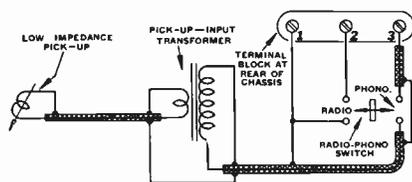
Fig. 2. Setup used when turntable is used at some distance from the receiver.
