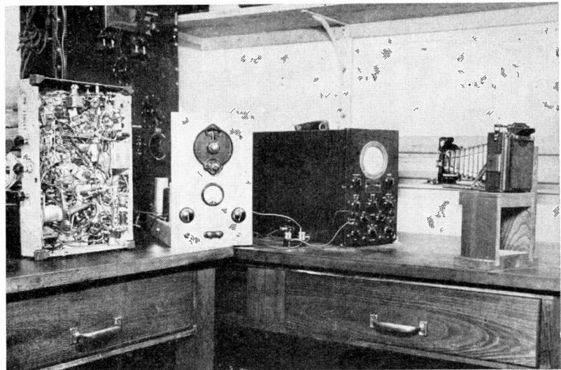
The arrangement for photographing oscillograms in the author's *Successful Servicing Laboratory*
