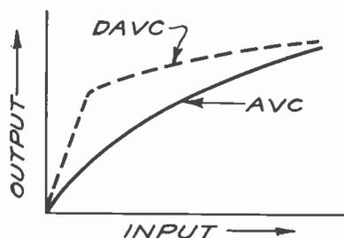
Fig. 4. The difference between receiver output with an avc system and one with davg action is easily seen by comparing the two curves above.
