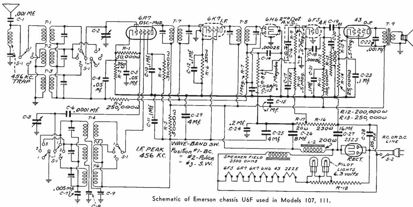
Schematic of Emerson chassis U6F used in Models 107, 111.
