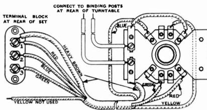
Fig. 1. Switch connections for phonograph.
