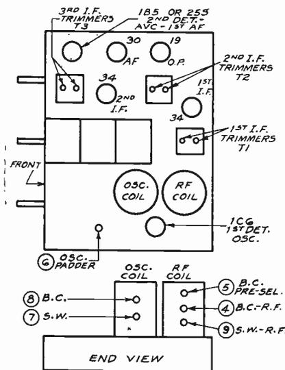
The trimmers on the Fairbanks-Morse Model 64 Battery set are identified by number corresponding to the table below
