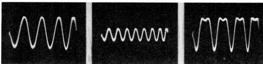
The 1000-cycle sine wave, Fig. 4, left, and the 2000-cycle wave, Fig. 5, were combined. The resultant asymmetrical wave of Fig. 6 shows the presence of the second harmonic
