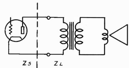
Fig. 2. In this output circuit  $Z_s$  is the impedance of the tube and  $Z_L$  is the load impedance, represented by the transformer and voice coil of the speaker.
