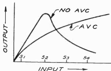
Fig. 1. Variation of output with signal input of sets with and without avc.
