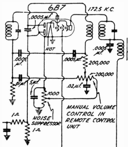
Fig. 6. An example of reflexing in the second detector of a superheterodyne, where the 6B7 is also an i-f. amplifier and controls the a.v.c.
