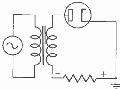
Fig. 1. The basic circuit of a half-wave rectifier tube. Note polarity of resistor.
