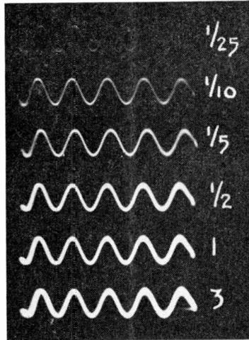
The results of different exposures of the same sine wave with constant image intensity
