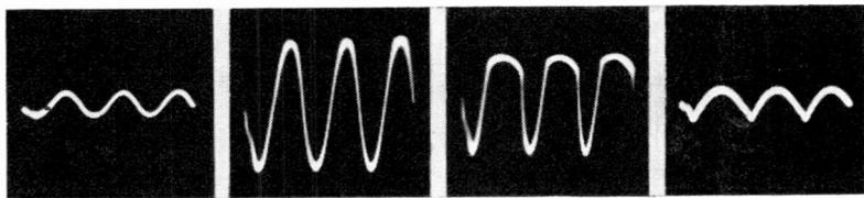
Figs. 2A, 2B, 2C and 2D, left to right. These oscillograms correspond with the four points designated along the horizontal axis of Fig. 1, and represent the demodulator output for a receiver not equipped with avc. The distorted output shown in Figs. 2C and 2D is due to overload and represents input in excess of S<sub>2</sub> in Fig. 1.
