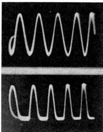
Fig. 2, above. The sine wave of a voltage applied to the transformer primary of Fig. 1. Fig. 3. With the oscillograph connected across the resistor, the rectified current wave was obtained.
