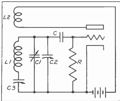
Typical oscillator circuit, showing trimmer C2 and padder C3
