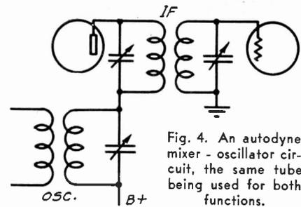
Fig. 4. An autodyne mixer - oscillator circuit, the same tube being used for both functions.
