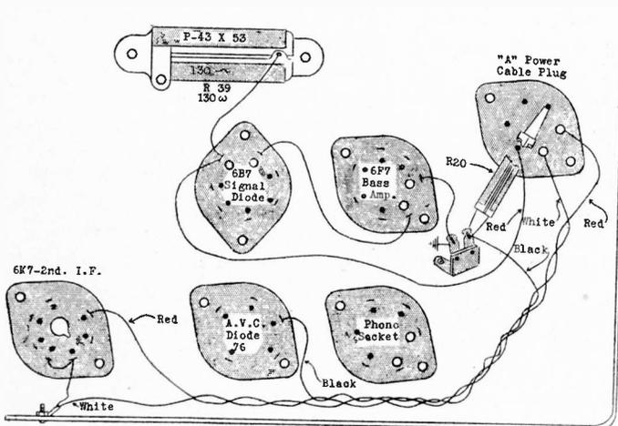
Fig. 1. On the left is shown the tube sockets and cable plug of the radio-frequency chassis of the Wells-Gardner 6F Series with the revised heater wiring, as explained in the accompanying text
