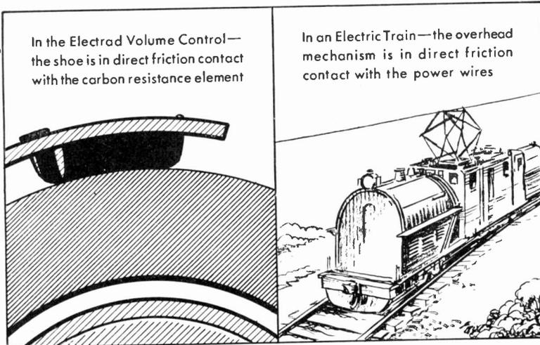
In the Electrad Volume Control—the shoe is in direct friction contact with the carbon resistance element
