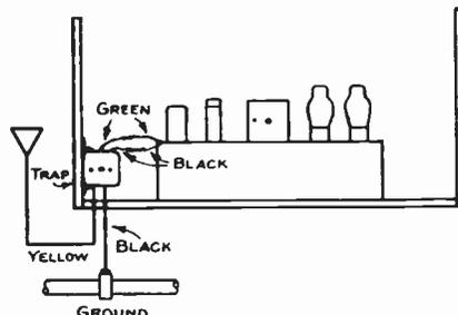
Installation of wave-trap in various Silvertone chassis
