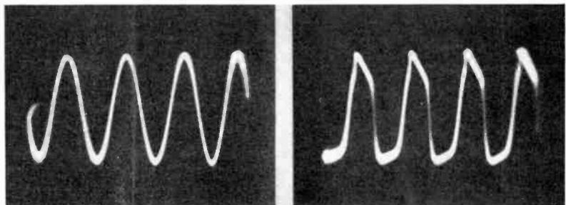
Compare the sine wave of Fig. 2, left, with the complex wave of Fig. 3 and note the differences in symmetry and regularity
