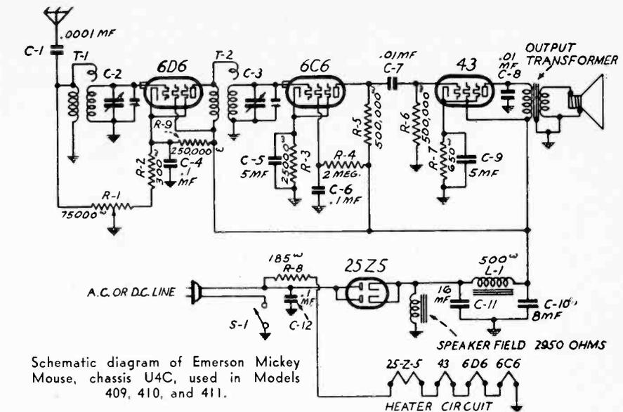
the antenna and adjust both trimmers on the variable condenser for maximum response. Use as weak a signal as possible.
