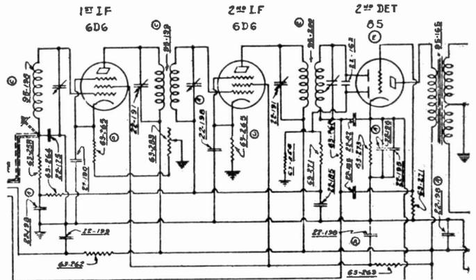
A 0.0001-mf. condenser, Part No. 22-162, was inserted between the diode plates of the 85 2nd detector and the wiring changed, as shown in the accompanying schematic. The 490,000-ohm resistor, Part No. 63-258, was connected between the lower diode plate and ground. Note other changes in the AVC wiring.
