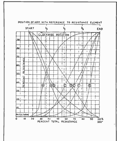
*Above chart shows standard control tapers. Curves H and C are recommended for Antenna-Cathode circuits.*
