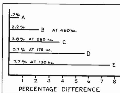
The apparent increase in adjacent channel selectivity due to frequency conversion.
