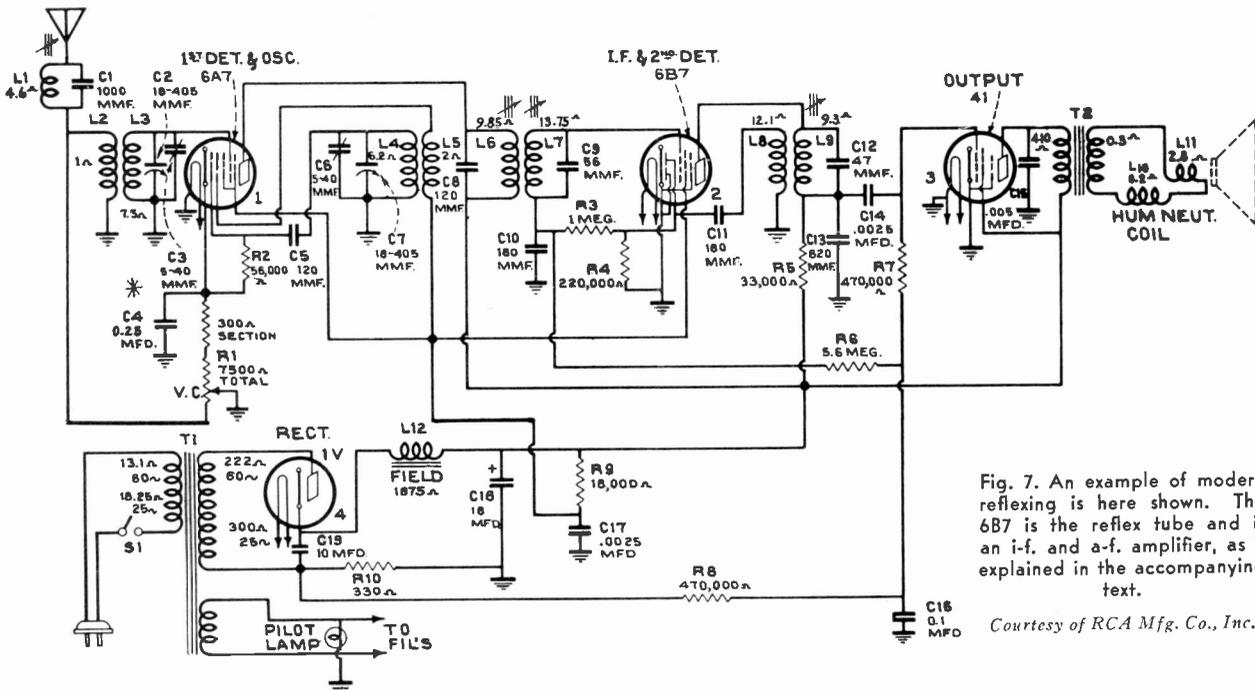
Fig. 7. An example of modern reflexing is here shown. The 6B7 is the reflex tube and is an i-f. and a-f. amplifier, as is explained in the accompanying text.
