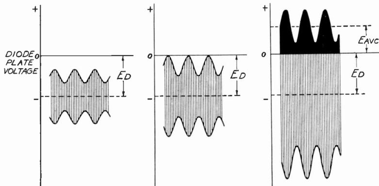
Fig. 6, left, shows the action when the peak value of the i-f. input to the avc rectifier is less than the delay voltage. Fig. 7 shows the peak value of the i-f. input equal to the delay voltage and Fig. 8, right, shows the i-f. input greater than the delay voltage. The resulting action is explained in the text.
