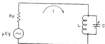
Fig. 2. Equivalent circuit of a single r-f amplifier stage.
