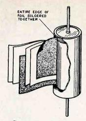
Construction of a paper tubular capacitor.
