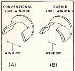
Fig. 1. Cross section of yoke winding.
