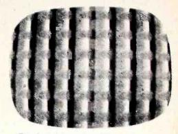
Fig. 7. Pattern produced by signal generator with 157.5 kc modulated by 400-cycle audio.
