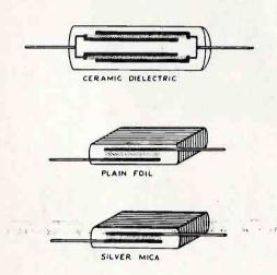
Construction of fixed mica and ceramic capacitors.
