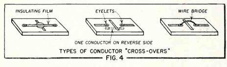
tube sockets and other components are sometimes connected to sprayed circuits by mounting them on the opposite side of the base plate so that the terminals protrude through holes into the grooves. Then, when the circuit is sprayed, connections are automatically made to the conductors. Circuit cross-overs are made in a manner similar to that employed in the painting process. Resistors, capacitors, and inductances may also be formed by spraying.
