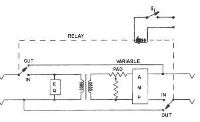
FIGURE 3: Ultimate equalizer-booster system. If input pad is "H" pad, input coil is not needed.
