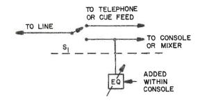
FIGURE 1: System for inserting equalizer in line. Switch Sl and equalizer can be either existing switch in console with equalizer added, or both may be external.
