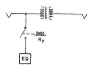
FIGURE 2: More flexible system providing equalizer bypassing for two way program feed.
