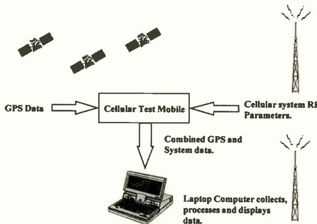
**FIGURE 1: Typical Cellular System Signal Measurements**
