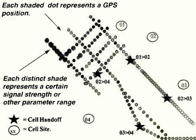
**FIGURE 2: Example of Signal Strength, System Event and GPS Position Plot**
