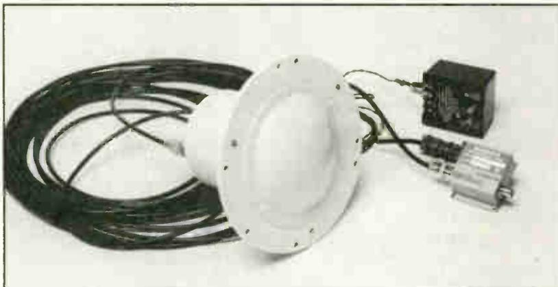
*The Integrated Feed Antenna/Down Converter is ready to mount on any dish - 36" or larger. A mounting ring is drilled to accommodate either a 3 or 4 strut mount. Unit is powered up by bias-T/regulator which splits off the 137.5 MHz IF to a BNC output connector, while routing regulated +15 VDC up the coax cable.*
