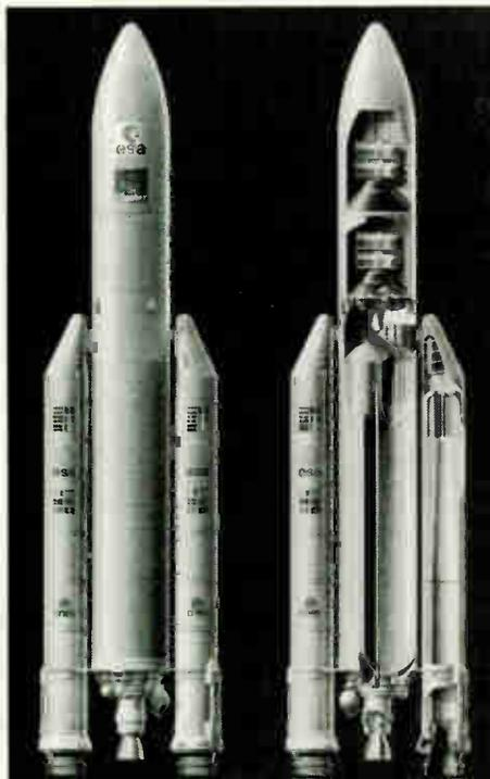
*Above, cross-sectional view of the the Ariane-5 launcher reveals the rocket's internal configuration for its doomed maiden flight with the four identical CLUSTER satellites.*
