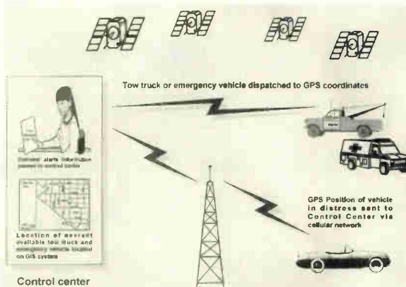
**FIGURE 1:** Using GPS to locate a driver in distress and dispatch the nearest break-down or emergency assistance
