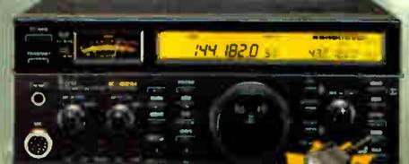
**IC-821H** 2M/440 MHz Advanced Satellite & Digital Base Station • All Modes • Easy to Use! • Continuous Adjustable Transmit Power • Sub Band Transmit • 9600 Full Compatibility Out of the Box • 160 Memories • Noise Blanker & IF Shift on Main & Sub bands (independent main/sub Rx) • Built-In Electronic Keyer • Compact Size! 9.5"(W), 3.7"(H), 9.4"(D), 11.0 lb
