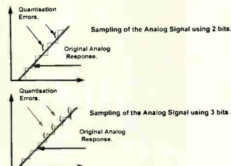
**FIGURE 3. Comparison of Sampling Resolution.**
