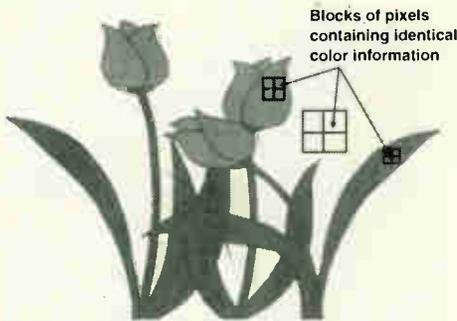
**FIGURE 2. Spatial Redundancy (Intraframe).**
