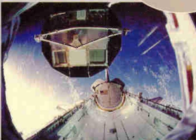
*There's no substitute for experience, and from its inception the Long-Duration Exposure Facility (LDEF) was employed as the ultimate orbital guinea pig, performing 87 experiments to gauge the long-term effects of space travel—not the least of which were tests on the space-worthiness of various structural materials.*
