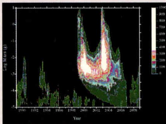
This figure, colored for impact, summarizes the early computer modeling results of the Leonid stream as performed by Peter Brown and the UWO Meteor Group. The Y axis shows the logarithm of meteoroid mass (10 g at top and 10 micrograms at the bottom) and the X-axis shows the time in years. The diagram in total shows which mass of Leonid meteoroids is predicted to be encountered by the Earth, and in what relative numbers according to computer simulations.
