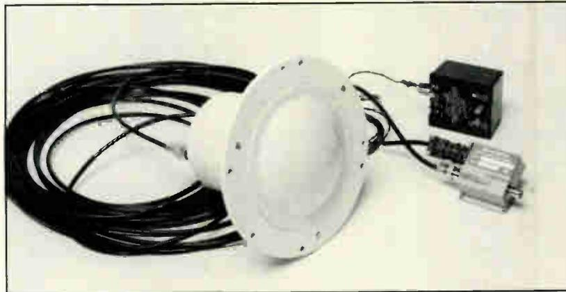
The Integrated Feed Antenna/LNA/Down Converter is ready to mount on our Model WPDA-3 Dish. A mounting ring is drilled to accommodate the 3 strut mount. Unit is powered by a bias-T/regulator which splits off the 137.5/137.1 MHz IF to a BNC output connector while routing regulated +15 VDC up the coax cable.
