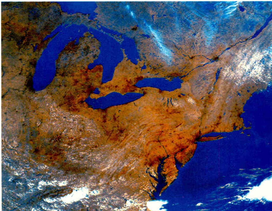
◀ Section of a multi-spectral, false-colored NOAA APT image of the Northeast US. This image was created directly from a raw image file using the MFCOLOR software from Weather Dynamics.
