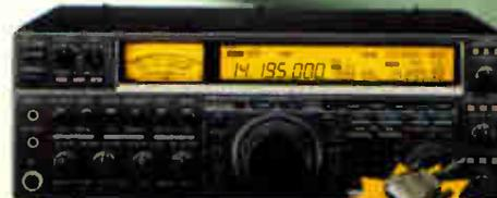
**IC-775DSP** Pull Out Those Weak Signals! • IF-DSP (Digital Signal Processing) on Tx and Rx • 200 W Stable Output Power • SSB/AM/FM/XCW/RTTY • Built-In Heavy Duty Power Supply • Built-In Auto Antenna Tuner • Auto IF Notch Filter • Adjustable DSP Noise Reduction • Level/Width Variable Noise Blanker • PSN Modulation • Much More, Call! • 16.7"(W), 5.9"(H), 15.4"(D), 36.8 lb
