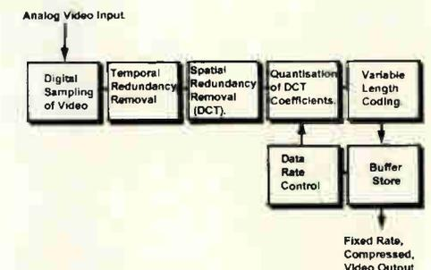
**FIGURE 4. Block Diagram of the Processes Involved in MPEG Compression.**
