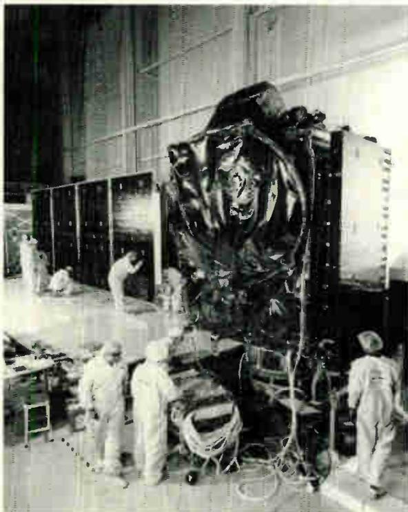
**Telstar 410 was the heaviest domestic communications satellite ever built, weighing 7,666 lbs.**
