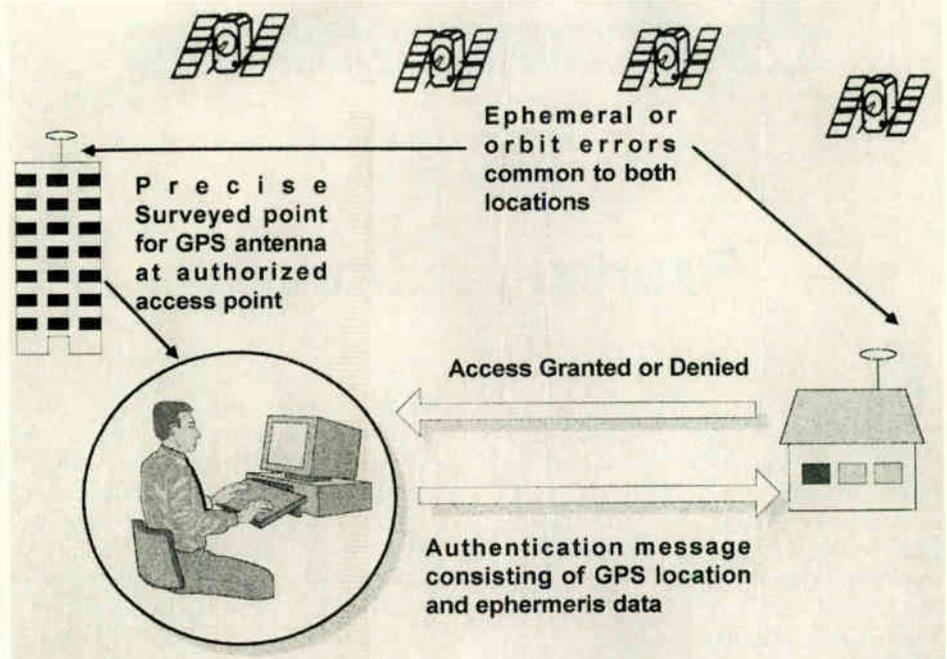
**FIGURE 2: Using GPS and its navigation message data to authenticate a users location**
