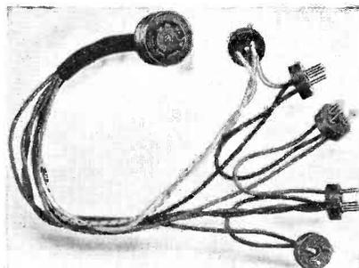
Fig. 3. B and C battery adapter.
