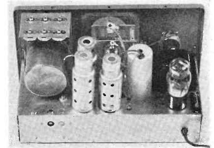
Fig. 5. The rear of the RCA model 150 test oscillator, showing positions of parts and tubes.
