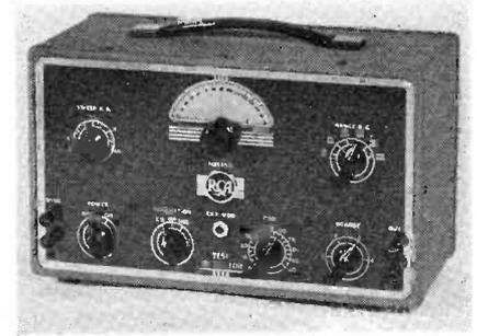
Fig. 4. The RCA model 150 test oscillator in its portable carrying case. Front view showing dial and panel arrangement.
