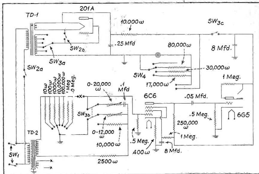
Fig. 4. Tobe a-c bridge-analyzer circuit.
