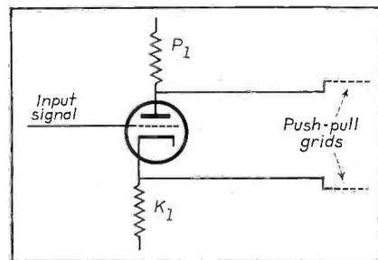
Fig. 4. Direct-coupled signal divider circuit.
