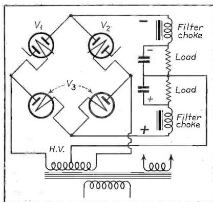
Fig. 1. Stabilized bridge type rectifier system.
