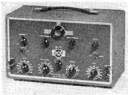
Fig. 1. The RCA model 151 cathode-ray oscilloscope in its portable carrying case. Front view showing calibrated screen and controls.
