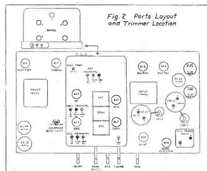
Fig. 2. G.E. E-129 parts layout and trimmer locations.
