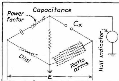
Fig. 5. Condenser analyzer part of bridge circuit.
