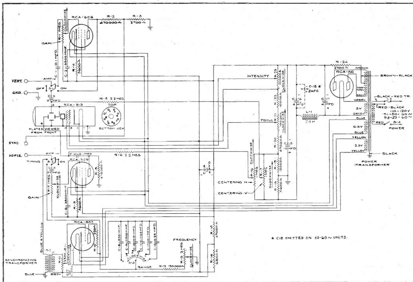
Fig. 3. The RCA model 151 cathode-ray oscilloscope circuit diagram.
