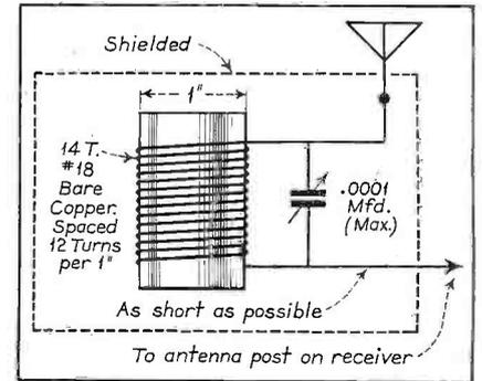
Fig. 2. Shunt wave trap.
