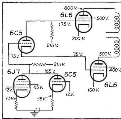
Fig. 5. Voltage distribution in the amplifier.
