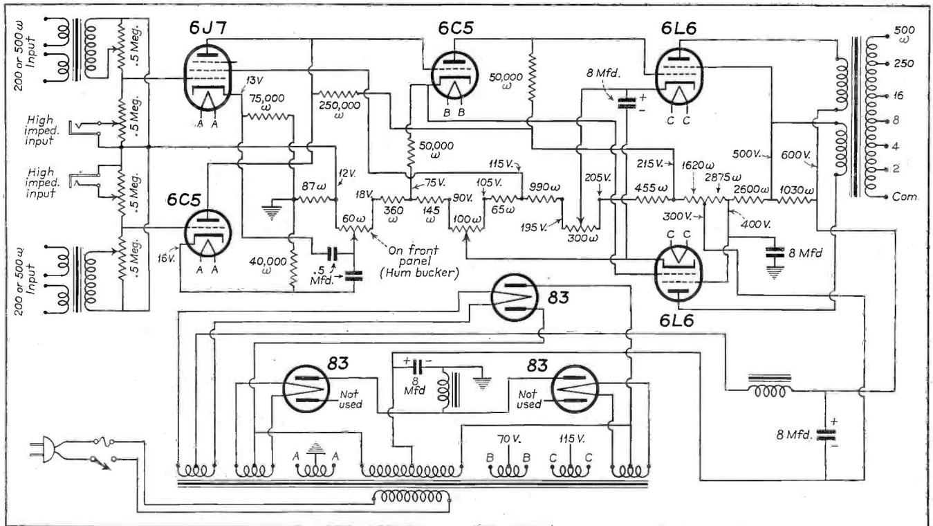
Fig. 6. The complete beam-power amplifier.
