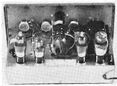
Fig. 2. The rear of the RCA model 151 cathode-ray oscilloscope with the case removed, showing positions of parts and tubes.
