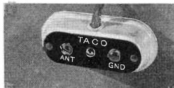
Exposed wiring coupler mounted on inside window sill or baseboard.
