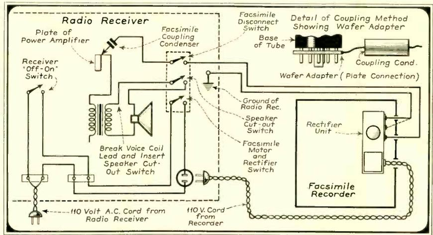
Fig. 1. A facsimile recorder may be connected to the average radio receiver by means of a simple plate connection wafer.
