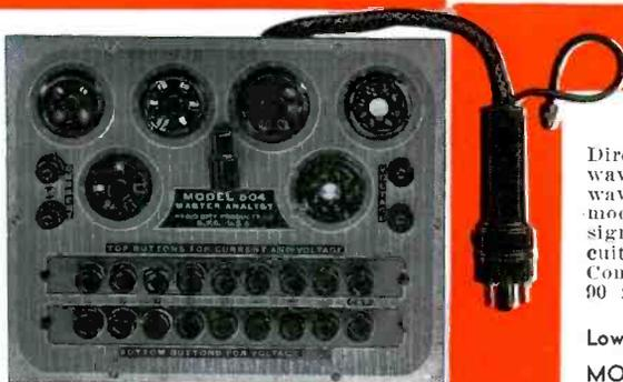
It seems RCP engineers have been working overtime. Laboratory 'info' says that the new Model 504 analyst will be ready March 1st. The Analyst is an improved unique push button circuit selector—making possible greater speed, safety and flexibility for analyzing symptoms at socket terminals in radio sets and P.A. installations.
