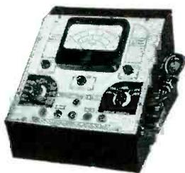
AC VACUUM TUBE VOLTMETER—DIRECT READING
