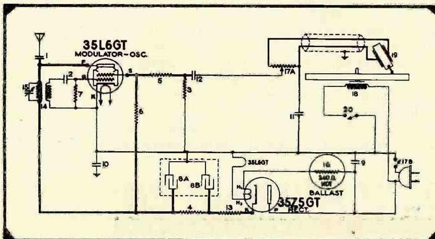
Fig. 5. Wireless record player with beam power tube, 35L6GT.
