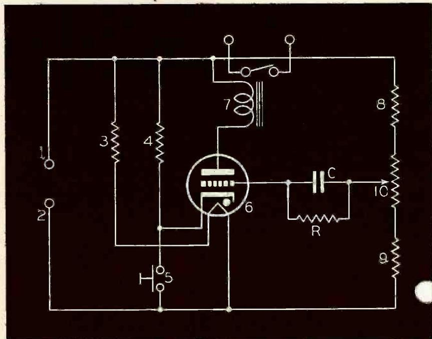
tion of the timing interval merely through adjustment of the rheostat knob.
