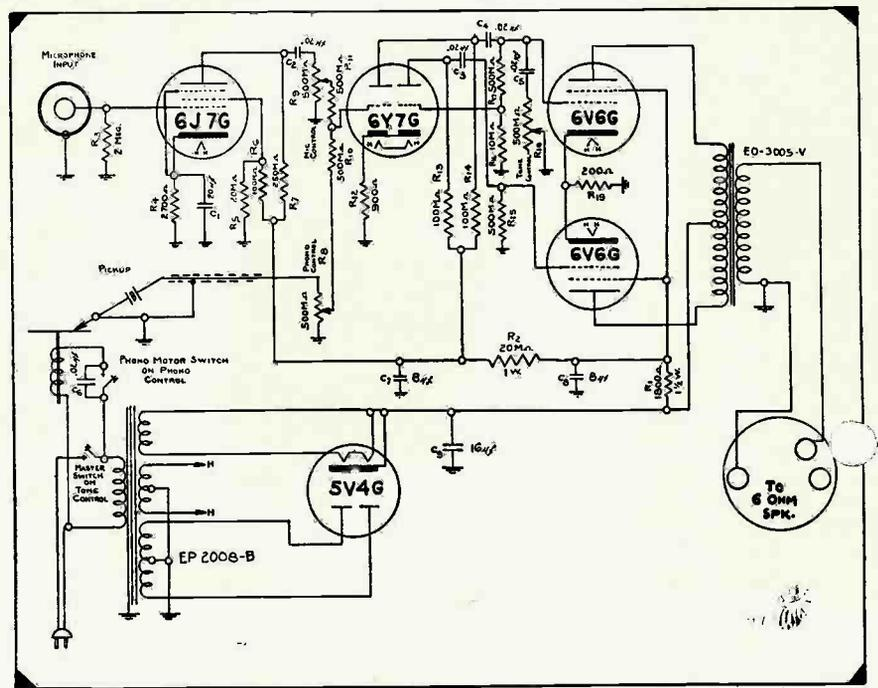
toward the plate. The second triode section of the 6SC7 serves as inverter. A pair of 6V6G's deliver the output to a speaker socket. A 5-megohm resistor connects each output tube plate with its driving triode plate to contribute a bit of degeneration.
