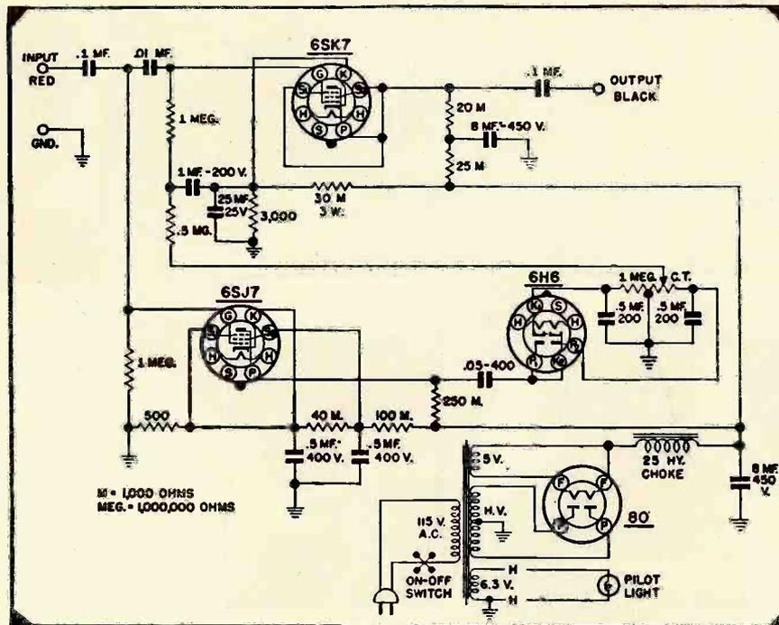
Fig. 4. Expander-compressor adapter unit that can be used with a standard amplifier.
