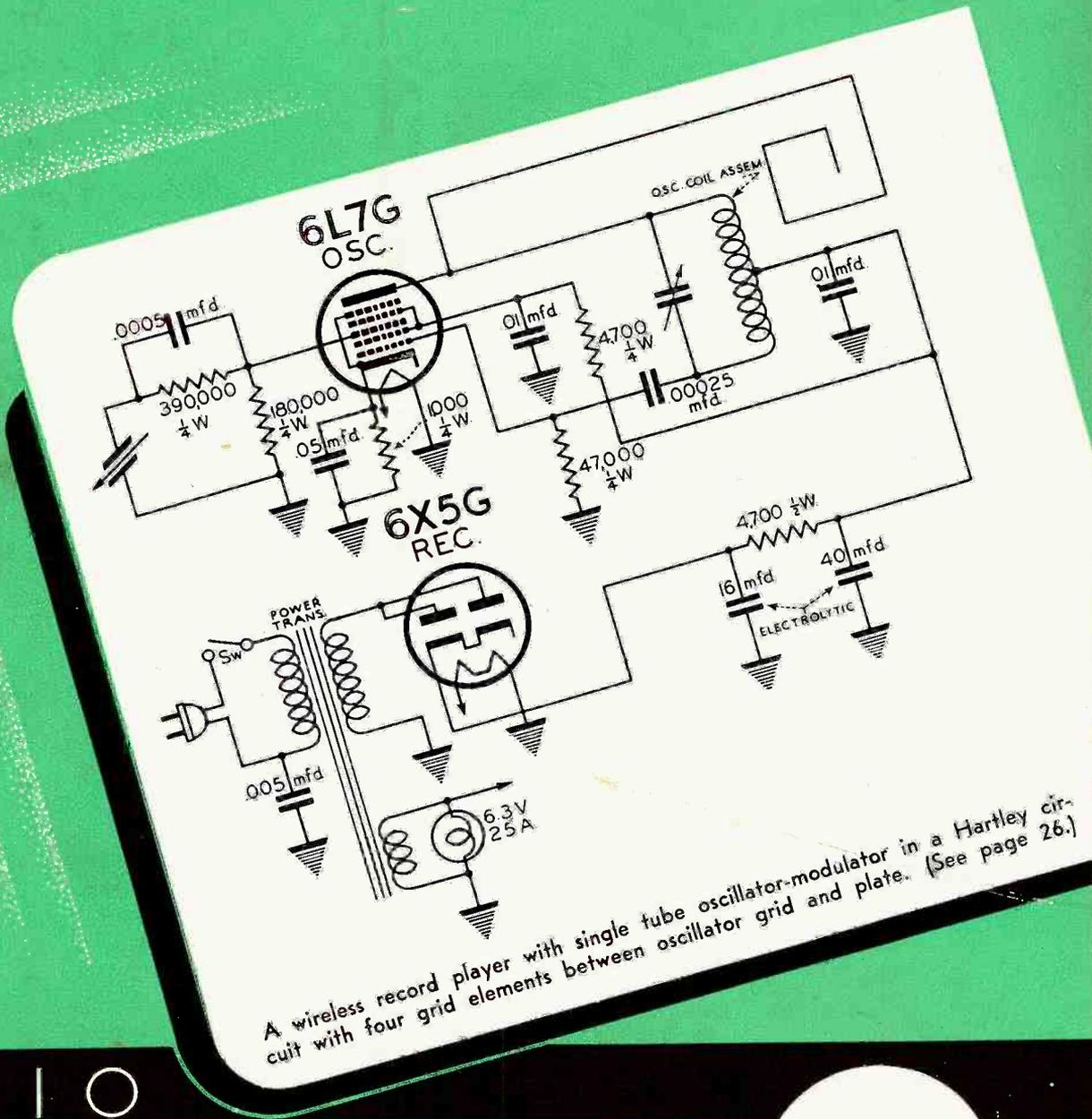
A wireless record player with single tube oscillator-modulator in a Hartley circuit with four grid elements between oscillator grid and plate. (See page 26.)
