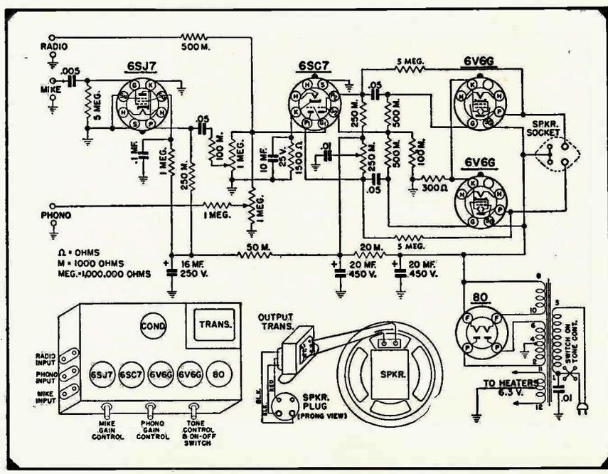
output load for the first stage, with the consequent distortion. Similarly, a 1-megohm resistor is used in the phono input to the arm of the phono volume control.
