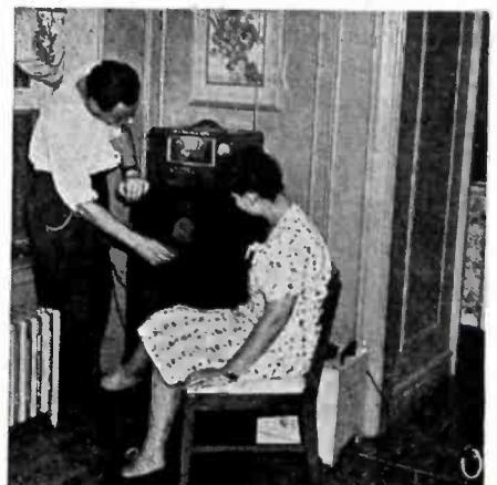
Rotating an f-m dipole for maximum signal response.
