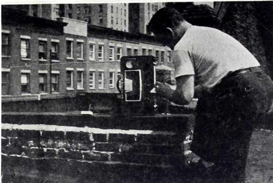
Checking antenna-location possibilities with f-m test unit. Receiver is placed in horizontal position for reception of horizontally polarized signals.
