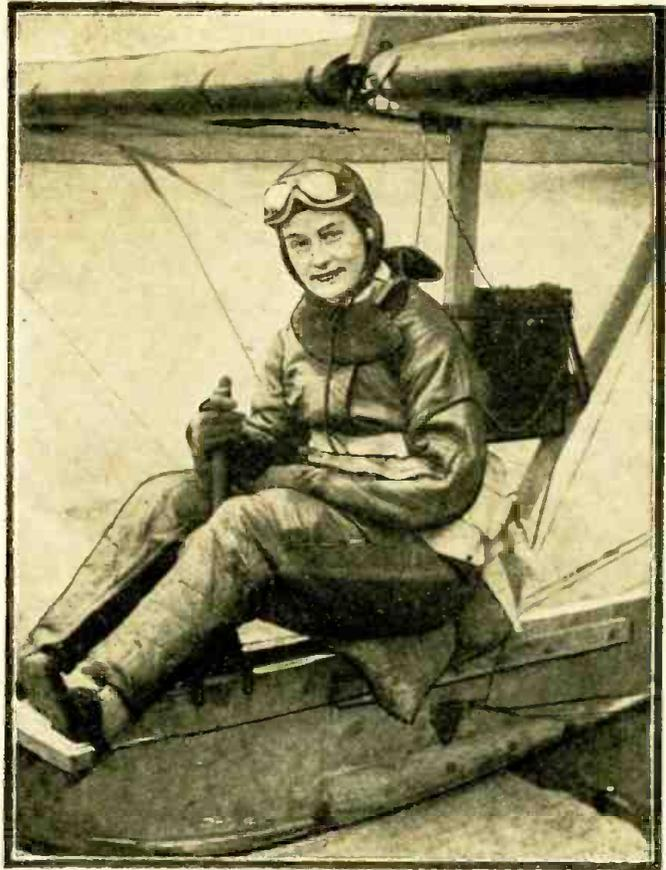
Mrs. Alicia Patterson Simpson at the glider controls. Note short-wave radio receiver mounted just back of the fair pilot. Radiophone instructions were received through headphones worn by Mrs. Simpson.
