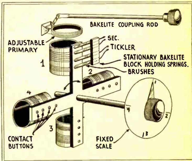
There are many variations of this arrangement, of course, and more crossarms can be used in the event that more than four coils are to be switched into and out of circuit. Most everyone knows that the reason why we use plug-in coils for short-wave circuits is because tapped coils or coils with sliders leave a lot of inductance in a circuit, which due to its electrical capacity and also a certain inductive (reactive) effect of the turns left connected, through unipolar cur-
