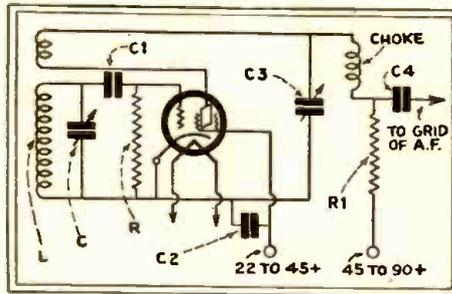
Hook-up of screen-grid tube in short-wave detector circuit, showing choke coil, condensers, etc.
