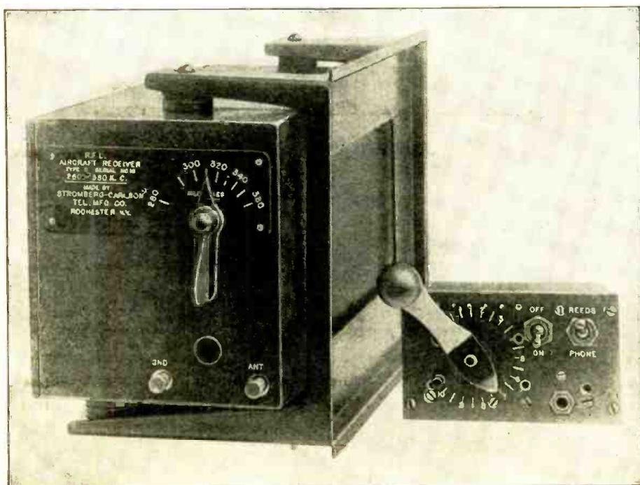
The Stromberg-Carlson Model B aircraft radio receiver, designed to receive weather and radio-beacon signals. It employs 5 tubes and requires only a 5-foot vertical mast for reception; it weighs 12 lbs.
