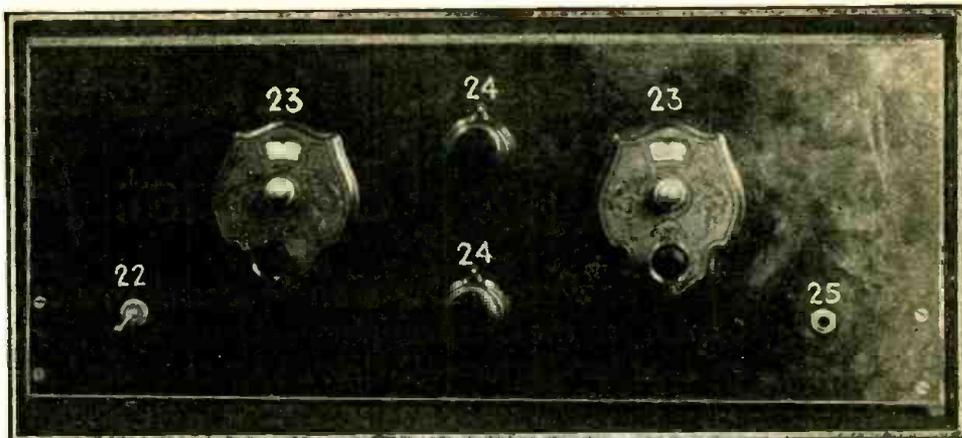
At right (above), panel arrangement of the "Two-in-One" receiver. The dials are of the illuminated type. If operation of the circuit-change switch is desired at the panel, one additional control knob will require to be provided for.
