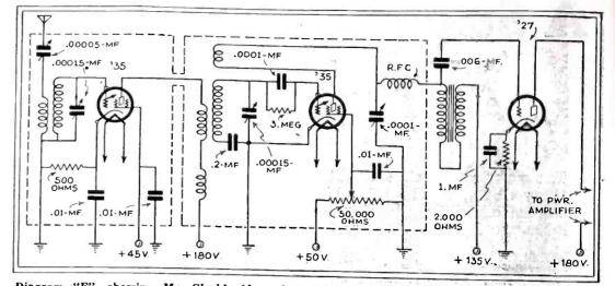
Diagram "F", showing Mr. Slack's idea of a good short-wave receiver with smooth control of regeneration and other features.
