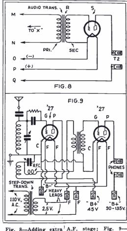
Fig. 8-Adding extra <sup>1</sup> A.F. stage; Fig. 9-A.C. Tube hook-up.
