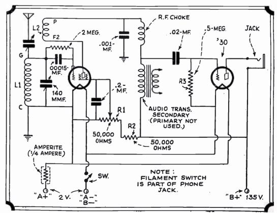
Schematic diagram of the 2-tube receiver here described. It's really so easy to build that you need not have had any previous experience in constructing sets.
