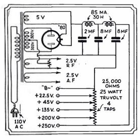
Power-pack circuit requested by Mr. Webster, and in which an '80 type rectifier tube is used. The two 30 henry chokes have iron cores.
