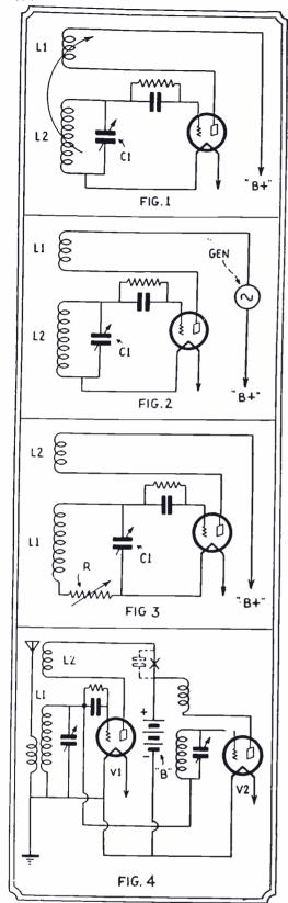
Figs. 1 and 2, simple regenerative circuits. 3, resistance control of oscillatory circuit. 4, basic super-regenerative circuit.
