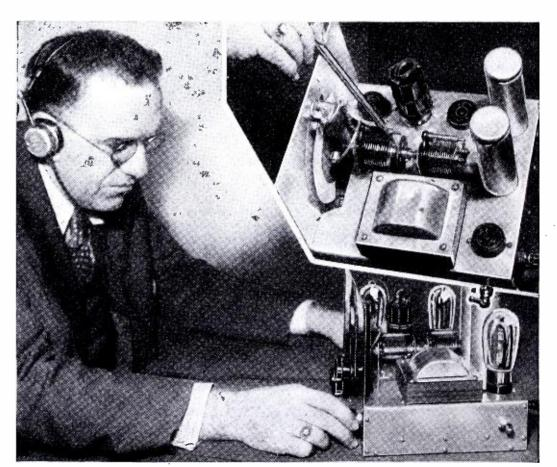
Fifth prize winner—a high-grade, short-wave converter built by C. E. Utermohle. It permits the reception of short waves on any "broadcast" receiver.
