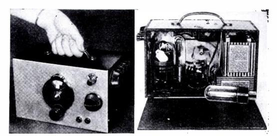
Two tubes, plus batteries and plug-in coils, a condenser or two, and a dial, make up this nifty little portable—a "delight to the ear as well as the eye."
