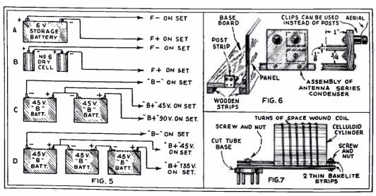
Fig. 5—left, battery connections for the Binneweg 2-tube receiver. Fig. 6—Assembly of the antenna series condenser. Fig. 7—Mounting for celluloid-supported low-loss coils.
