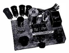
Note the neat construction of the Royal S-W receivers: plug-in coils in background.
