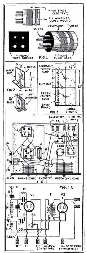
Details of plug-in coils, and also panel, sub-panel, and schematic wiring details.
