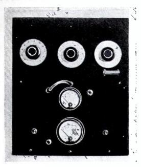
Front view of 2 tube portable transmitter.
