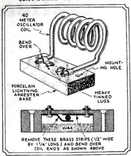
Simple coil mount from lightning arrester
