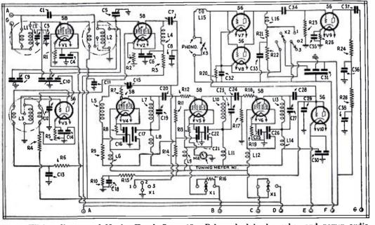
Above: Wiring diagram of Norden-Hauck Super-15. line-up.
