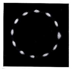
Electrons oscillating in the electrodelless gas filled glass ring illustrated in Fig. 6. ..The ring is filled with Neon and Helium.
