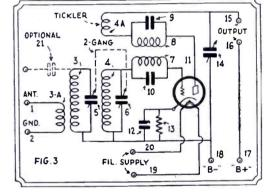
A.C. schematic diagram for the 1-tube superregenerator.
