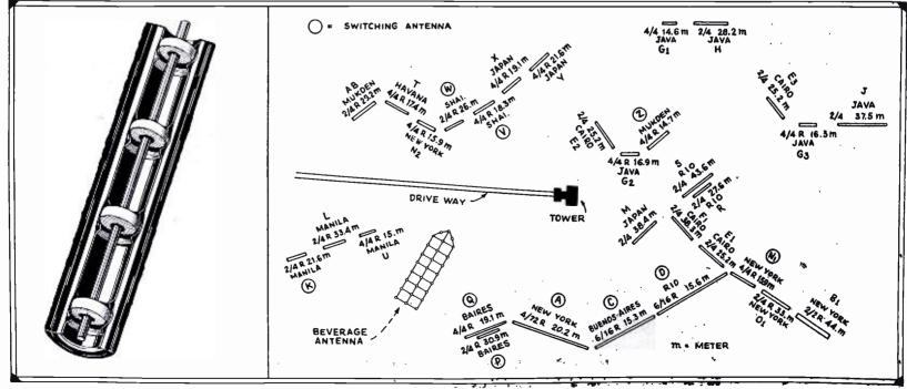
Left—Cross sectional view of the new high-frequency "energy cable" devised by the Telefunken Company, and used for connecting the antenna with the transmitter or receiver in short-wave stations. Plan view at right shows directional antennas and also position of ultra short-wave antenna tower.
