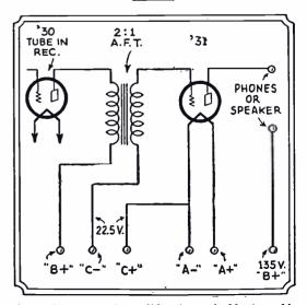
An audio stage of amplification suitable for add-ing to a first audio or detector stage.
