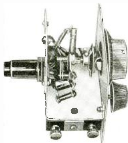
A close-up of the adapter, showing the single metal tube at the right, as well as the tuning condenser and dials.
