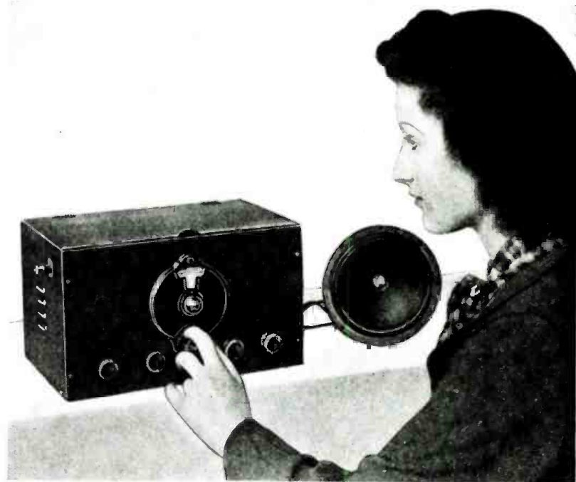
Tuning in the 5-meter stations is indeed a pleasure, with this perfected Acorn tube circuit devised by Mr. Shuart.
