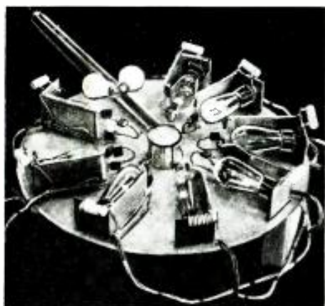
Photo above shows complete multi-tube oscillator as designed by Mr. Zottu. In the center of the group of tubes there is a specially designed low-loss tank circuit. The tubes are coupled to the tank through by-pass condensers.
