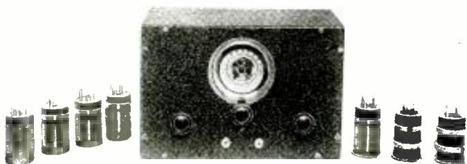
2-tube all-wave receiver—an excellent “headphone” job—and it has a range of 9\frac{1}{2} to 2,000 meters.
