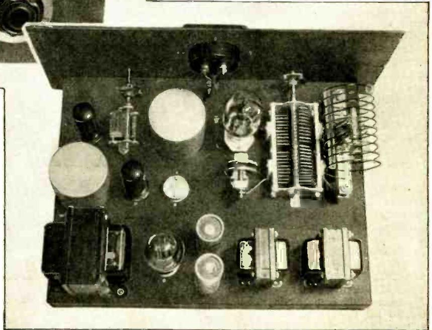
● NOT so long ago it required a 2 quart bottle to pack 250 watts of R.F. Lately it seems that the "bottle" is getting smaller and the contents getting more powerful. At the moment we have a tube not much larger than the old 201A and capable of over 200 watts output. This tube is the new HK-54, a swell tube for the medium-power transmitter. The entire transmitter featured in this story was built around the new tube.
