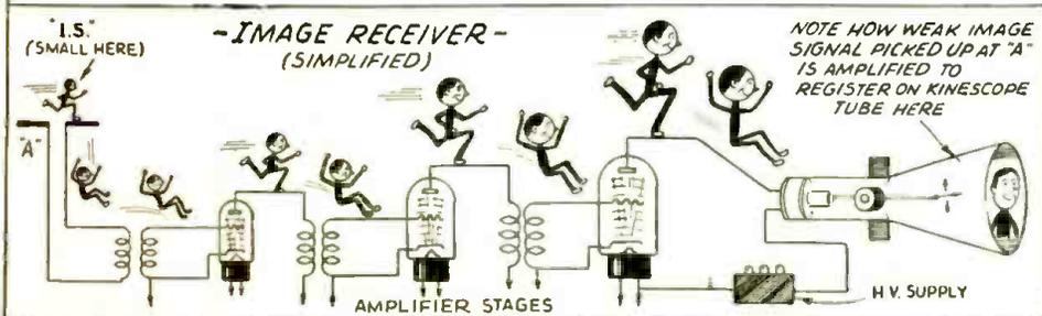
The process of picking up, transmitting and receiving the television image, as well as the sound is shown in the diagrams above and to the left. The lower diagram is presented for the general reader who may find it difficult to follow the more technical diagram above. Note how the image, as well as the sound currents, is continuously amplified.
