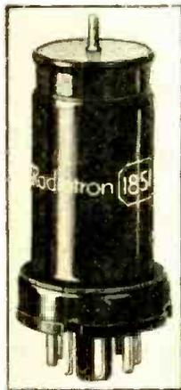
• THE 1851, a new pentode with unusual characteristics, has been developed for use by the amateur and experimenter in experimental television receivers. It is especially designed for use in the R.F. and I.F. stages of a television receiver employing a high I.F. It may also be used in the first stages of a video amplifier, particularly noteworthy is the amplification factor of 6750 and the trans-conductance of 9000 micromhos. The 1851
