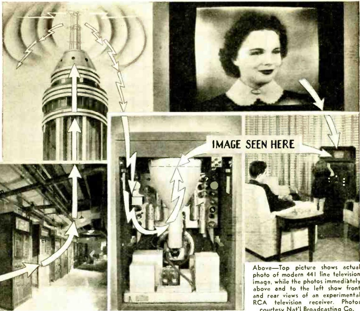
Above—Top picture shows actual photo of modern 441 line television image, while the photos immediately above and to the left show front and rear views of an experimental RCA television receiver. Photos courtesy Nat'l Broadcasting Co.
