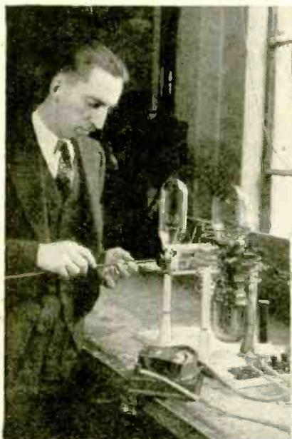
This new U.H.F. tube uses a glass cup as base to which copper terminals are fused.
