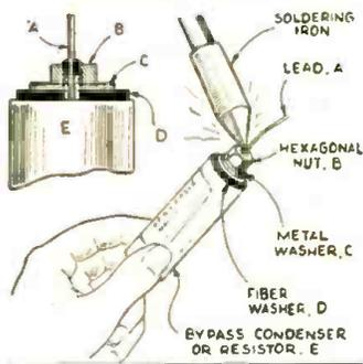
How many experimenters have found that after using a pigtail tubular condenser in several circuits the pigtail leads break off flush with the side of the condenser?
