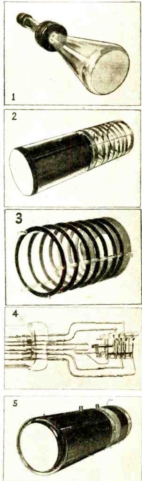
Beginning with top photo—television cathode ray tube using magnetic focusing; experimental electron image tube; electrode system of electro-statically focused image tube; condensing electron lens system; experimental electron gun for use with magnetic focusing.
