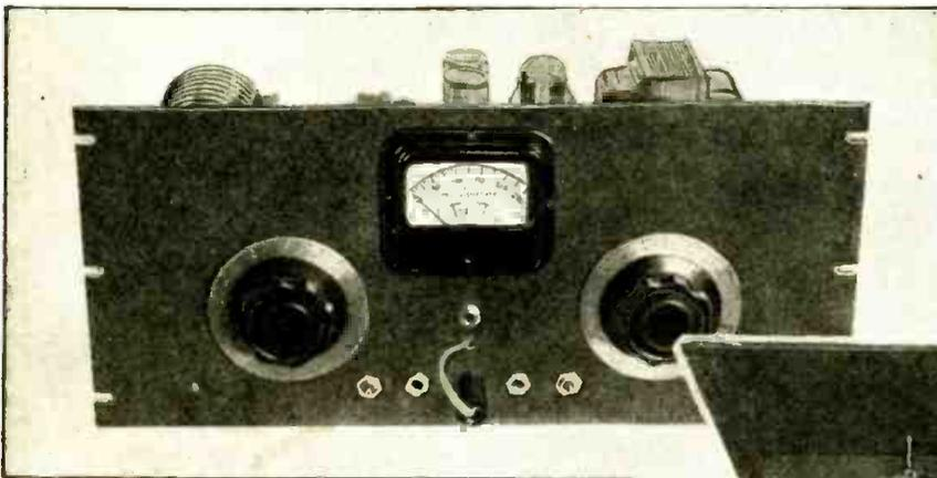
used 6L6 beam tubes in the exciter stages. We also have kept the number of stages down to a minimum, knowing that it is just as economical to buy crystals as the other components, and it is a lot easier.
