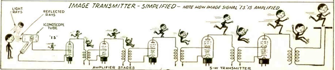
By following the large arrows across the series of pictures, the path of the television image is easily traced. Below, we see the image and sound signals passing through the transmitters located in the Empire State Building. The image is "piped" from the NBC studio in Radio City through a coaxial cable to the Empire State Tower.
