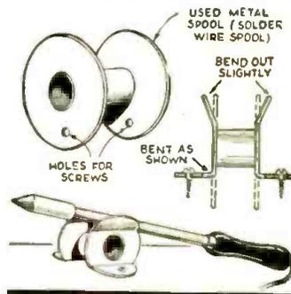
Our old friend, the soldering iron holder, comes under a new guise this month. This holder is made from an empty solder spool. As the illustration shows, the holder may be secured to the work-bench by wood screws.—*Bill Knife.*
