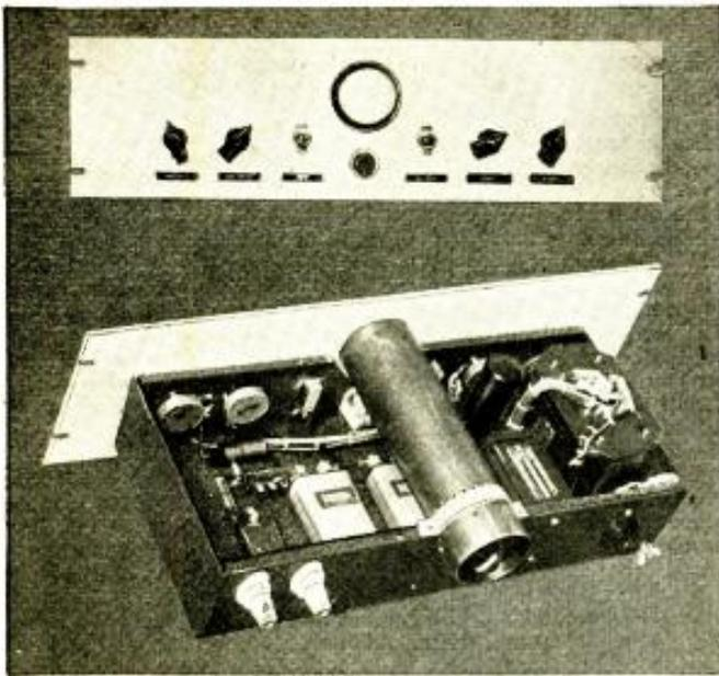
Front and top views of cathode ray oscillograph as built up for "rack" mounting by Mr. McEntee. It is very compact and forms a useful and handy adjunct to any complete Ham transmitter.
