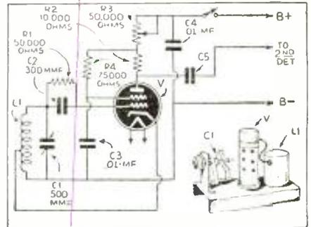
Circuit diagram for a simple and very useful beat-frequency oscillator, which will make it easy to locate those elusive DX stations.
