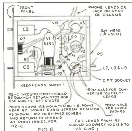
Bottom view, showing how 6J8G tube is mounted, also disposition of the other parts.
