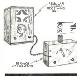
can be used in matching I.F. coils, by tuning the radio to a strong harmonic of the oscillator frequency.—*Frederick F. Slack.*
