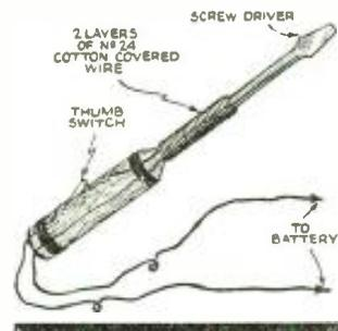
hold a bolt or a screw for insertion in an out-of-the-way corner. Of course, the tool will not operate with brass screws.—*Steve S. Boychuk.*
