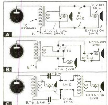
The diagrams show three methods of connecting an extension loudspeaker.
