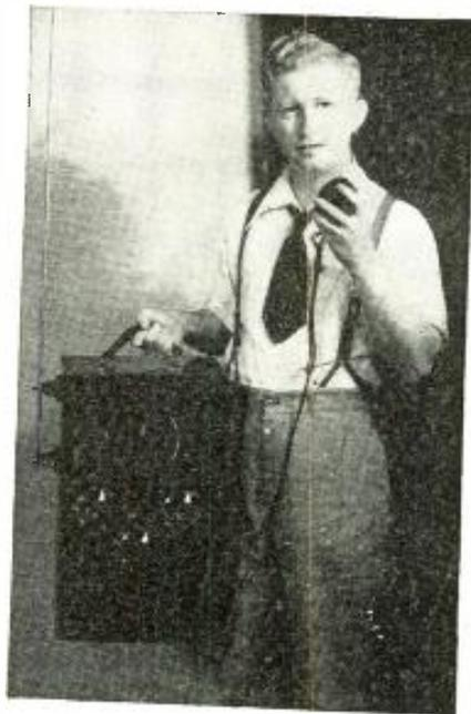
The portable 2½ meter transceiver—it carries 2-way phone.
