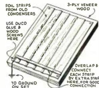
system entirely eliminates the hand capacity which is so bothersome on short wave apparatus.
