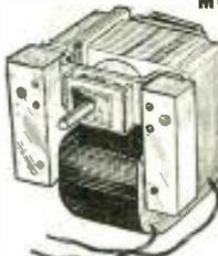
A self-starting shaded pole motor originally designed for use on radio chassis for Push Button Tuning. High speed and powerful. One lubrication lasts lifetime. Excellent for model railroad trains, small boats, humidifier water pumps and a host of other uses. Has 1/2" long shaft, 3/16" diameter. Complete with brass mounting posts. Measures 2 1/2" x 2" x 2 1/4" overall. For 110 volts, 60 cycles, A.C. only. Shp. wt. 4 lbs.
