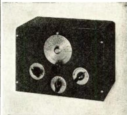
● Using an 1852 tube, a gain of 1000 or more and image rejection ratios of 500 or more may be obtained ● Coverage from 1.6 to 64 MC with band switching ● Electrical bandwidth ● Regenerative circuit with exceptionally smooth control ● Built-in filament transformer ● May be used as Short Wave Converter ● Completely wired and tested, Type 5DXP, Net Price \$16.50, less tube ● Also available in kit form, Type 5DXK, Net Price \$13.50 complete except for tube. ● Send for Bulletin 103-A.
