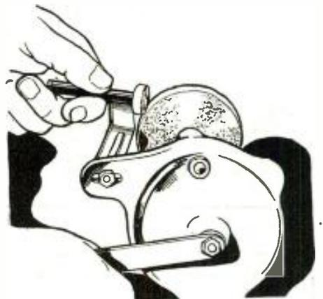
Roughing out glass lens blank on hand-operated grinding wheel.
