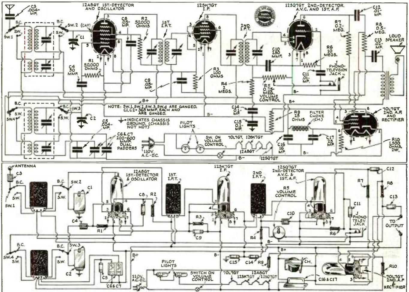
Wiring diagram of the 2-band receiver.
