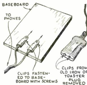
posts. However, I had some old plugs of the type used for electric irons and toasters. I removed the clips from these plugs and screwed them to the board, where they worked fine as phone jacks.—Dayton Baldwin, Jr.
