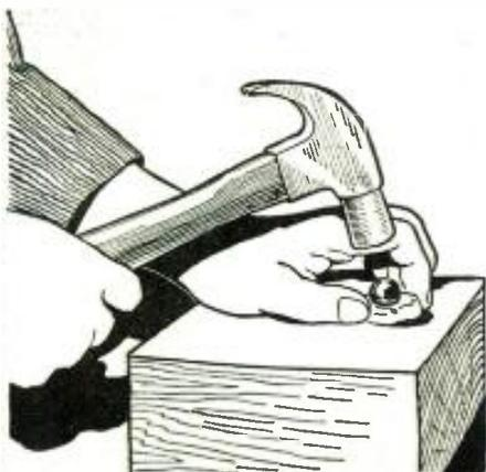
Ball bearing hammered into lead sheet makes grinding lap.
