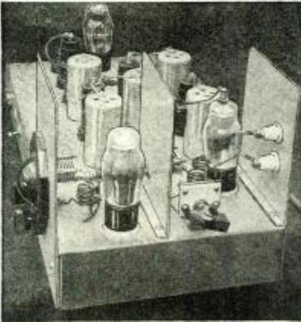
View of the 8-tube television receiver chassis, showing shields. The sweep circuits and power supply are mounted on separate units and will be described next month.
