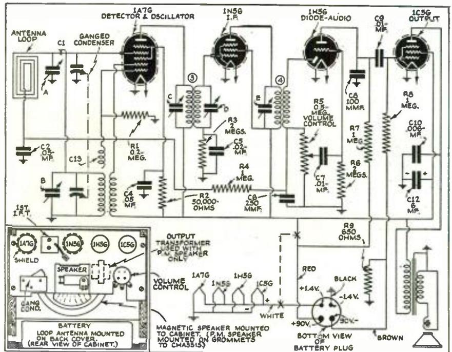
The battery used on this receiver is a 1 1/2 volt and 90 volt "AB" dry pack 6 1/2" x 5 7/16" x 2 3/4" in size. Knight battery No. A10049 is recommended for this receiver. This battery pack has a minimum life of about 150 continuous hours. The life may be appreciably extended to above 200 hours under intermittent use.
