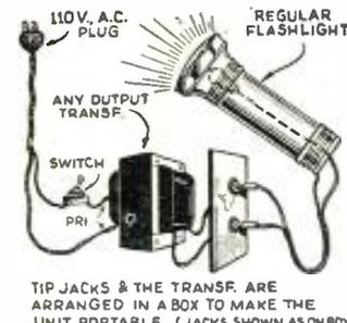
TIP JACKS & THE TRANSF. ARE ARRANGED IN A BOX TO MAKE THE UNIT PORTABLE. (JACKS SHOWN AS ON BOX)
