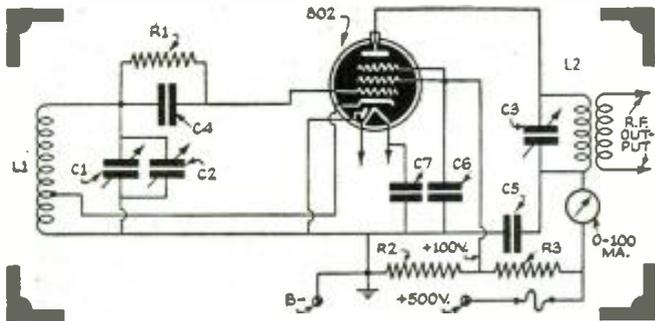
Electron-coupled oscillator for transmitter. No. 1210.
