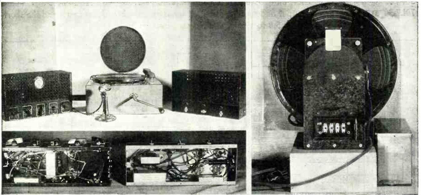
Photos above show front and bottom views of the A.F. amplifier and its power-supply unit. Right-hand photo shows loud-speaker.
