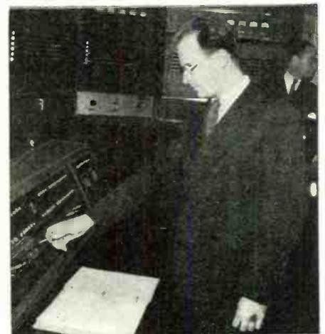
Dr. Peter C. Goldmark, chief television engineer for CBS, shown at the transmitter control desk in the Chrysler Tower. Signal lights and transmitter controls are seen at lower left. The sound transmitter is in the background.
