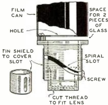
How focus slot is made light-tight.
