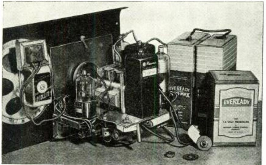
Here is a view showing all the parts, including the batteries, for building the portable 3-tube receiver, which does the work of 6 tubes.
