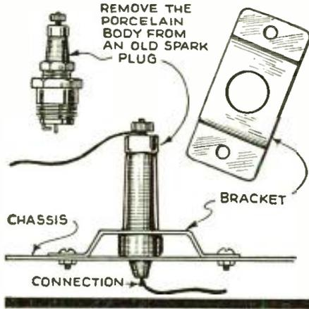
center of the plug. If space permits the mounting bracket may be installed underneath the chassis.—Richard Krogman.
