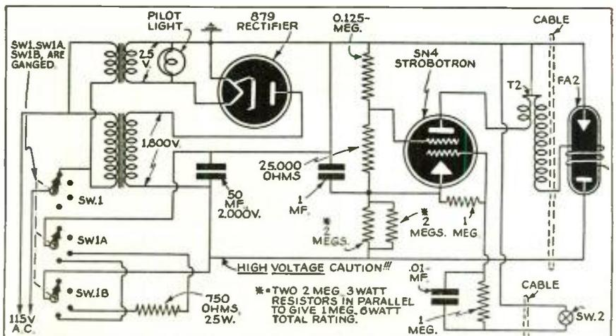
Wiring diagram of Speedlight flash unit—insulate high voltage wiring carefully.
