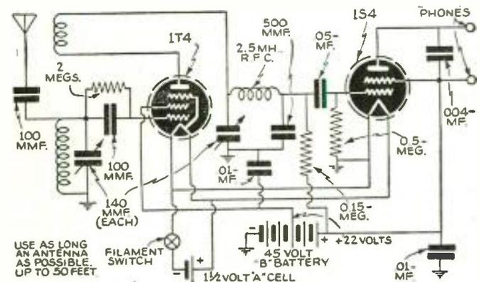
A 2-Tube Receiver for the experimenter. (No. 1227)
