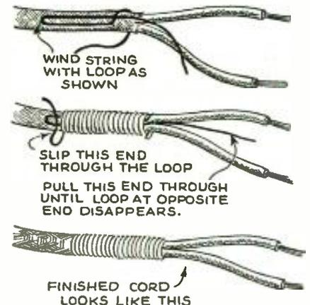
ping as possible. The cord will be firmly secured, and no knots or loose ends will remain.—Steve Liska.
