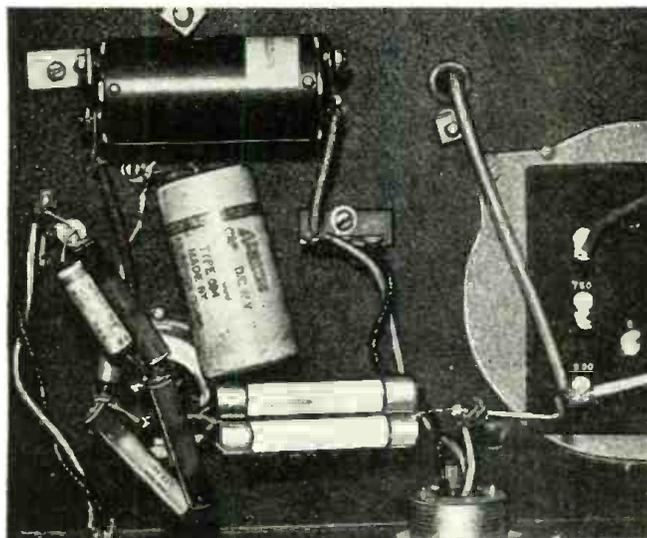
Closeup of Strobotron socket, showing resistor network.
