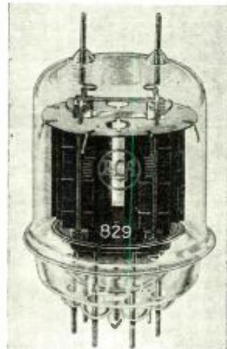
60 ma. is approximately 8500 micromhos. The grid-screen mu-factor is 7. The tube may be used as grid modulated push-pull R.F. power amplifier in class C telephony, as plate-modulated push-pull R.F. power amplifier in class C telephony, or as push-pull R.F. power amplifier and oscillator in class C telegraphy. A complete description with characteristics, applications, diagrams and charts appears in an 8 page booklet published by the manufacturer.
