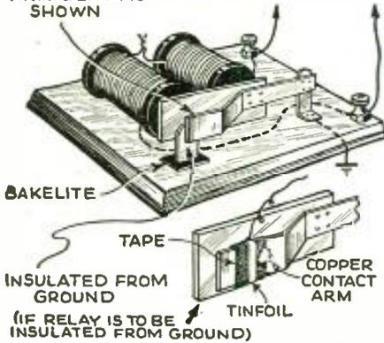
of the 10c store variety. The circuit of the buzzer is changed, the interrupter being disconnected from the magnet circuit. The magnet is connected directly as the primary and when energized attracts the rebent contact, causing it to close the secondary circuit. If necessary the relay may be rebuilt to insulate the contact arm bracket from the base.—Harry Greenberg, W2MSQ.
