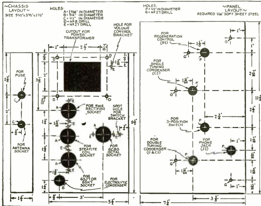
Layout details for the panel and the chassis of the receiver are given above.
