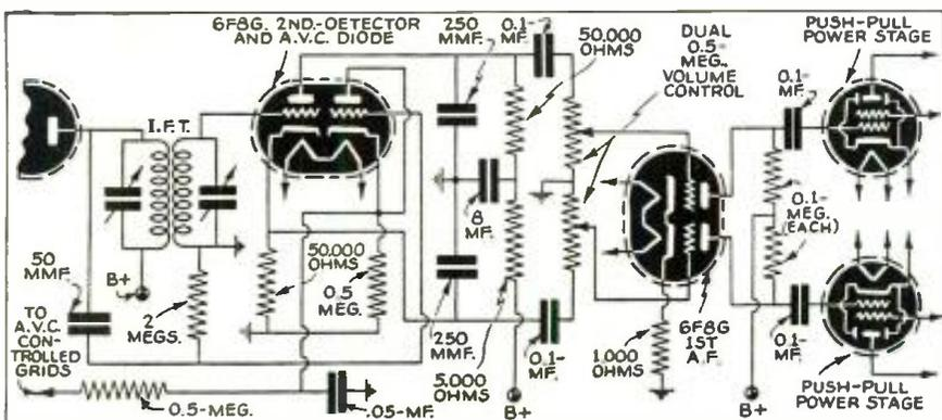
This interesting circuit was supplied by Harvey Gernsback, and shows the hook-up for an infinite-impedance second detector in a superhet receiver. Note that this circuit permits the second detector to feed the push-pull audio frequency amplifier stage, without the use of a transformer.
