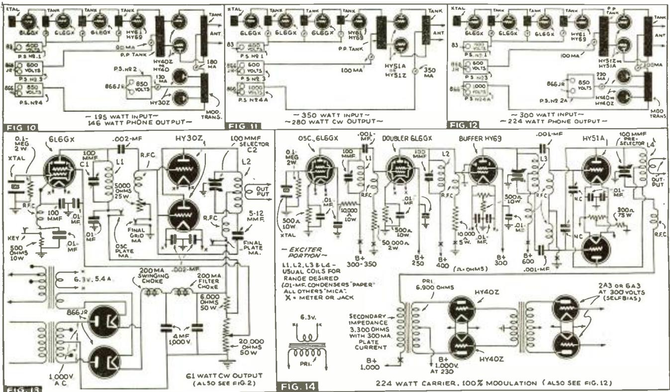
Fig. 10—phone Xmitter of 146 watts output; Fig. 11—280 watt output CW rig; Fig. 12—set-up for 224 watts output, phone; Fig. 13—complete diagram of 61 watt CW output transmitter (refer also to Fig. 2); Fig. 14—phone Xmitter of 224 watts output (refer also to block diagram, Fig. 12).
