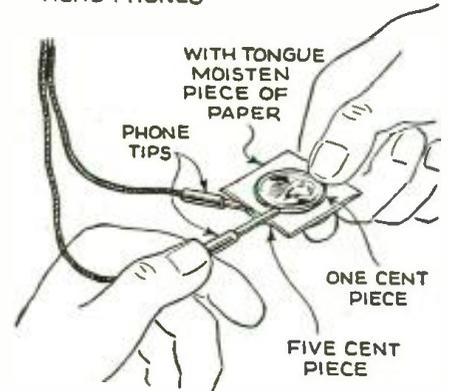
paper. This paper must be thoroughly moistened with saliva, which serves as electrolyte in the tiny battery. Touch one phone tip to the nickel and start tapping the penny with the other. If the phones are in working condition a faint click will be heard when the penny is tapped.—James Haluszczak.
