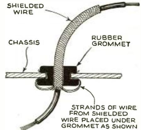
nection but also holds the wire in place and makes a neat end on the shield.—Oleg Mcinikoff.
