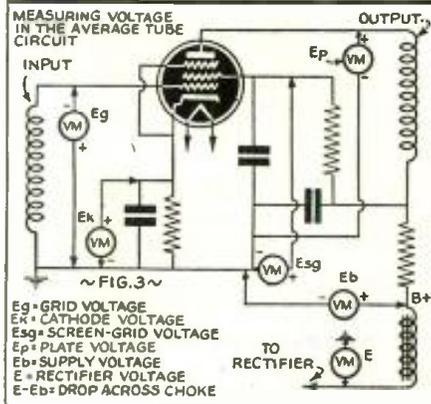
How and where to make voltage tests.
