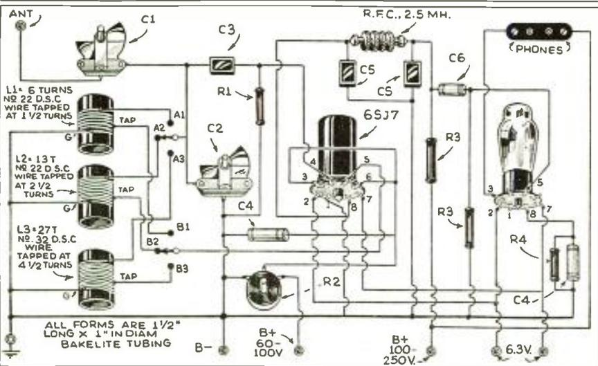
By merely turning a switch, three short wave bands (from 15 to 100 meters) are quickly and easily covered.
