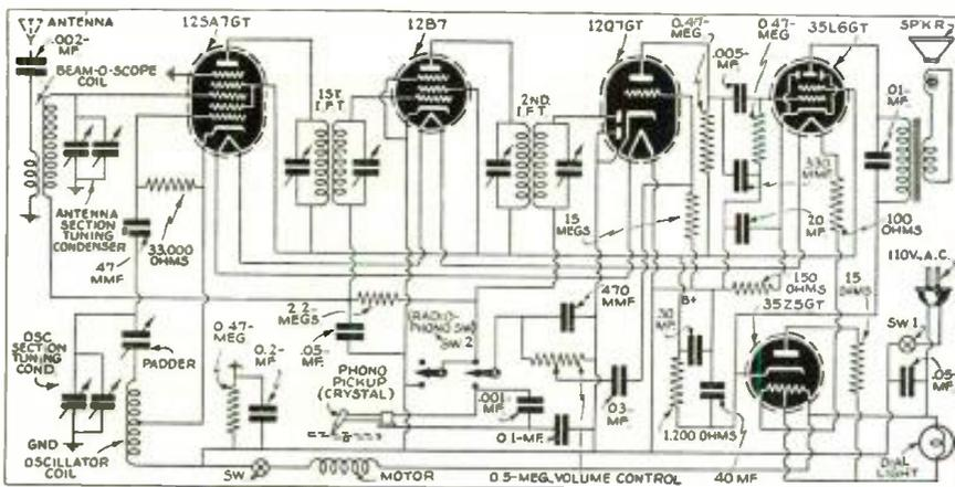
The diagram above shows the G.E. Co. model H508 portable radio phonograph combination circuit. A crystal phono pickup is used and the circuit is adapted for operation on 115 volts A.C. The lineup of tubes comprises a superhet with one stage of I.F. amplification. Variations of this circuit will prove interesting to experimenters.
