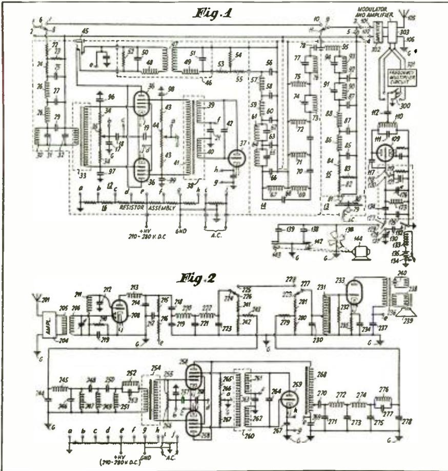
Top:—Transmitter of new system. Bottom:—The accompanying receiver.
