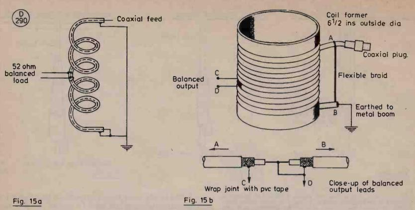
Fig. 15. (a) Broadband coaxial balun; (b) Broadband coaxial balun.
