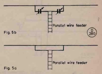
Fig. 5. (a) Basic T-Match: de-tuning effect from the T-rods is compensated by adjustment of length of antenna to restore resonance; (b) T-Match with compensating capacitors which tune out the reactance introduced by the T-rods.
