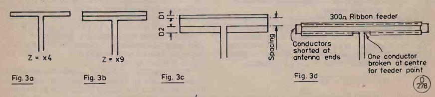
Fig. 3. (a) Simple folded dipole; (b) Three-conductor folded dipole; (c) Folded dipole using conductors of different diameters. With this technique a wide range of impedance transformations may be obtained; (d) The use of 300-ohm 'ribbon' feeder for the construction of folded dipoles.
