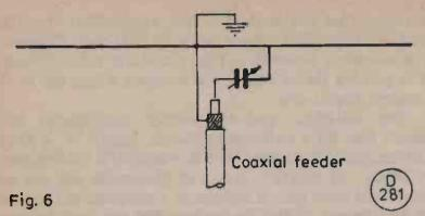
Fig. 6. The Gamma Match: this technique permits a balanced antenna, such as an Yagi, to be fed with coaxial feeder. The feeder screen is connected directly to the centre of the driven element, which should be earthed at its centre.
