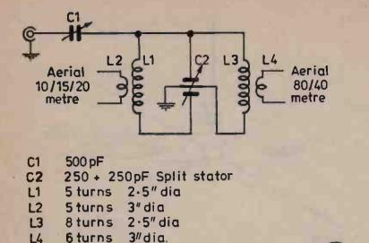
Fig. 9. The HF antenna matching unit mentioned in the text; note that L1 is mounted inside L2, and L3 is mounted inside L4. More detailed constructional information is contained in the RSGB Radio Communication Handbook.
