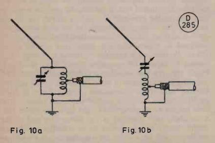
Fig. 10. (a) Tuner unit for use with end-fed antennas whose length is a multiple of a half-wave (parallel-tuned circuit); (b) Tuner unit for use with end-fed antennas whose length is an odd multiple of quarter-waves (series-tuned circuit).
