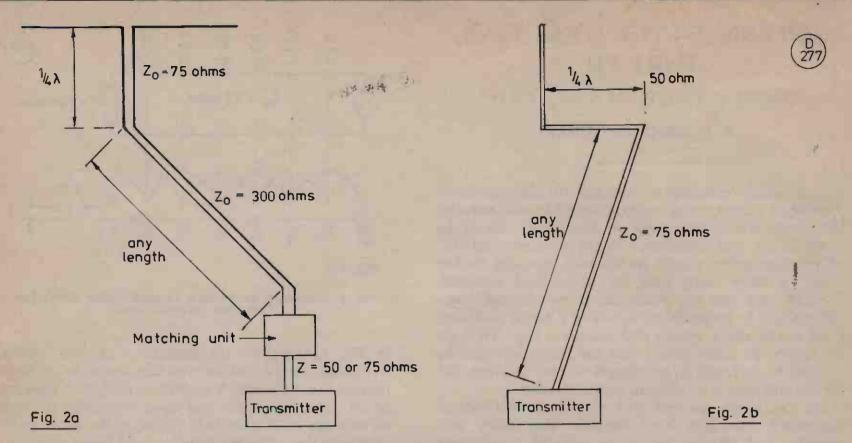
Fig. 2. (a) Half-wave dipole using transformer of quarter of 75-ohm feeder; (b) Vertical antenna using transformer of quarter of 50-ohm feeder.
