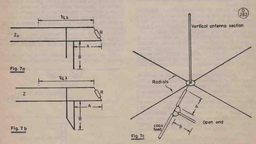
Fig. 7. (a) Matching with open stub, where R is less than  $Z_o$ ; (b) Matching with closed stub, where R is greater than  $Z_o$ ; (c) Stub matching for a ground-plane antenna using coaxial feeder. As the feed impedance is lower than the feeder's characteristic impedance, an open stub is employed.
