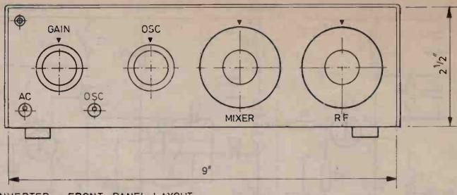
Fig. 3 HF CONVERTER - FRONT PANEL LAYOUT
