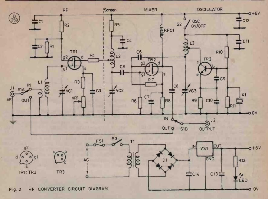
similar device as a mixer. A 2N2222 is employed in the 10 MHz crystal and harmonic oscillator.
