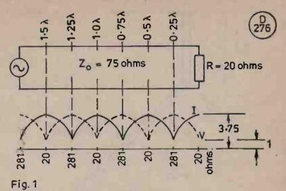
Fig. 1. Standing waves on a 75-ohm feeder connected to 20-ohm resistive load.
