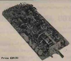
ARIO Mosfet receiver. 28-30 MHz Double conversion superhet. RF and amplifiers stages are gate protected mosfets for good sensitivity and low intermodulation. Noise limiter and squelch circuit. AM, SSB and CW reception. 12v. DC.
