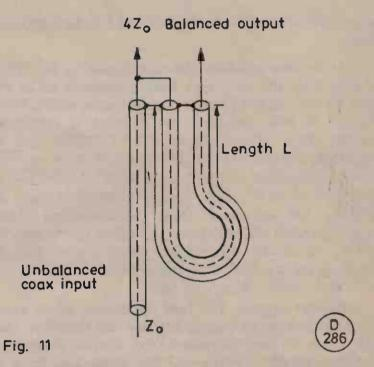
Fig. 11. Coaxial balun giving an impedance transformation of 4:1; length 'L' is a half-wave on the frequency for which the balun is designed, and must take into account the Velocity Factor of the coaxial cable used.
