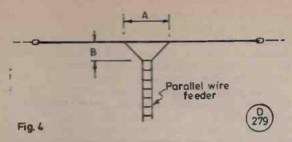
Fig. 4. The Delta Match; lengths 'A' and 'B' are discussed in the text.
