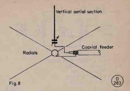
Fig. 8. Matching a ground-plane's feed impedance to the feeder by making the antenna's length greater than a quarter-wave; the reactance is removed by inserting the series capacitor. For details of lengths, see text.
