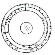
Outer Diameter = 70 mm. Inner Circle = 50 mm. Central Hole = 17 mm. Figure 1
