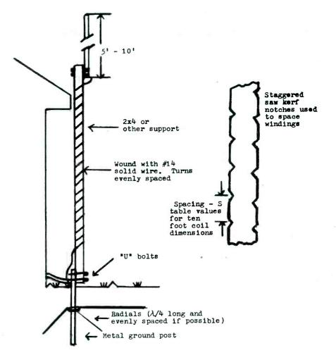
Here on the desert I use a ground plane made of wires buried under the surface of the ground and connected to a metal stake at the base of the antenna. The ground plane wires should extend radially outward in a symetric pattern. In my location, they extend only in a generally north-south direction but the reinforcing in the slab foundation may contribute some ground conductivity in one direction.
