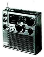
The tuning system is very unique. It will be a little hard to explain, but it goes. There are two controls: main and bandspread. but do not think of the DX-160, it is far from it. The main dial is marked every 250 kHz, but for accuracy, a crystal marker which puts out harmonics every 250 kHz is built in. After tuning to a 250 kHz interval on the main dial, the bandspread becomes accurate to 5 kHz. The bandspread tunes + or - 150 kHz from the 250 kHz main dial setting.
