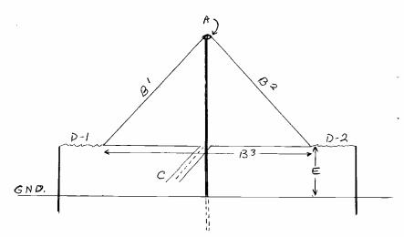
A- Insulator, with B-1 and B-2 separated electrically B-1, B-2, B-3- INSULATED wire of sufficient diameter for local condx C- Coax to receiver D-1, D-2- non-conductive support ropes E- a distance of 10 feet or more Note: All 3 sides should be equidistant. Coax should droop down to CND level, then be run atop the ground or buried, to rx. (Neal A. Perdue, AL) MERRY CHRISTMAS MERRY CHRISTMAS MERRY CHRISTMAS MERRY CHRISTMAS
