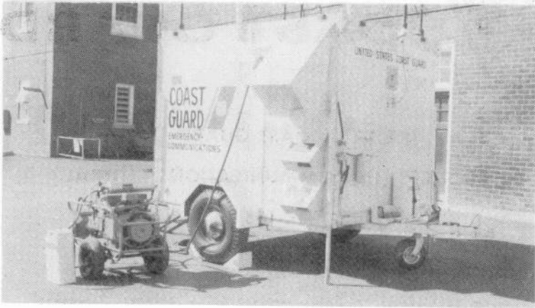
Communications Central AN/TRC-168 with 10kW portable gasoline generator
