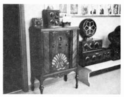
The Freed-Eismann Neutrodyne was made in 1923 and featured 5 tubes and 3 tuned circuits. It sold for \$150. Almost hidden by its white name tag is the Crosley Pup, the portable predecessor to the popular transistor. It used one tube, headphones and sold for \$10.
