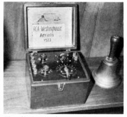
The oldest radio in the collection is the RCA-Westinghouse Aeriola built in 1922. As are many of the sets, it was battery operated and the listener heard the programs through earphones or the old-fashioned horn type loudspeaker.
