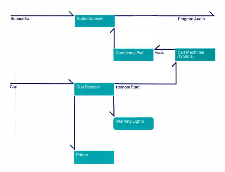
Cue Decoder provides discrete relay closure 30V/0.1A.
