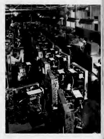
RCA Color TV receivers are shown undergoing final color tests on the assembly line of RCA's Home Instrument Division plant at Bloomington.
