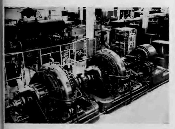
The 200-kilowatt Alexanderson alternator revolutionized radio during first World War. Today, short-wave transmitters have replaced long-wave alternators.
