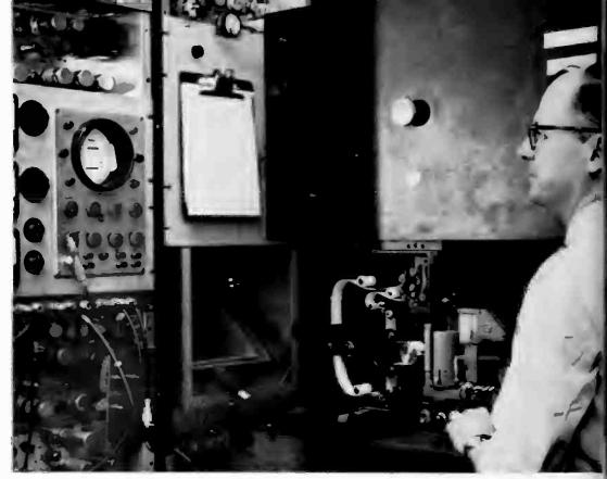
Bob Fraser, NBC development engineer, is shown above making preliminary adjustments on an experimental high-definition kinescope recording camera and recording chain.
