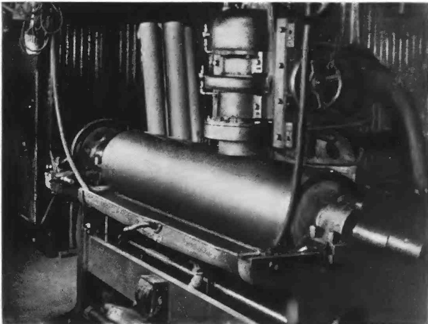
AFTER the COLO<sup>R</sup>oto Magazine is printed, the copper cylinders are re-surfaced so that another set of pages may be etched. The cylinder was made by depositing copper on a steel core in an electrolytic bath.
