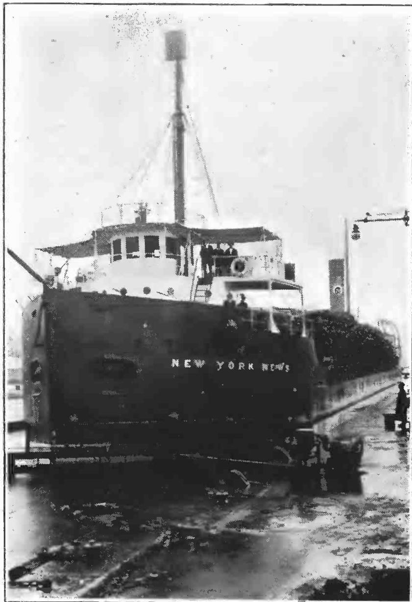
THESE steel steamers were built by The Tribune to carry pulp logs from our timber lands to our paper mill. Special design gives them larger capacity than any other boats navigating the St. Lawrence and Welland canals.
