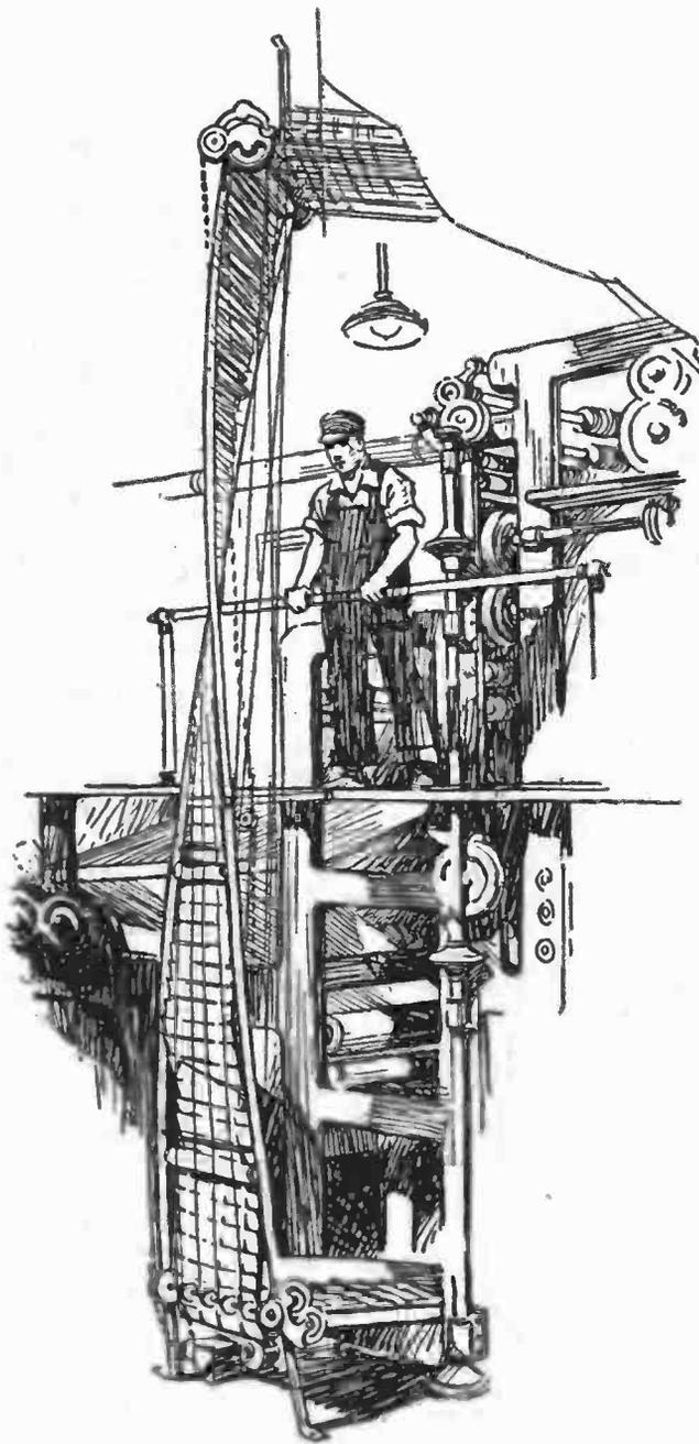
Each conveyor consists of spiral-wound, wire spring cables facing each other and running over pulleys. The pressure of these cables against each other holds the papers firmly between them and carries them swiftly upward.
