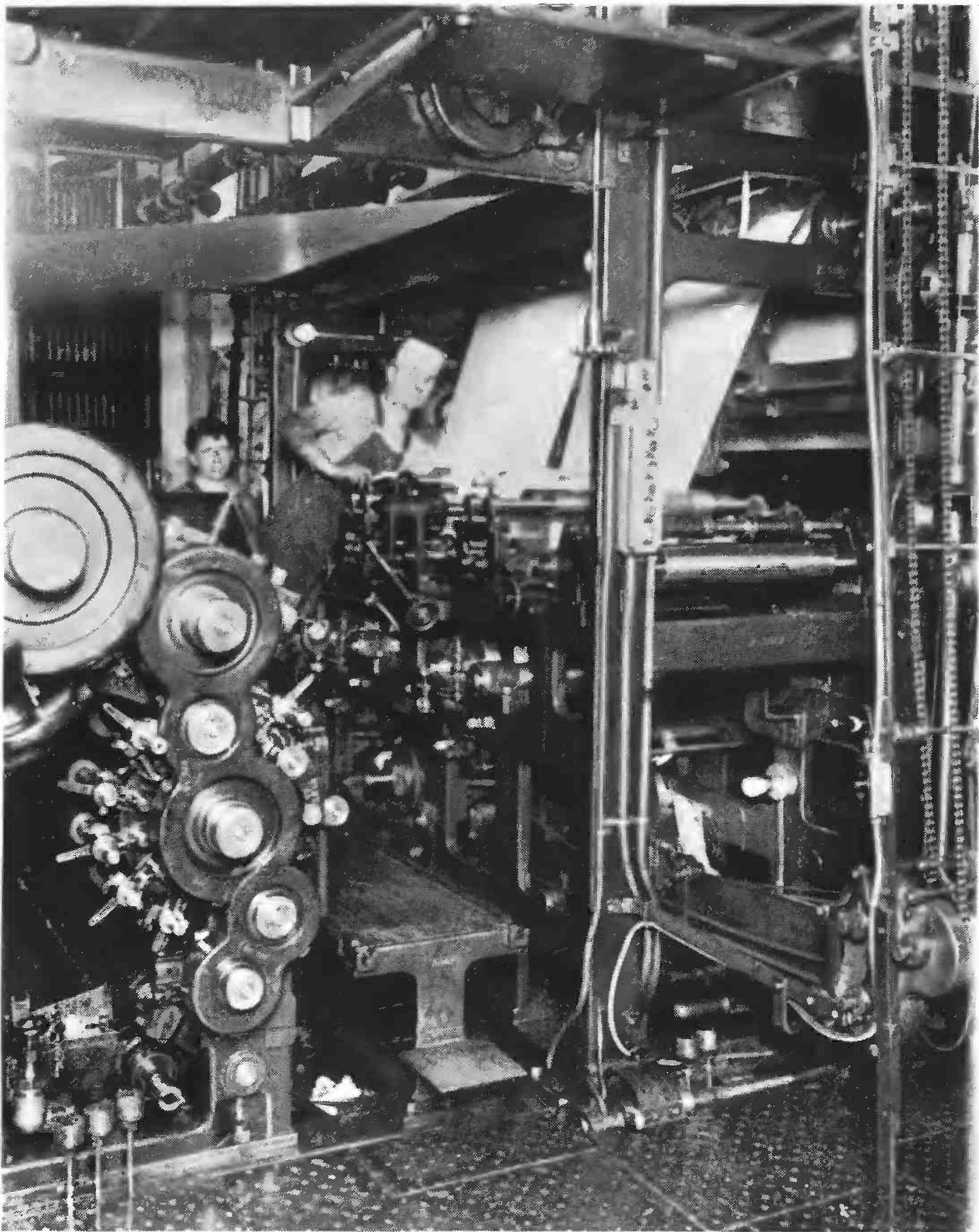
*IN THE center is shown that part of the press which cuts and folds Tribunes—printing unit at left—conveyor at right.*
