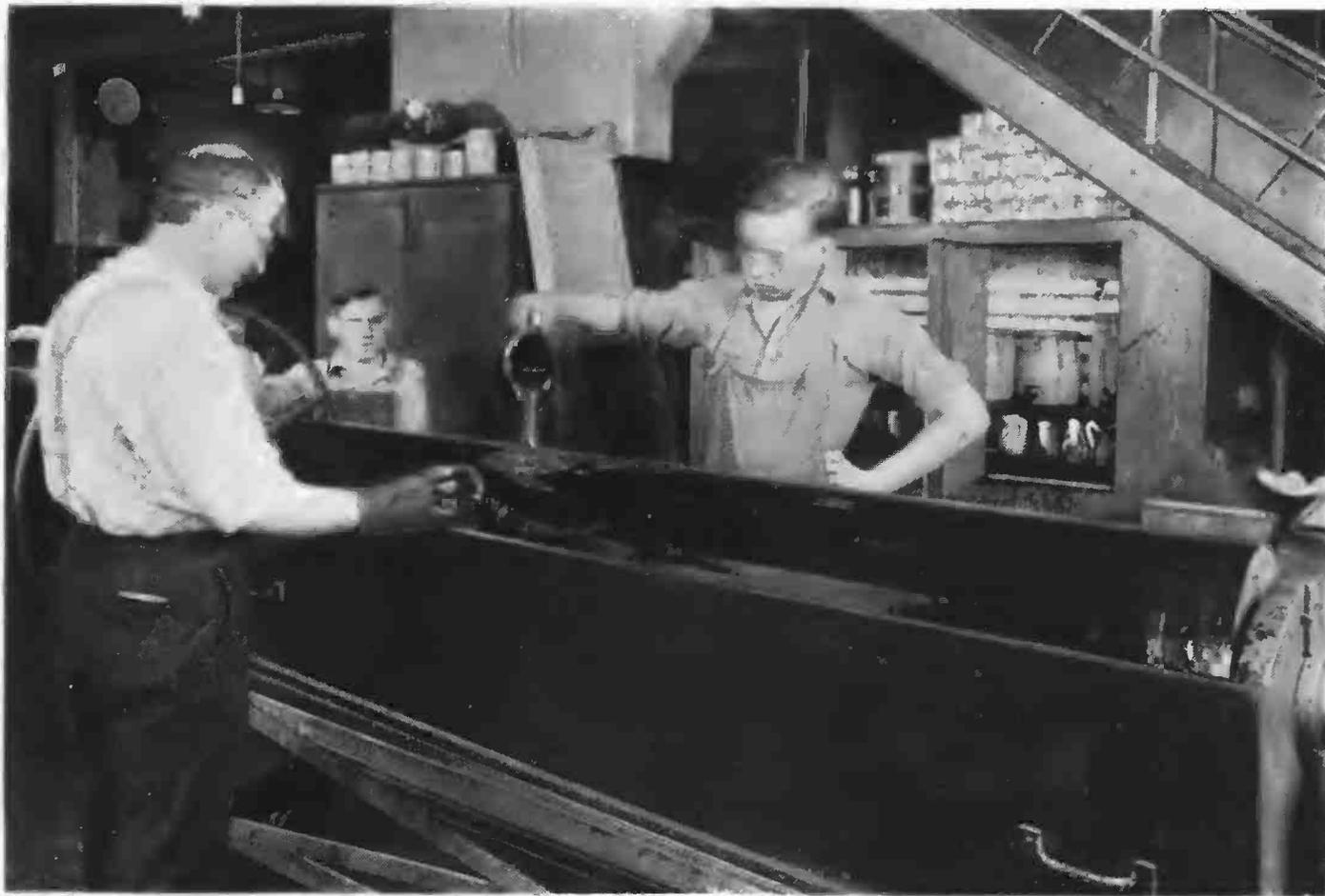
ETCHING one of the copper cylinders which print COLO<sup>R</sup>oto.
