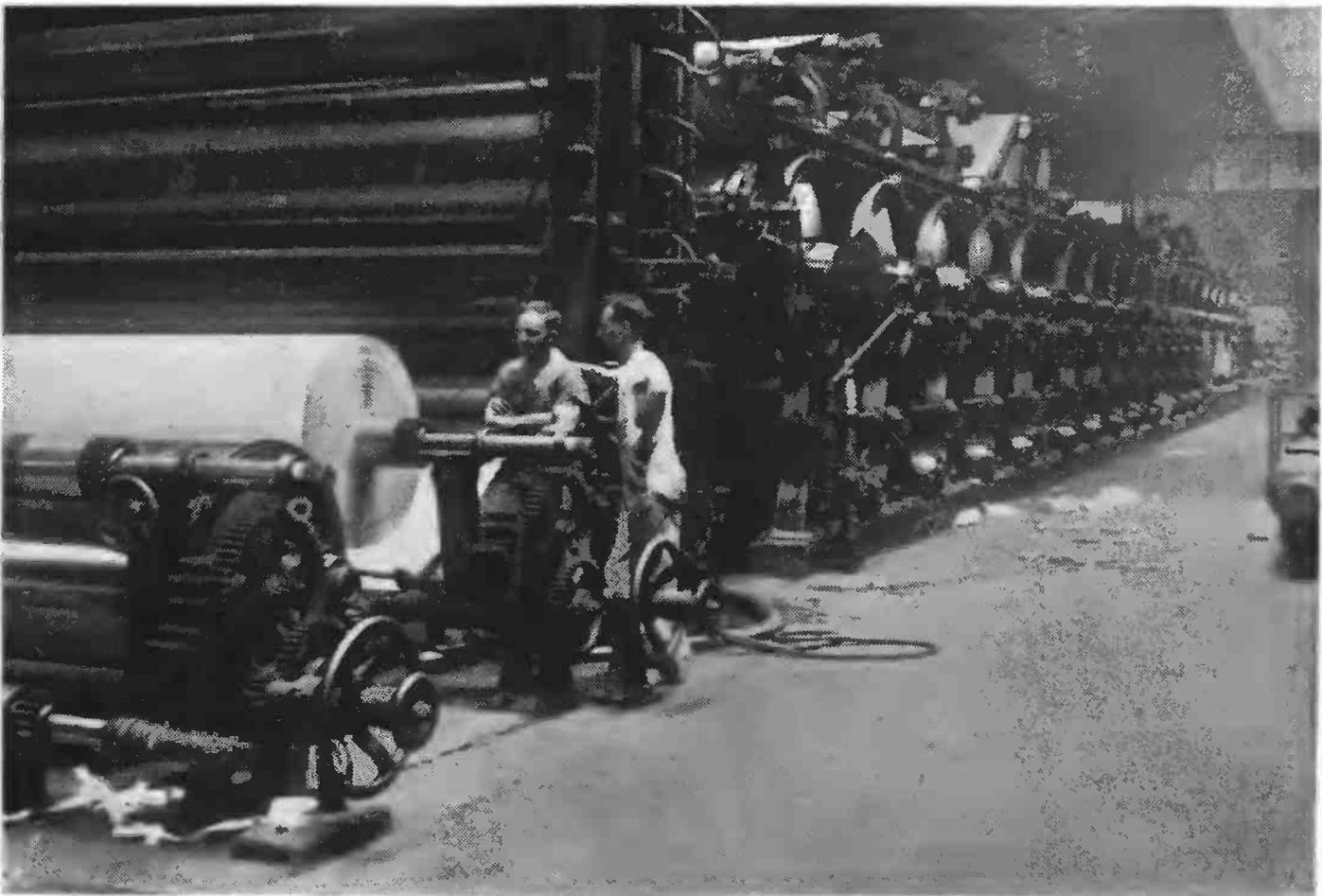
THIS picture shows, from right to left, the long row of dryers, the calendering stack, the winder, and the re-winder of one of *The Tribune's* paper machines.
