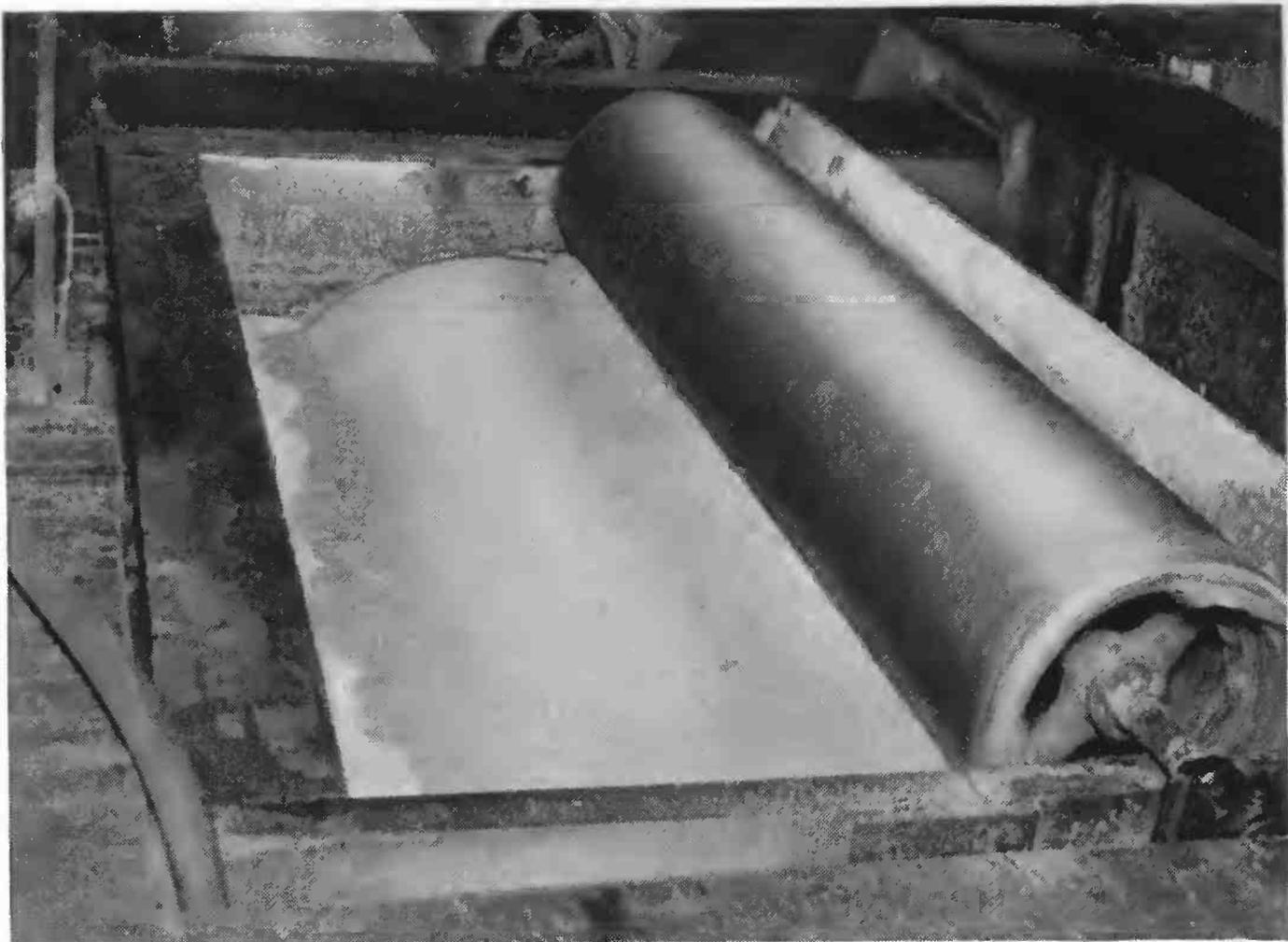
*AFTER splinters have been screened from the wood pulp it is forced between these two rolls. Water carrying away all soluble impurities flows through the lower, which is made of fine copper screen.*
