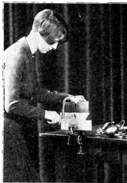
Cutting heavy sheet metal for shields, etc., is one of the most difficult jobs for the radio set builder. This work cannot be done successfully with shears, but the illustration shows how the job may be easily performed with a saw such as the F. P. M. holding the sheet metal between two boards. The cutting pattern is marked on the board facing the operator—or operator.
