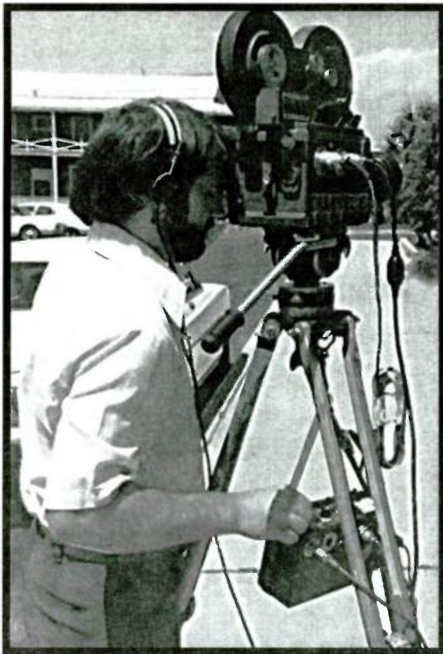
WECT TV 6 Cameraman covers a news event in the late sixties with a sound news camera. The processed black and white footage was then edited on the equipment shown below and then delivered to the control room ( bottom picture) for insertion in the daily newscast.
