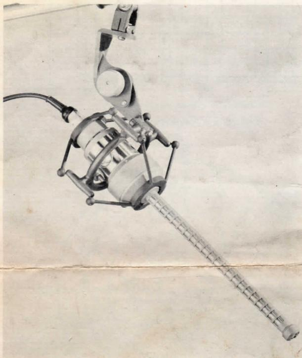
The Cardiline\* Model 642 is a highly directional dynamic microphone utilizing a combination of the characteristics of cardioid and distributed front opening designs. The cardioid action gives the microphone essentially unidirectional characteristics at frequencies up to 500 cps. At this point the distributed front opening takes over for the balance of the range to which it responds providing directional characteristics illustrated in the polar diagram, Figure 3.
