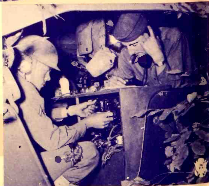
Reporting by radio from concealed command car. Note transmitter key on radio operator's thigh.
