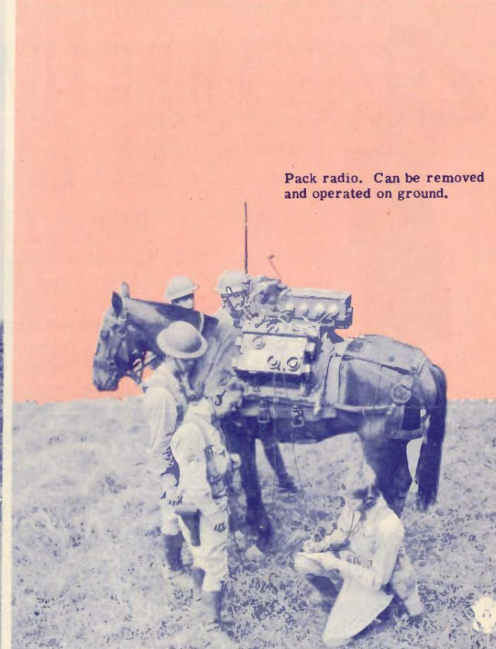
Pack radio. Can be removed and operated on ground.
