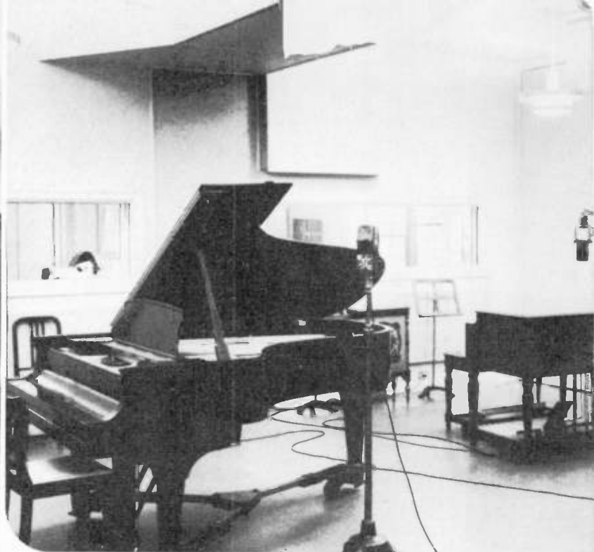
STUDIO C. Hinged panels on wall are for adjusting the studio's acoustics to fit each program.
