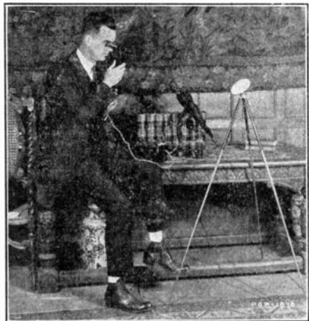
How the Macbeth illuminometer is used to determine the illumination at any desired place. The illumination received by the little disc tells what is being received by that particular part of the room, and every corner and nook can be tested.
