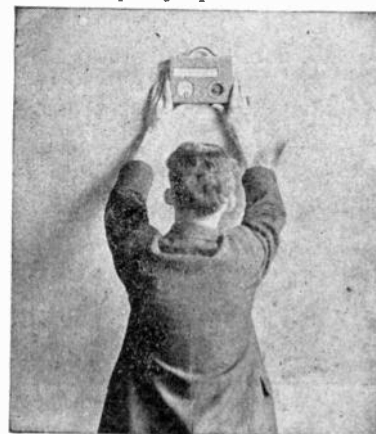
Using the foot-candle meter to determine the illumination received by a screen or wall. This suggests its use for determining the illumination of the moving picture screen.
