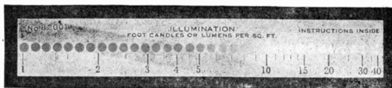
View of the scale of the foot-candle meter, indicating in this case an illumination of 10 foot-candles, quite a high illumination, as light is now distributed.
