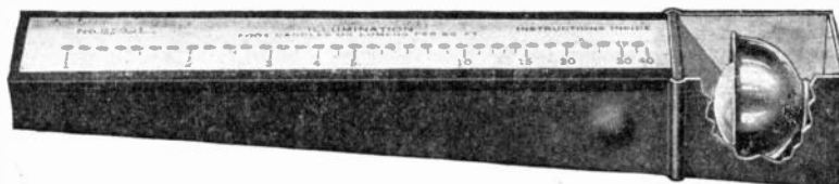
The foot-candle meter's essential part, the case holding the standard lamp, with the series of translucent apertures, whose brightness tells by simple inspection the illumination received at any place where the instrument is placed.
