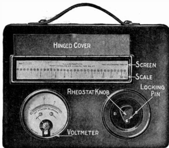
On left the candle-power meter in its compact traveling case, ready for transportation to the scene of its operation. The light-box cover is raised to show the screen.
