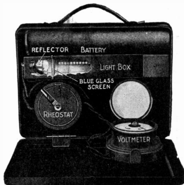
On left the candle-power meter in its compact traveling case, ready for transportation to the scene of its operation. The light-box cover is raised to show the screen.
