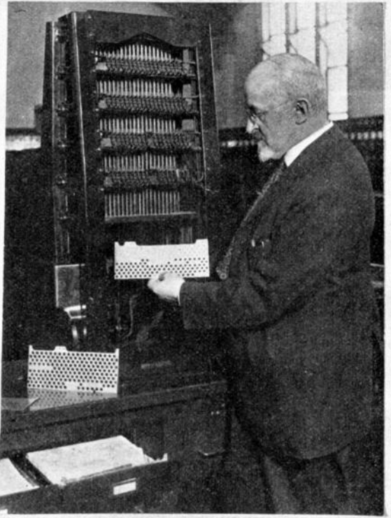
The illustrations show the elaborate switchboard, plugging-in boards, the perforated card apparatus, and sending instrument used for the complicated fire-alarm system of New York. The illustrations give some idea of the complexity involved in taking care of the numerous alarm stations scattered over the great city.
