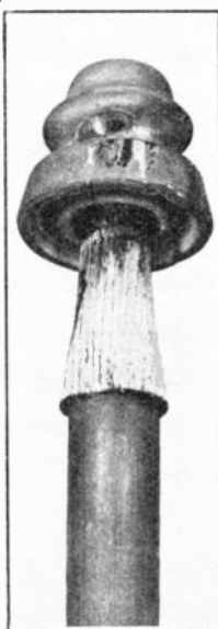
Two views of an insulator pin on a high tension transmission line pole, where a fire was caused by a surface current leak.
