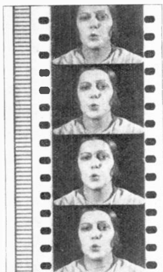
Four views of a face on a moving picture film, with the record of the voice enunciating the sound of "O" photographed on the left edge.
