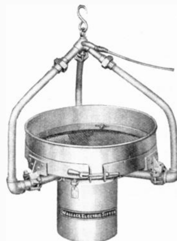
A most ingenious electric sifter agitated by a motor purposely thrown out of dynamic balance.
