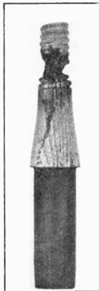
Two views of an insulator pin on a high tension transmission line pole, where a fire was caused by a surface current leak.
