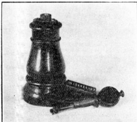
An electric cigar lighter; the upright portion holds gasoline and a sparking rack is seen at its base; the lighter proper is lying alongside of it; it operates by connection to the lighting circuit.
