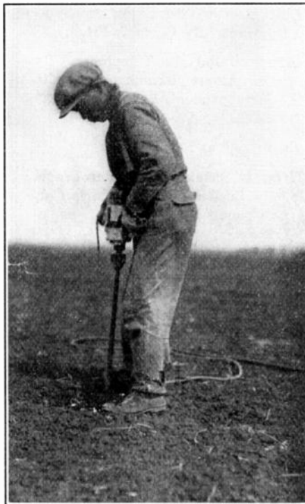
Using electricity to bore holes in the ground for the planting of grape vines—a California achievement which economized time and money.
