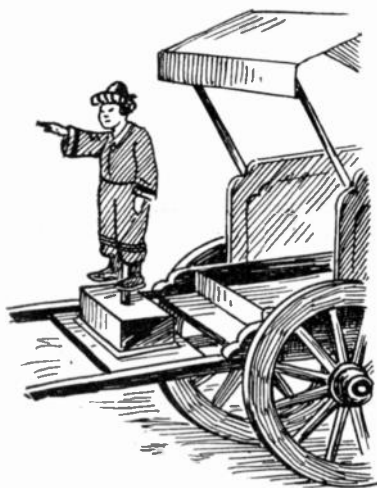
Chinese figure supposed to be turned by the action of a magnet or loadstone within it, so as to point always to the south. It is to be assumed that the jolting of the cart assisted its movements.
