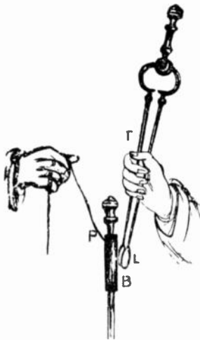
Old-fashioned way of magnetizing a piece of steel held against a poker, by stroking with tongs. Reproduced from an old book.
