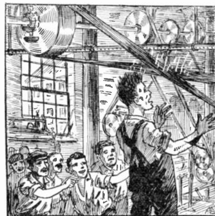
Static electricity in a factory, produced by the travelling belts, making a workman's hair stand on end, to the surprise of his companions.
