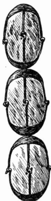
Armored loadstones with top and bottom pole pieces of soft iron fastened on by the wires as shown.
