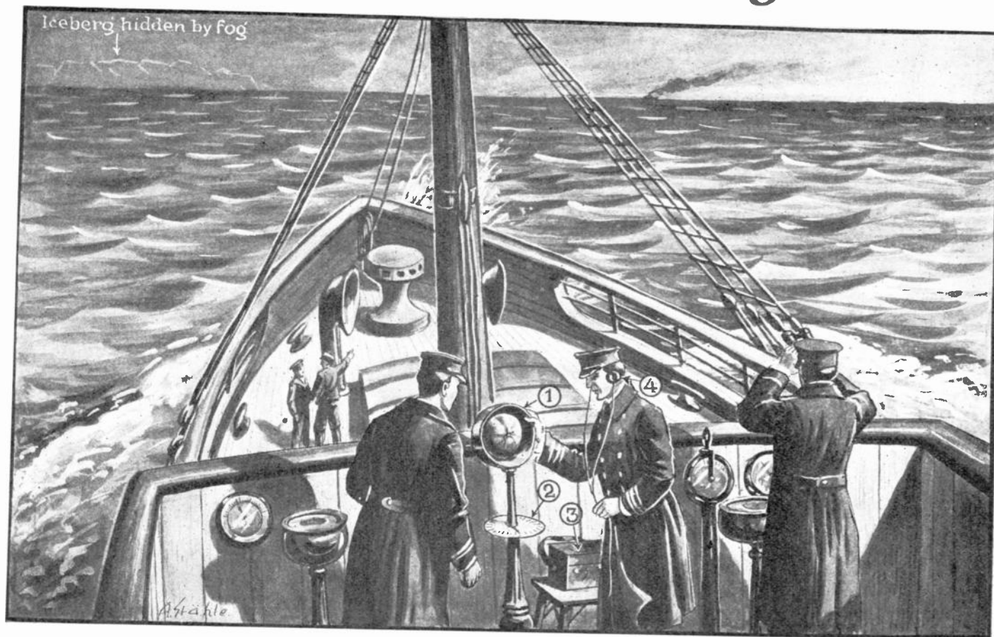
Detecting an iceberg in the distance by the action of infra-red rays; they are received by a reflector (1) and made to affect telephones (4). A dial (2) gives the direction of the iceberg; in the box (3) is contained the apparatus, and the headset tells of the impending danger.
