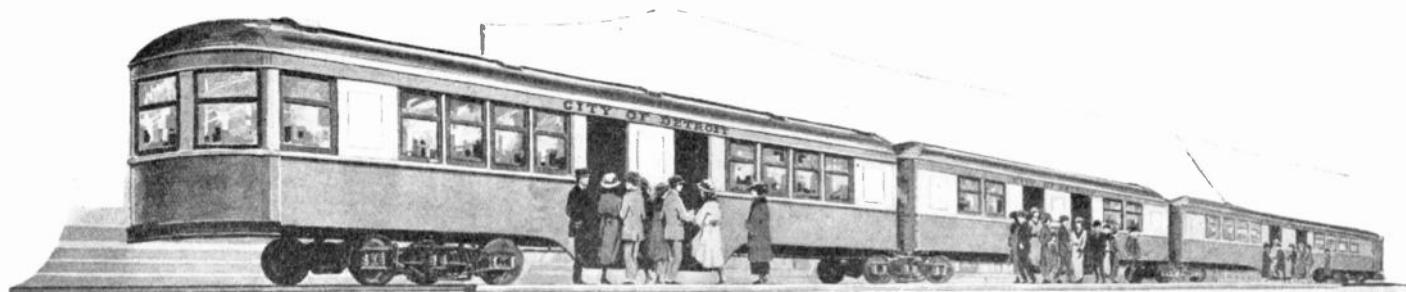
Articulated trolley train. The interesting feature is that the intermediate trucks serve each one for the ends of two cars; thus in the three-car train there are only four trucks, where normally there would be six. It has been used in England and is now to be tried out in this country.
