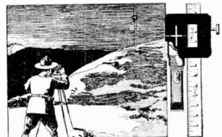
This target is for use on a leveler's rod. An electric flashlight is mounted on the rod, giving a luminous target upon which the leveler trains his instrument for reading the levels in the usual manner. Thus the device may be used in dark places.
