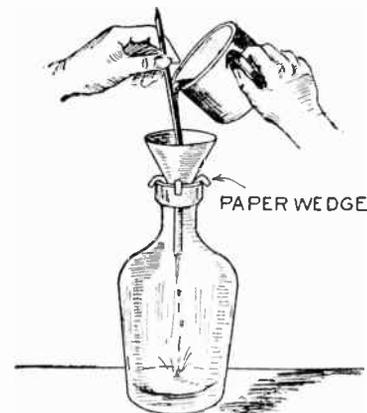
**POURING THE SOLUTION THROUGH THE FILTER**
