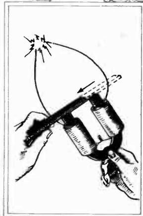
Faraday's primitive "magneto" coil! A change in the magnetic field caused by the sudden motion of the permanent magnet induces an electromotive force in the coil and available at the terminals right.
